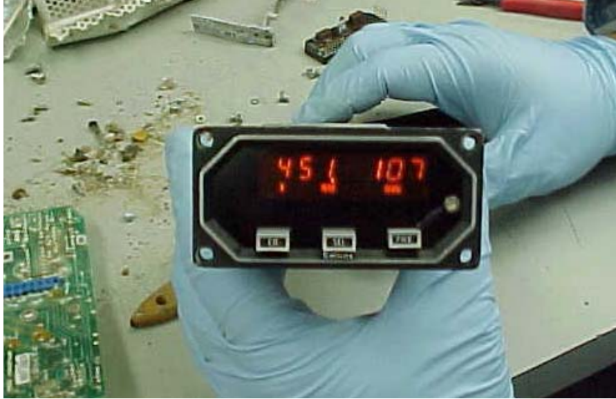
Figure 2 - Accident Display Installed in Slave Unit
