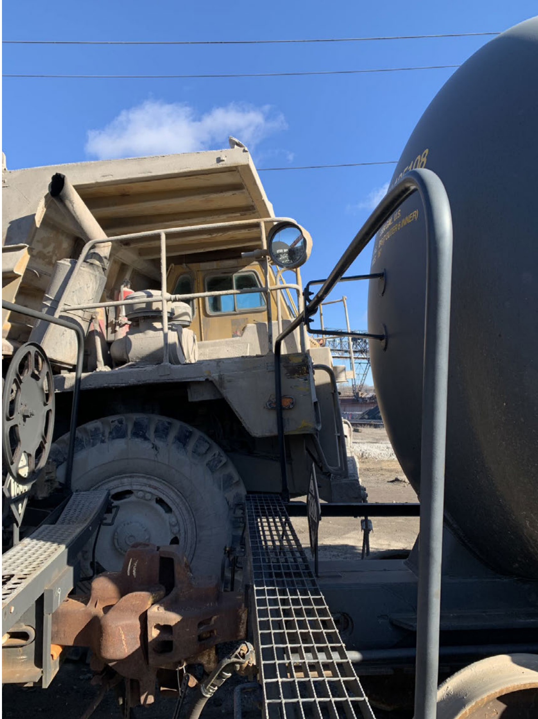
Figure 1. This photo was taken by the system safety group chairman during the on-scene portion of the investigation. It shows the final resting place of the truck and train. The front right of the truck contacts the side of a railcar.
