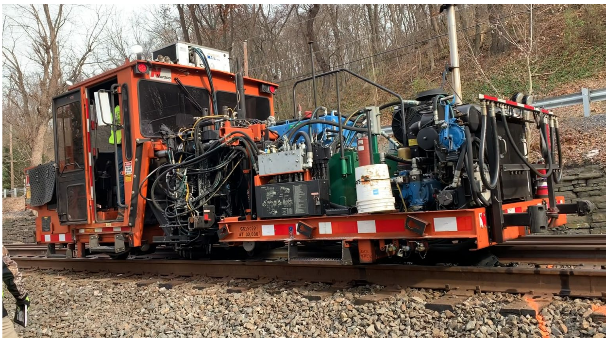
Spiker 2 Exterior - NTSB photograph shows the roadway maintenance machine (Spiker 2) involved in the accident on Norfolk Southern's main track Buffalo line in Reed, PA.
