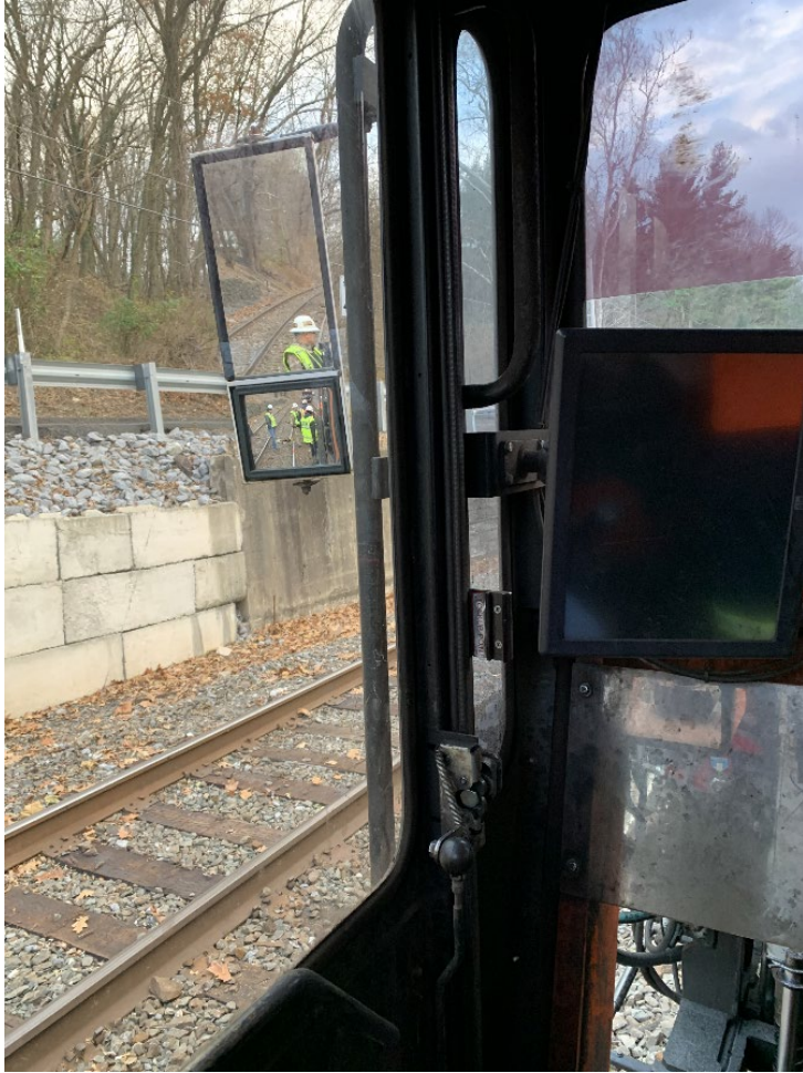
Spiker 2 Mirror - NTSB photograph that shows the left rear-view mirror of Spiker 2 from the perspective of the left operator seat.
