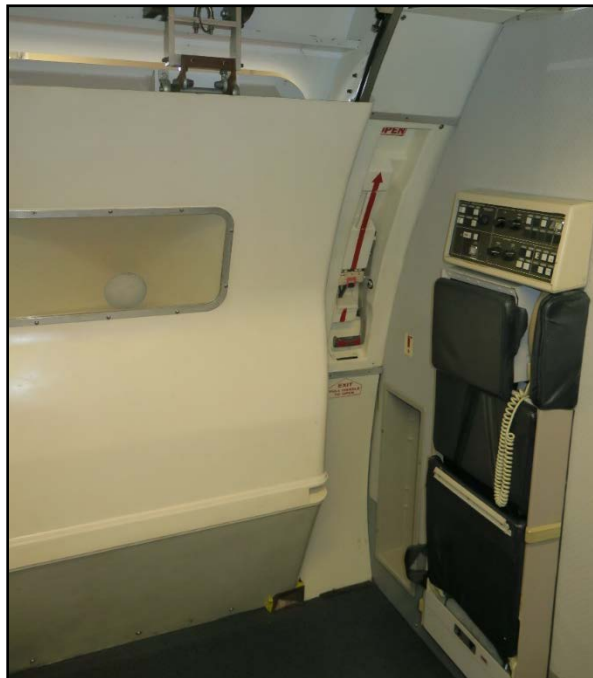
Photograph 3 – Boeing 767 door trainer Type A exit.
