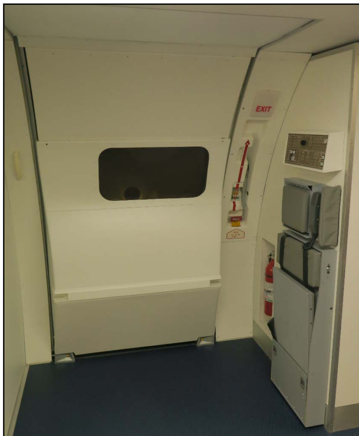
Photograph 1 – Boeing 767 door trainer Type A exit.
