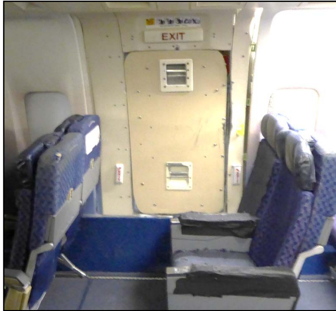
Photograph 4 – Boeing 767 door trainer Type III exit.
