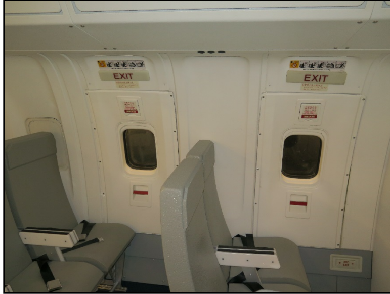
Photograph 2 – Boeing 767 door trainer Type III exits.
