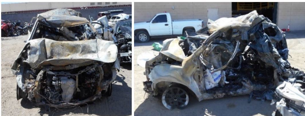
Figure 4. Frontal view of Equinox deformation. Figure 5. Left side view of Equinox deformation.
