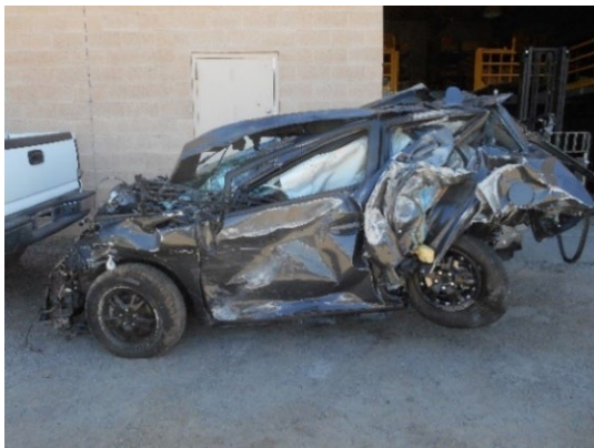
Figure 14. Left side view of deformation to Prius.
