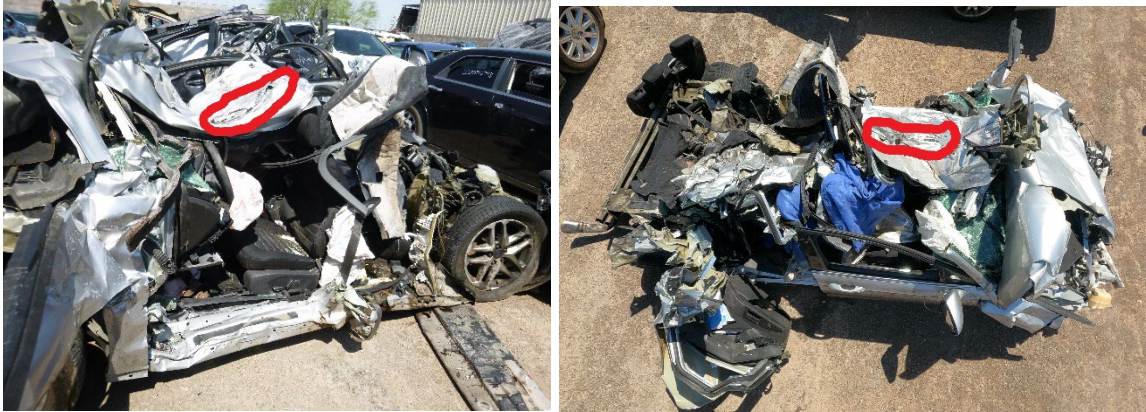
Figure 12. Exterior view showing rubber transfer to roof. Figure 13. Overhead view of Ford Fusion.
