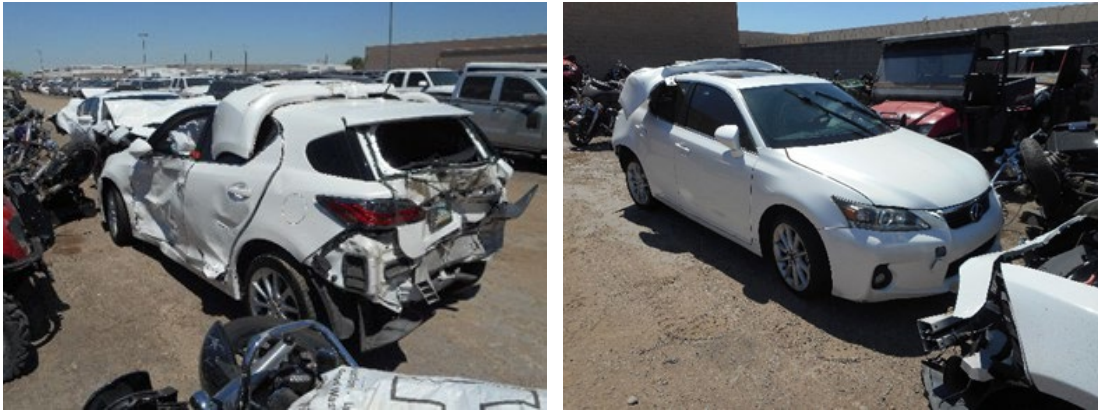
Figure 21. Rear left angle view of deformation. Figure 22. Front right-angle view of undamaged front end.
