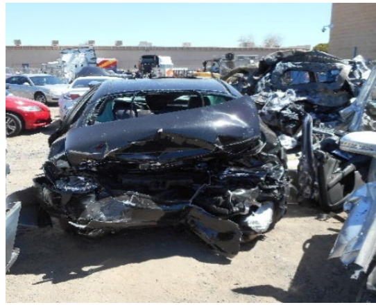
Figure 17. Frontal view of deformation to Mercedes. Figure 18. Rear view of deformation to Mercedes.
