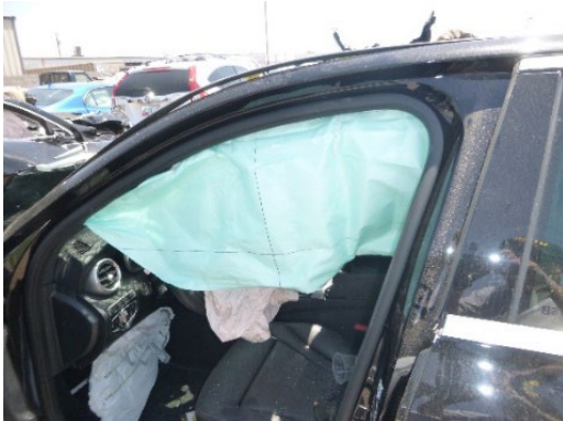
Figure 19. View of deployed airbags from outside driver's door. Figure 20. View of extended and locked seatbelt.
