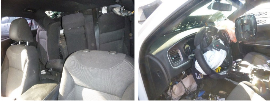
Figure 26. Interior view showing intrusion into back seat. Figure 27. Frontal view of deployed airbags.
