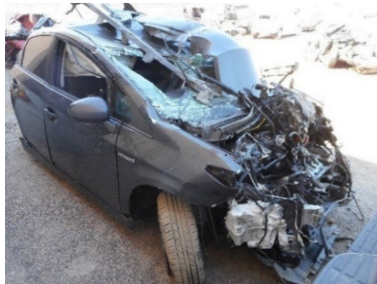
Figure 15. Front right-angle view of Prius deformation.
