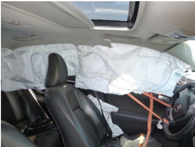
Figure 23. Interior view of side curtain and driver torso airbags deployed.
