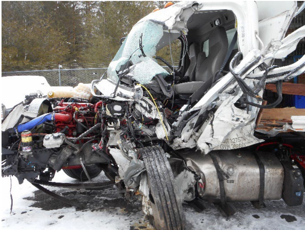
Figure 2. Left side view of damage to 2021 Freightliner box truck.
