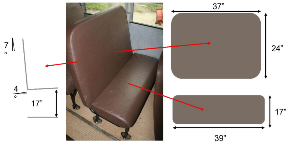
Figure 11. Dimensions of the "Add-on" passenger seats in the last two rows on the right
