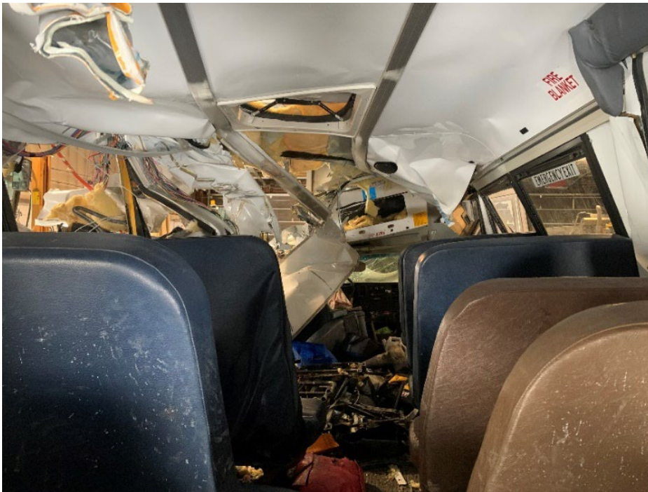
Figure 9. Interior view looking rear to front at intrusion to interior of 2013 Chevrolet Express.
