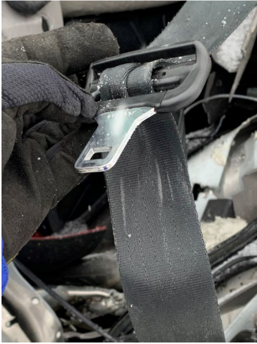
Figure 5. View of loading evidence on latchplate and webbing.
