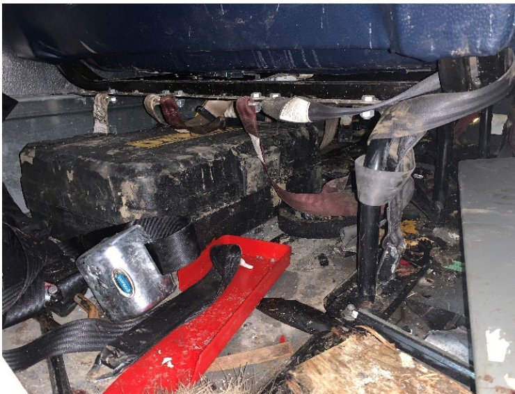
Figure 14. View of lap belts hanging underneath seats and wrapped around seat legs.
