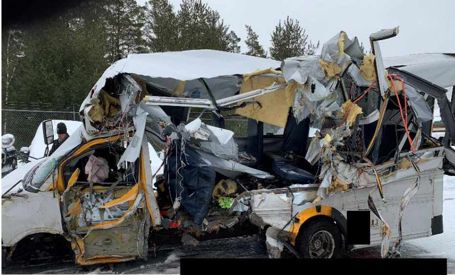
Figure 8. Left-side view of damage showing integrity loss to passenger seating compartment.
