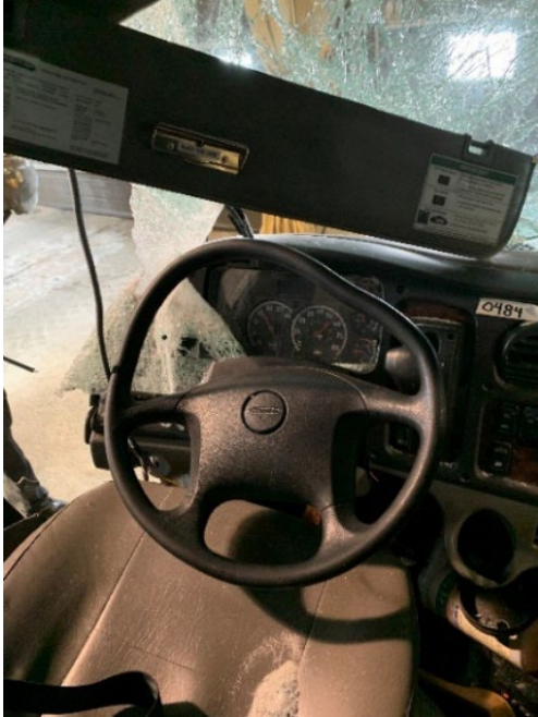
Figure 3. Interior view of deformed steering wheel.
