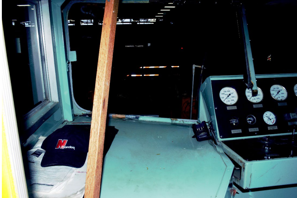
Photo 5 Close-up photograph of the location where the CTA employee was ejected through the windshield. The photograph shows the damage to the top of the equipment box and the missing glass caused by contact with the employee's body. (Source: NTSB)
