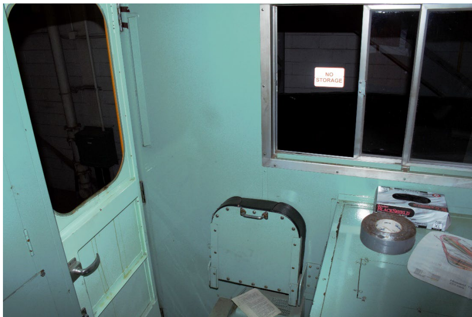
Photo 4 Photograph showing one of the fold-down seats in the cab of the snow removal vehicle and the proximity to the entrance door located at the rear of the cab. (Source: NTSB)
