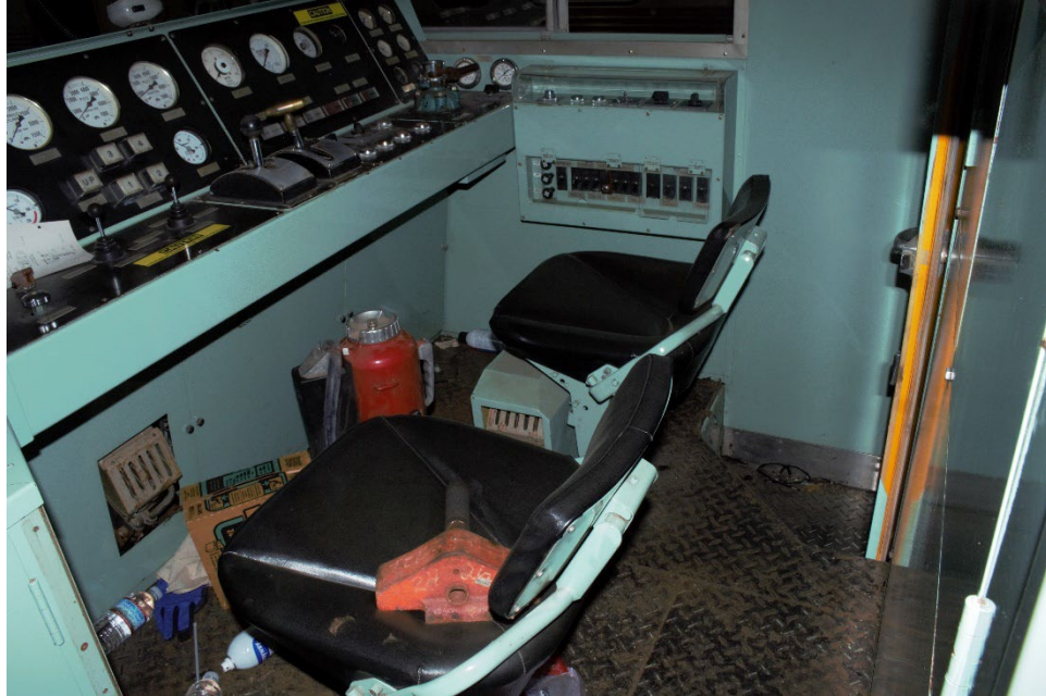
Photo 3 Photograph of the interior of the snow removal vehicle cab showing the proximity of the operator's seat to the control console and the entrance door behind the seat in the background. (Source: NTSB)
