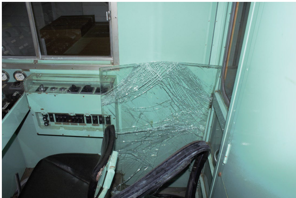
Photo 6 Photograph of the windshield broken out by the ejection of the employee from the vehicle, laying inside of the End No. 2 cab, after it was recovered from the scene. (Source: NTSB)
