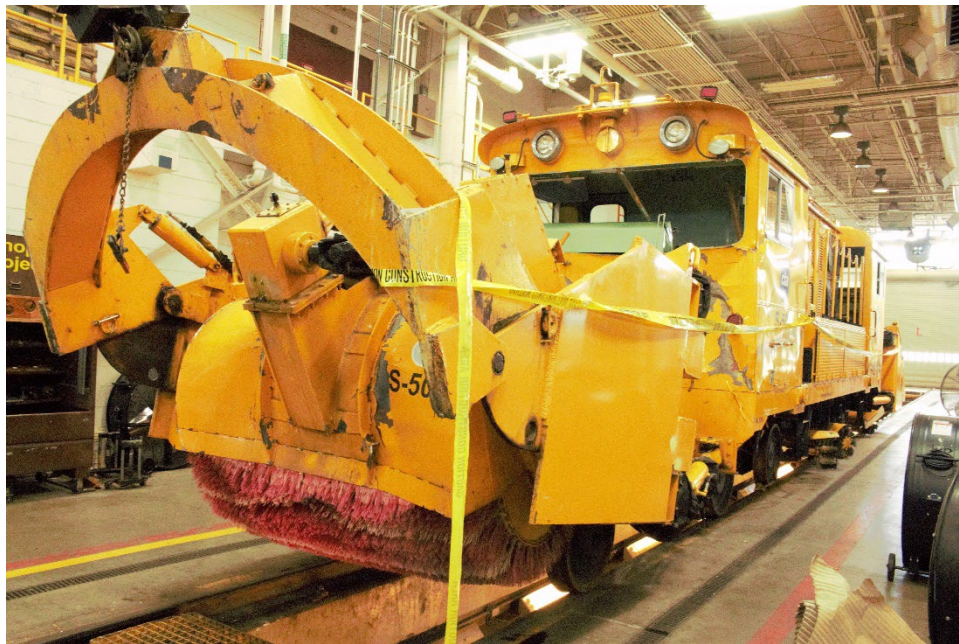
Photo 2 Close-up photograph of the brush attachment located on End No. 2 of the rail borne snow removal vehicle. (Source: NTSB)
