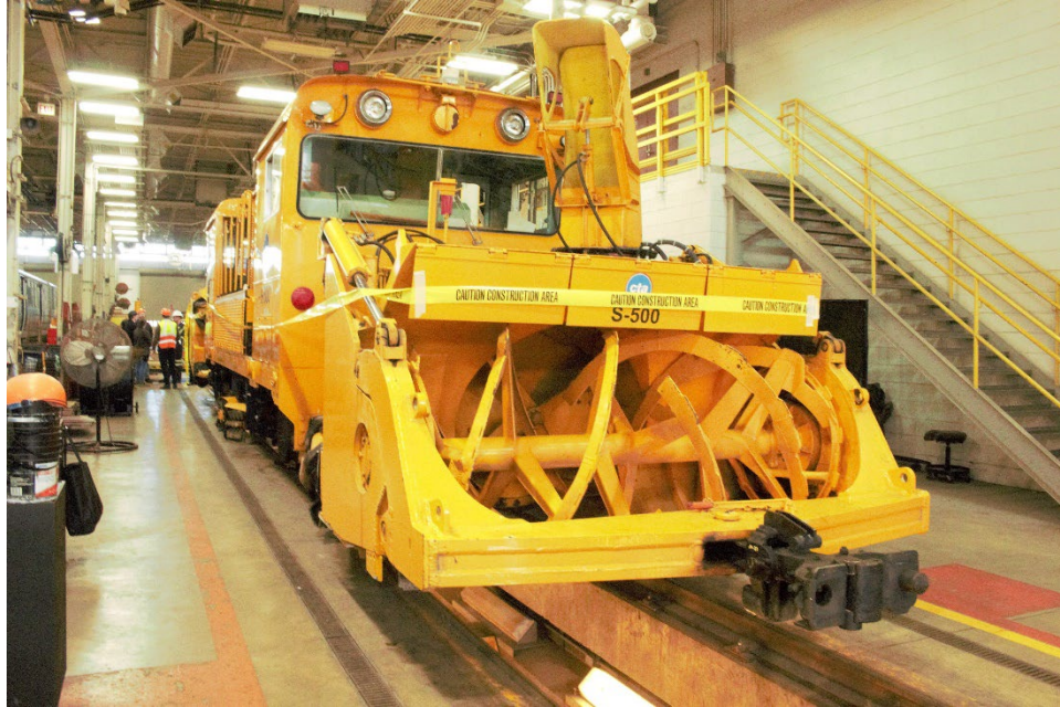
Photo 1 Close-up photograph of the snowplow attachment, located on No. 1 End of the rail borne snow removal vehicle taken at the Skokie yard. (Source: NTSB)
