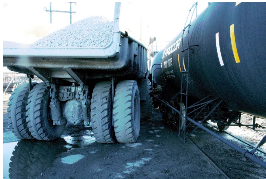
Figure 2 Photograph showing a closeup of the dump truck the final rest position adjacent to the right side of the rail car. (Source: NTSB)
