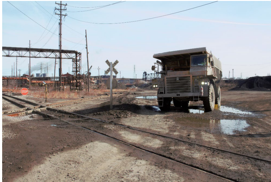
Figure 7 Photograph showing the angle of approach of the dump truck to the crossing. (Source: NTSB)
