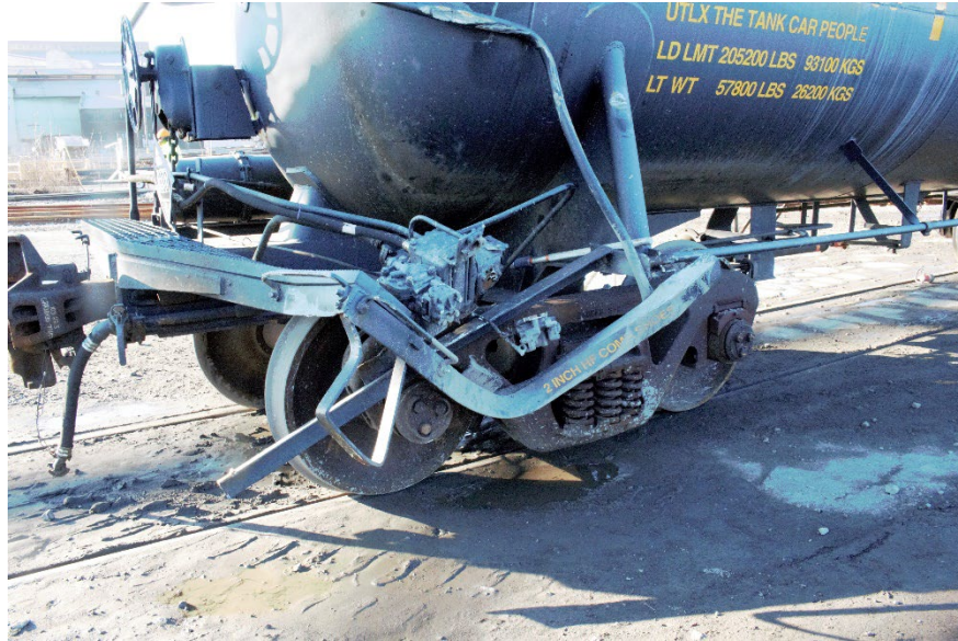
Figure 3 Photograph showing a closeup of the damage to the rear running board where the conductor was standing and the side of the rail car resulting from the impact with the dump truck (Source: NTSB)
