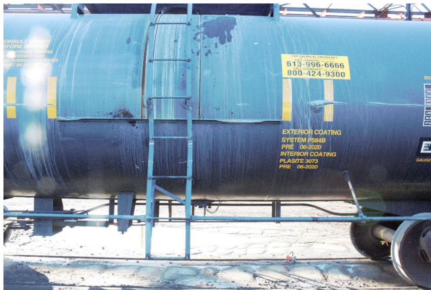
Figure 4 A closeup photograph of the side of the rail car damage by the collision with the dump truck. In the background, the conductor's lantern is seen underneath the rail car. (Source: NTSB)
