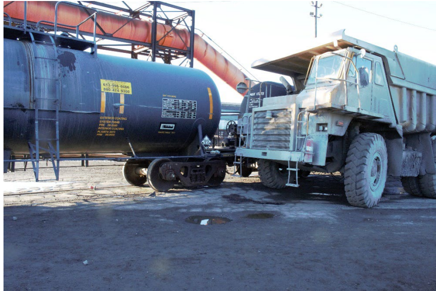
Figure 5 Photograph showing a closeup of the front of the dump truck and its proximity to the rail car at final rest. Damage seen to the side of the rail car occurred during the accident. (Source: NTSB)
