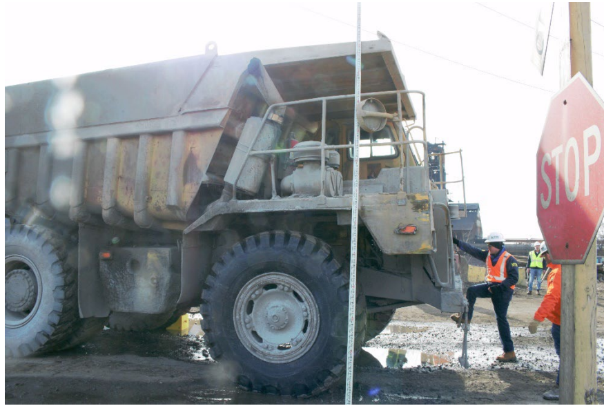
Figure 9 Photograph showing the right side of the dump truck and the obstacles limiting the driver's ability to see the train approaching from the right. (Source: NTSB)
