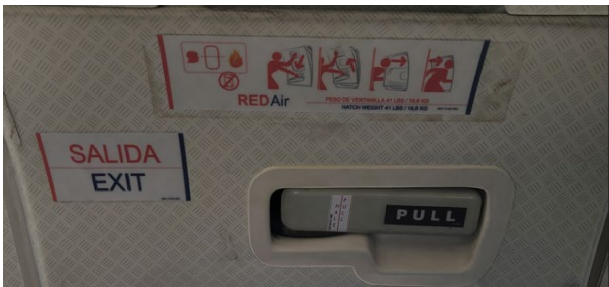
Figure 15- Overwing window exit hatch placard.
