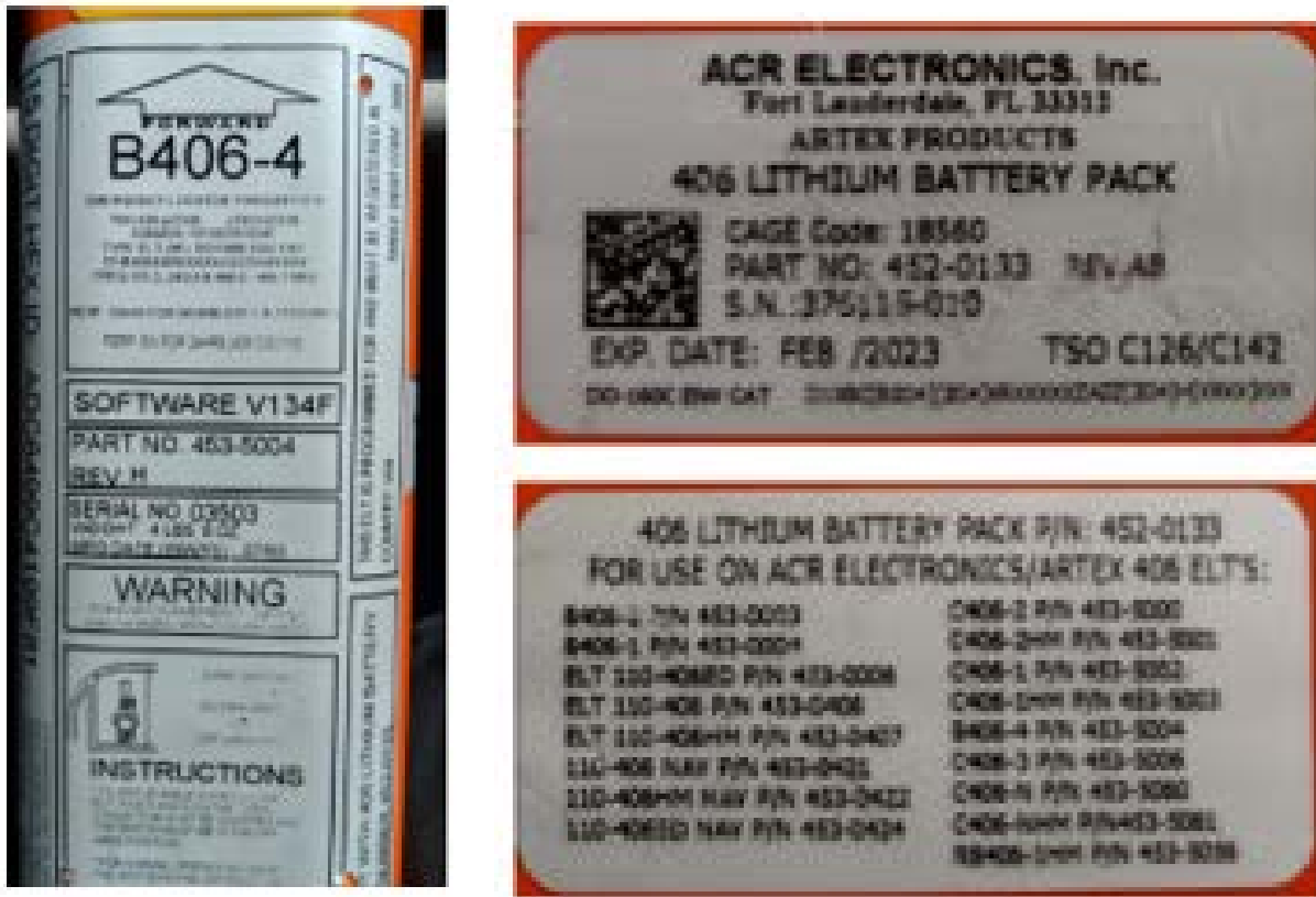
Photograph 20- Labels obtained from the Fixed ELT.
