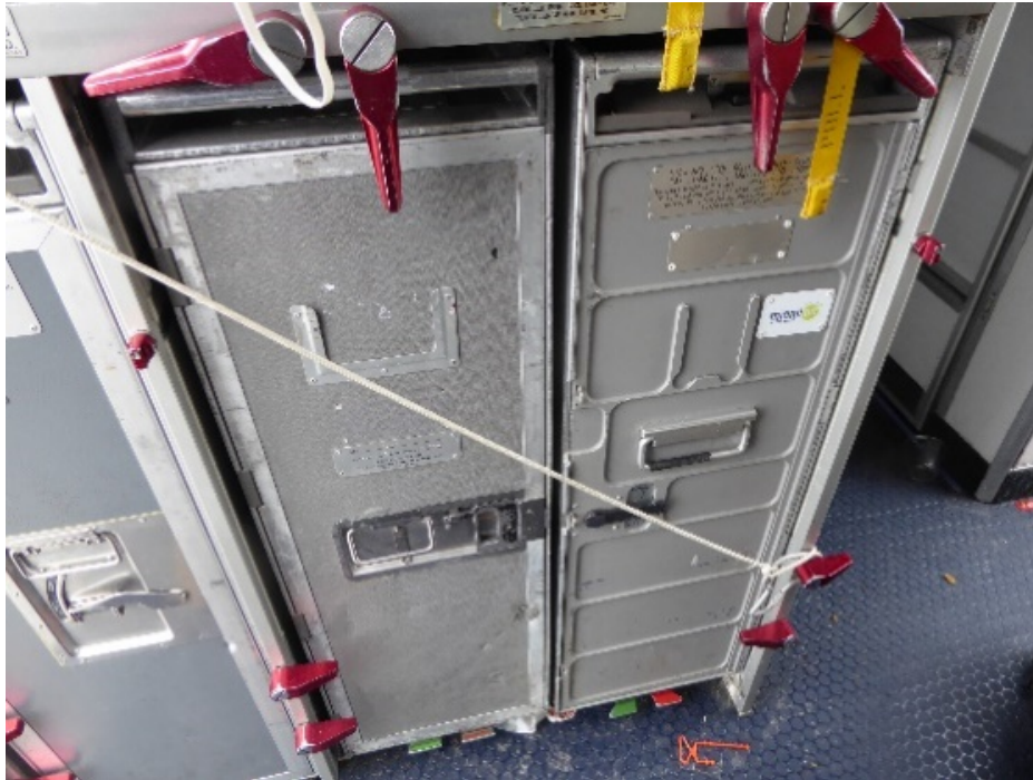
Photograph 16- Raft lanyard connected to the galley cart latch in the G1 galley.
