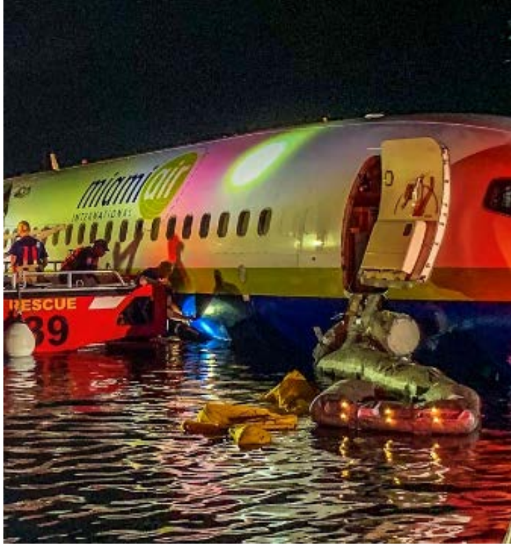
Photograph 7- 1R slide partially inflated and the toe end lighting illuminated.
