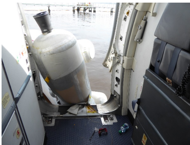
Photograph 5- Internal view of the 1L door and slide.
