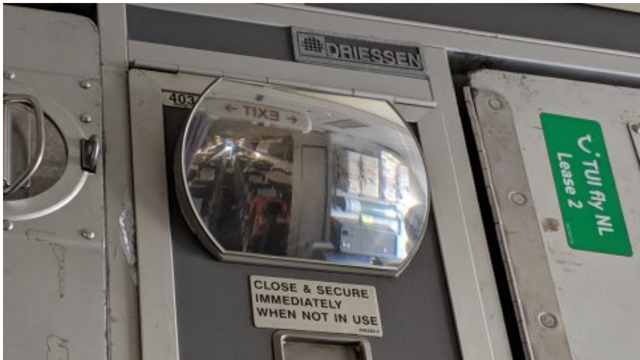
Photograph 19- Mirror that was in aft galley that allowed for a visual of the airplane cabin while sitting in the aft jumpseat.
