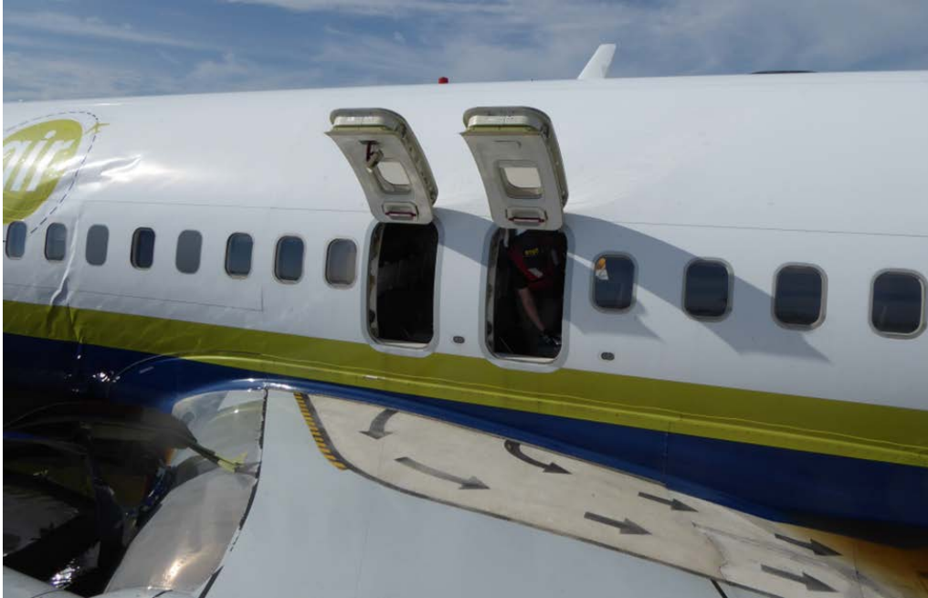
Photograph 13- External view of the overwing window exits – left side.
