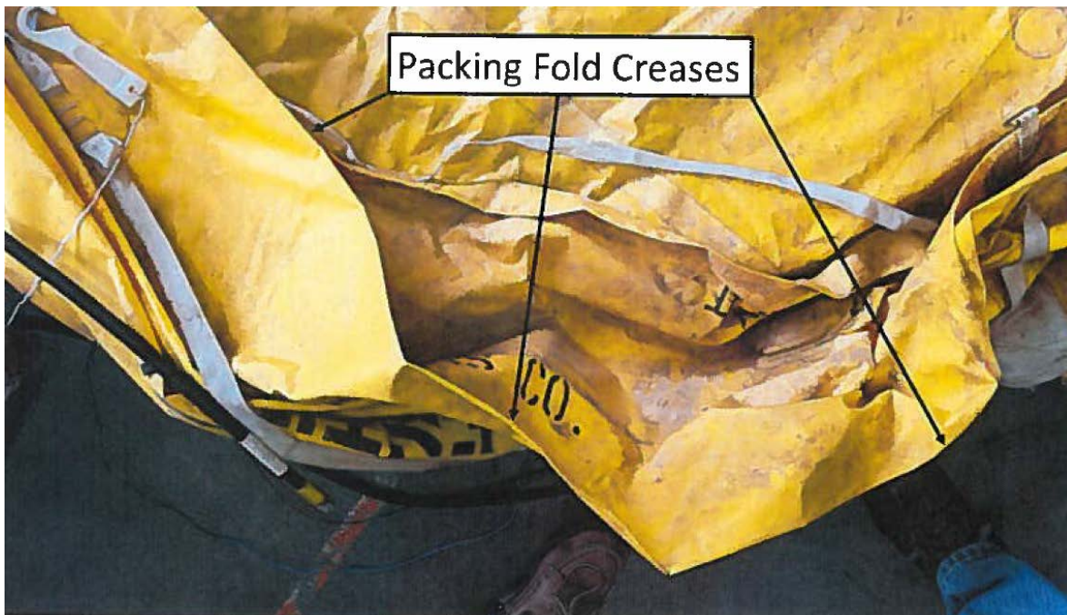
Photograph 26- The fold creases in the raft.
