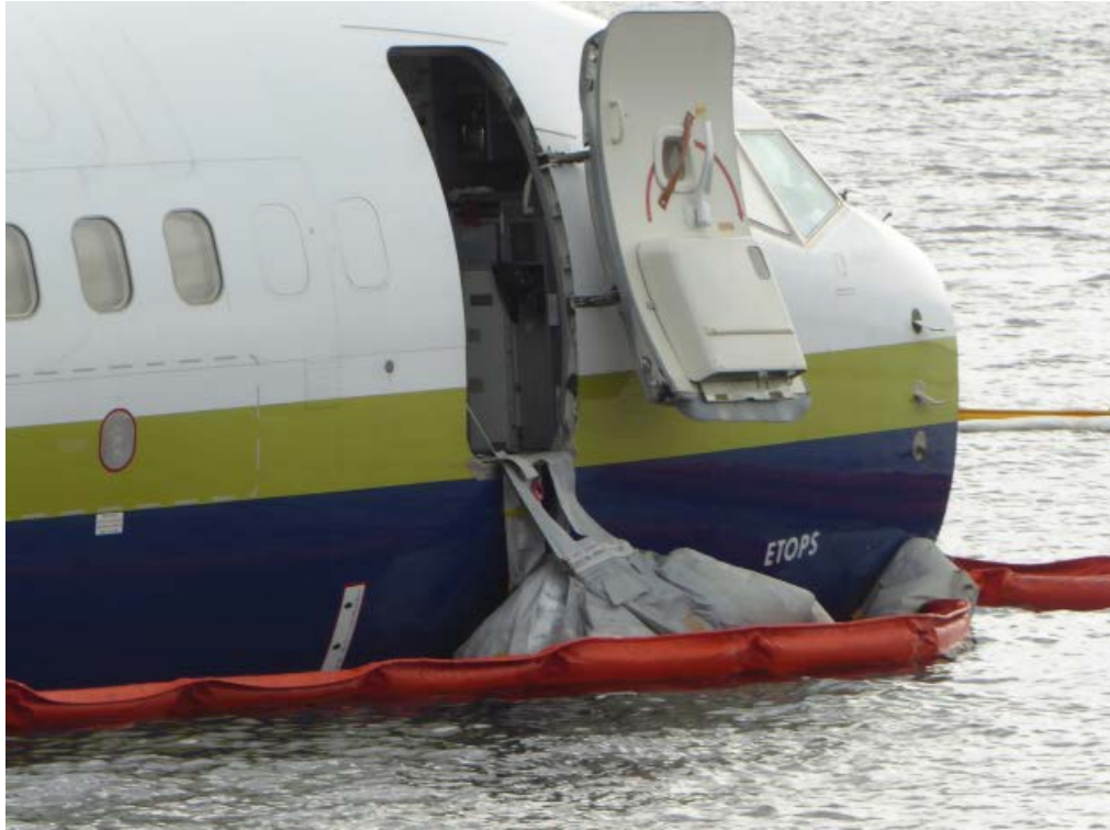
Photograph 8- External views of the 1R door and slide.
