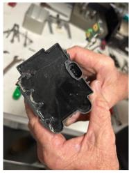
Main board also had damage/corrosion consistent with being under water. No preaccident damage wase noted.
