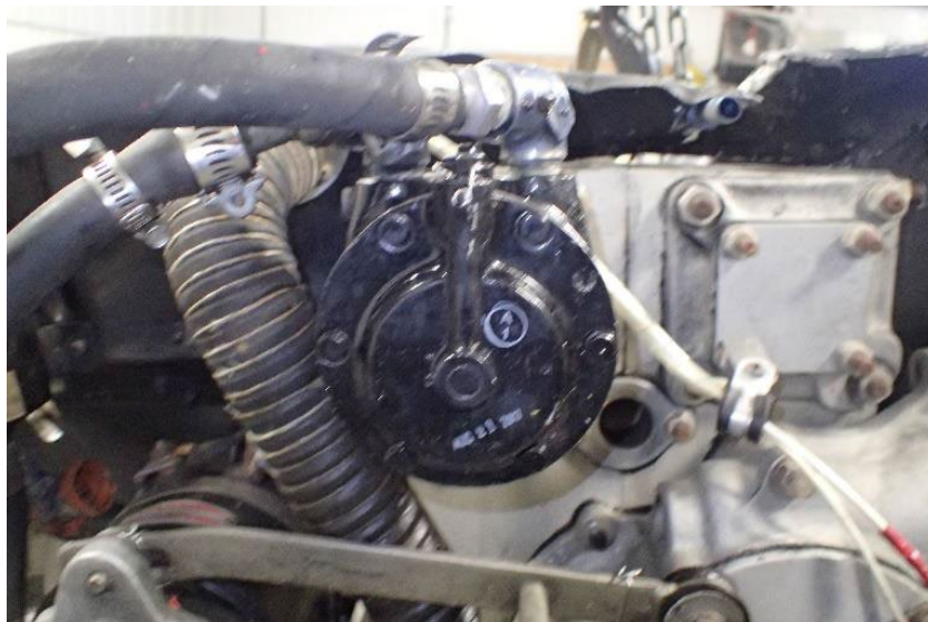
Figure 617 - Vacuum pump view #2
