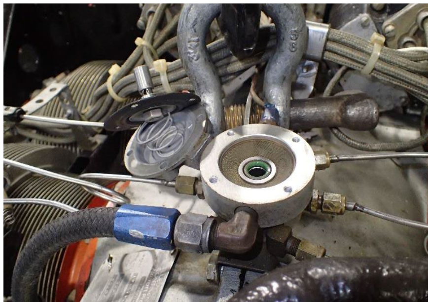
Figure 27 - fuel manifold valve
