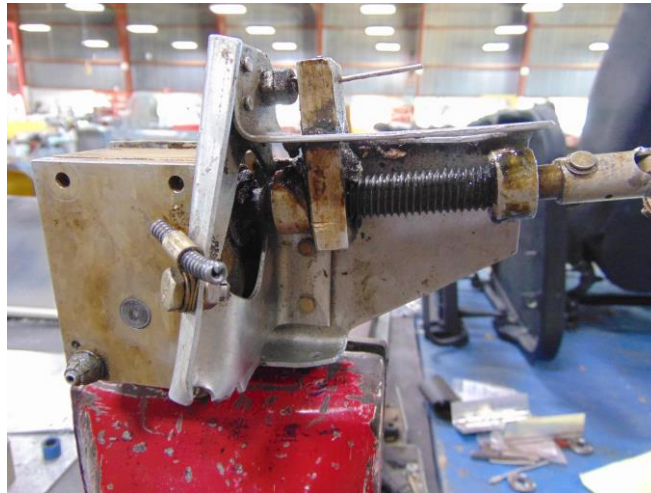
Lower portion of the stabilizer assembly, trim control mounted for testing
