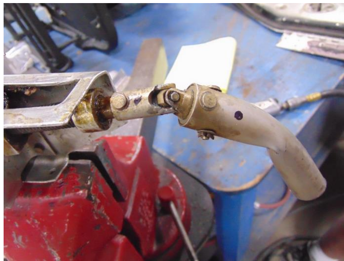
Universal joint and remaining piece of torque tube. The black dots were added as a reference of the alignment.
