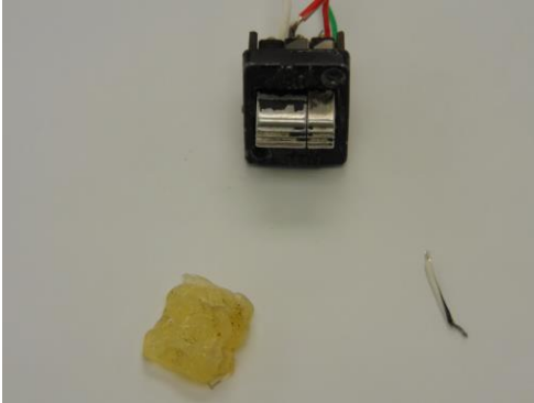
Elevator electric trim switch (front) with removed potting and detached wire
