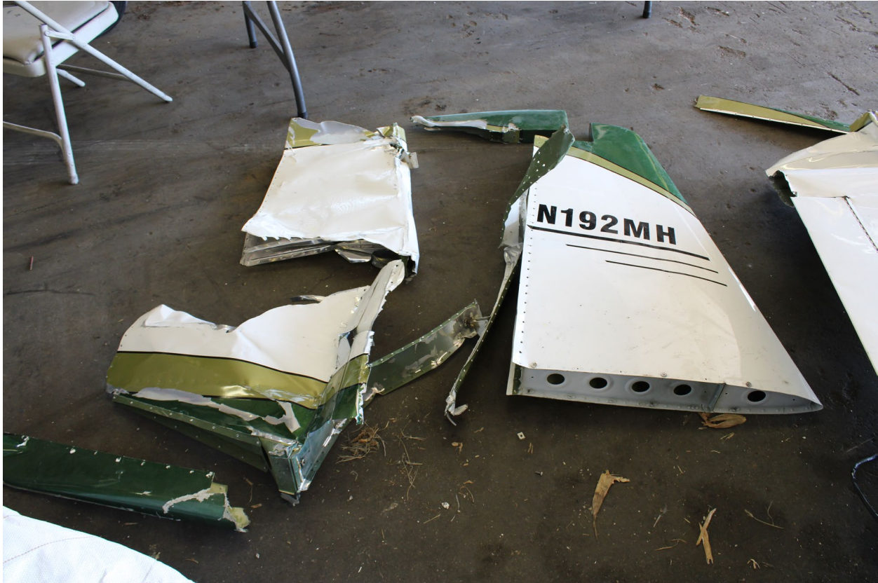
Figure 1. Separated vertical stabilizer and rudder.
