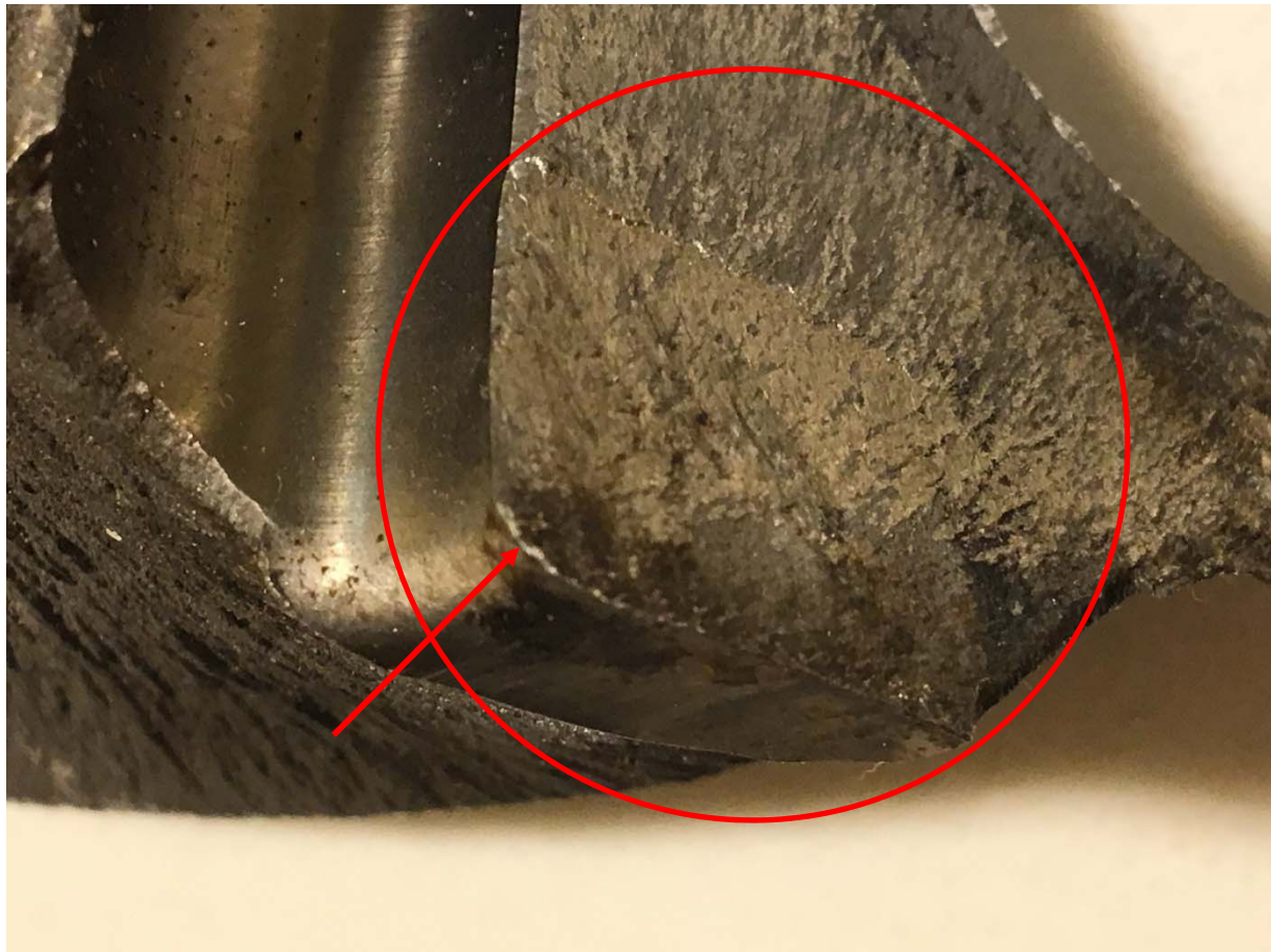
Figure 14 – 3 inch by 3 inch piece of main cylinder exhibiting features consistent with fatigue
