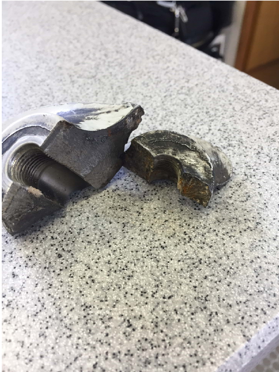
Figure 11 – Main cylinder pieces recovered from the runway
