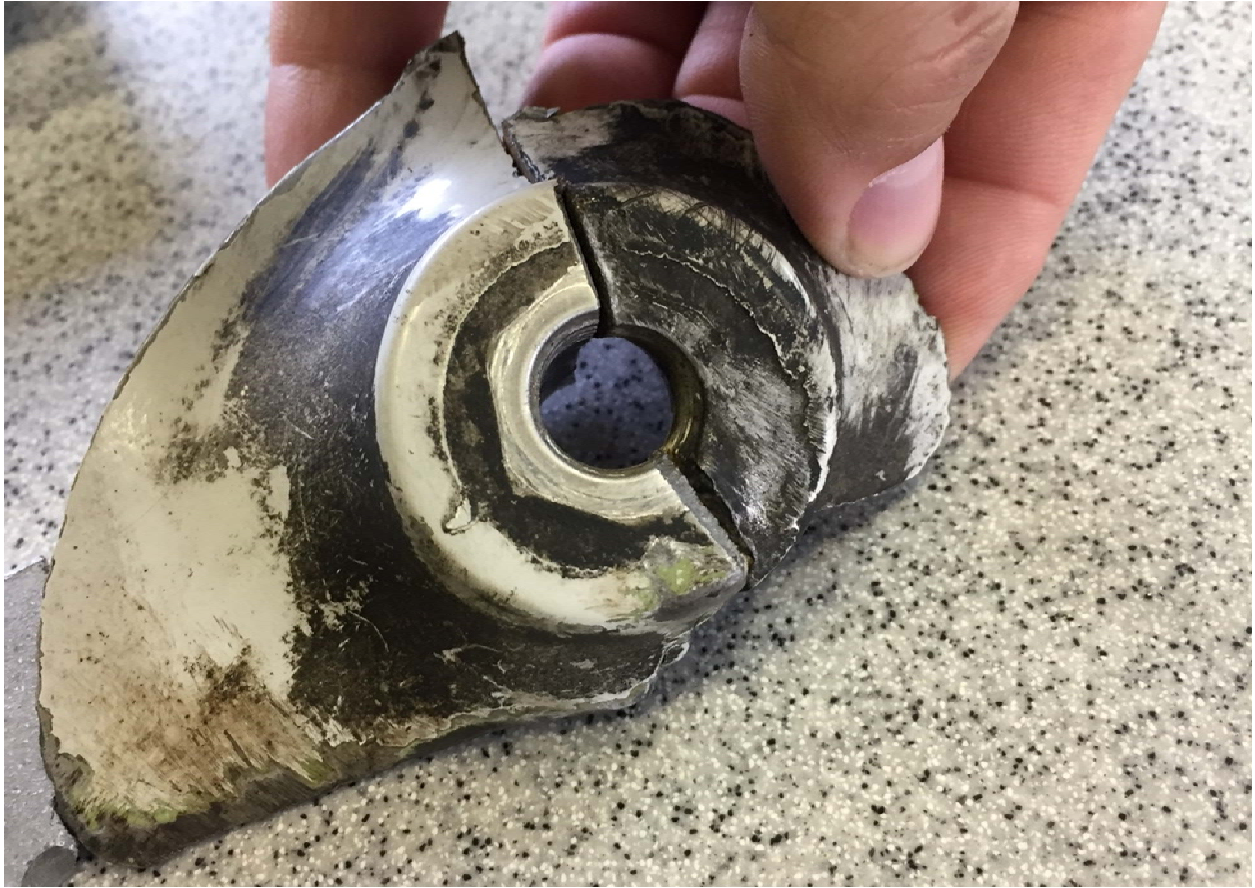
Figure 12 – Main cylinder pieces recovered from the runway
