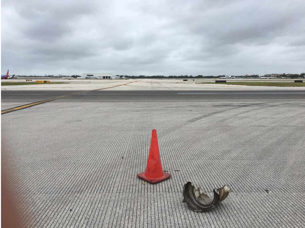
Figure 10 – Large section of main cylinder recovered from the runway
