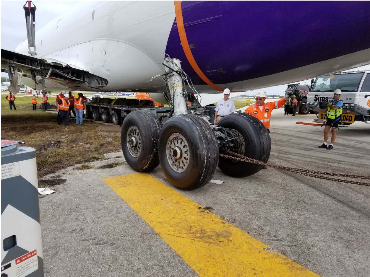
Figure 7 – Lower portion of the left main landing gear after being detached from the side brace
