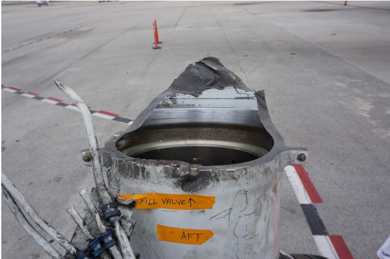
Figure 8 – Aft side of lower section of the main cylinder and fill valve
