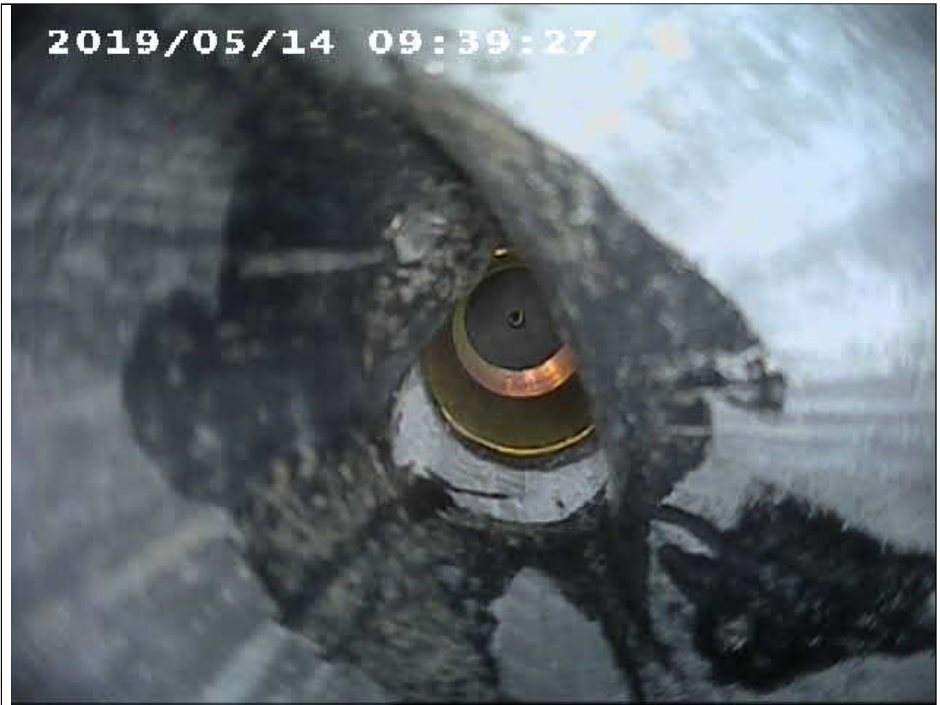
Figure 5: Kinked end under full vacuum.
