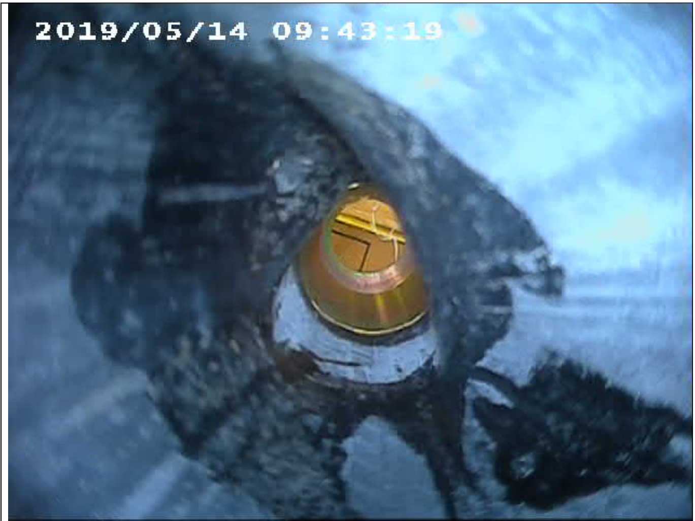
Figure 6: Kinked end under no vacuum,
