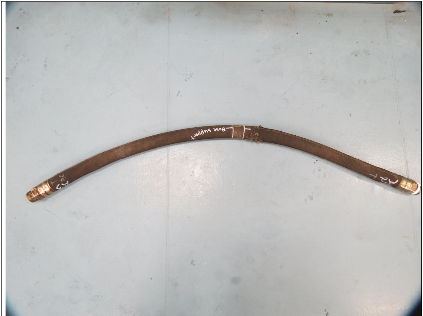
Figure 2: Assembly A2-A3. Has severe kink at end marked A2. Slight indentation at the opposite end fitting. Worn cover and some frayed wires at the hose support location. No leaks during pressure testing.
