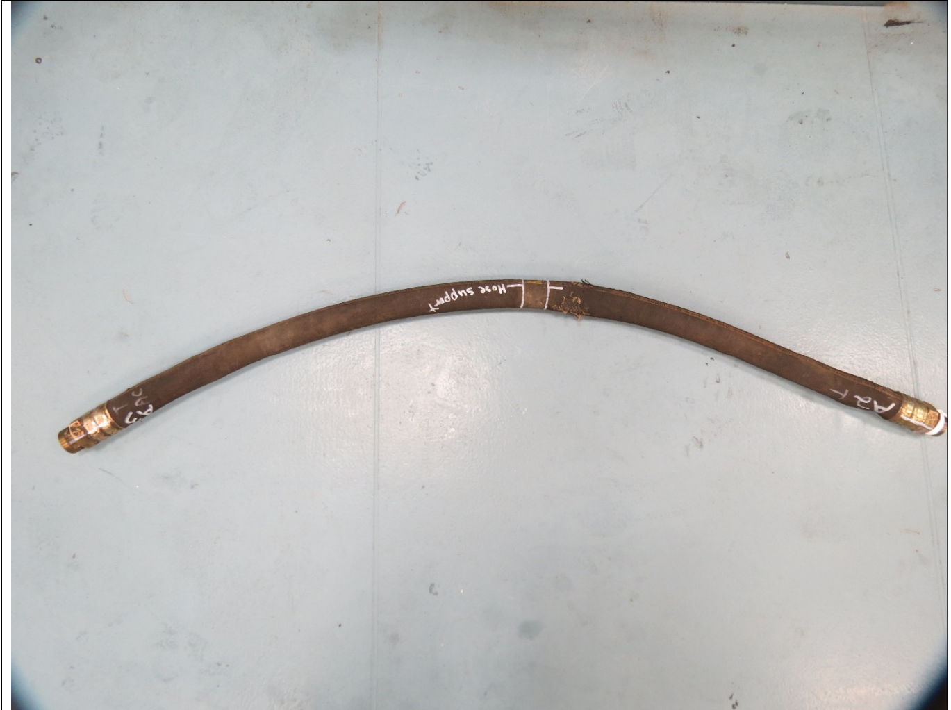
Figure 8: Assembly A2-A3. Has severe kink at end marked A2. Slight indentation at the opposite end fitting. No leaks during pressure testing.
