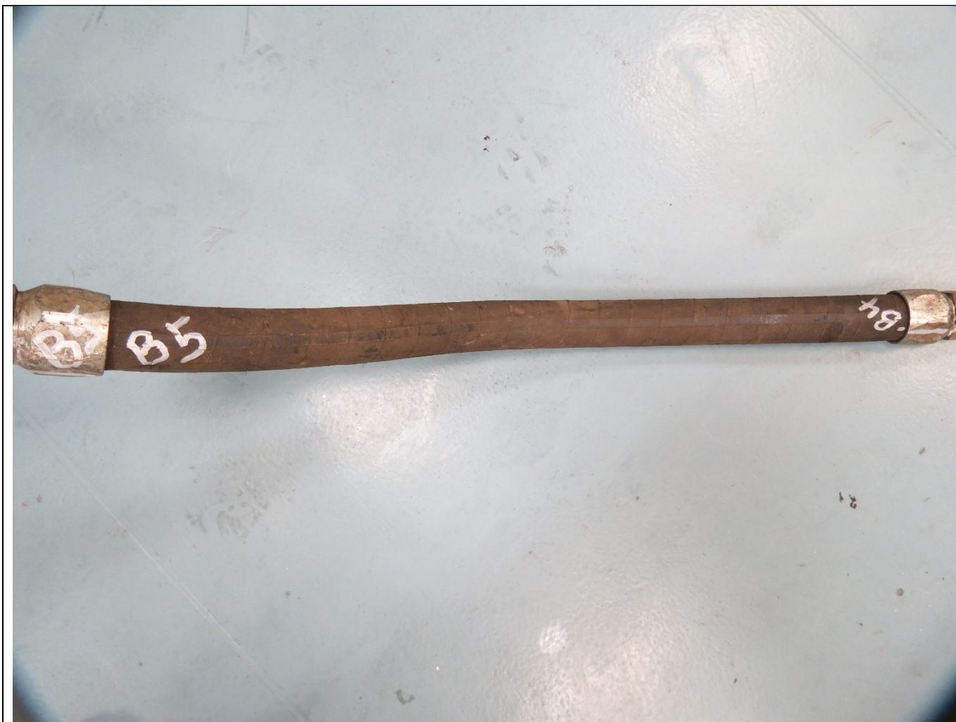
Figure 6: Assembly B4-B5. No external damage to the outside of the hose. No issues with the hose ID.
