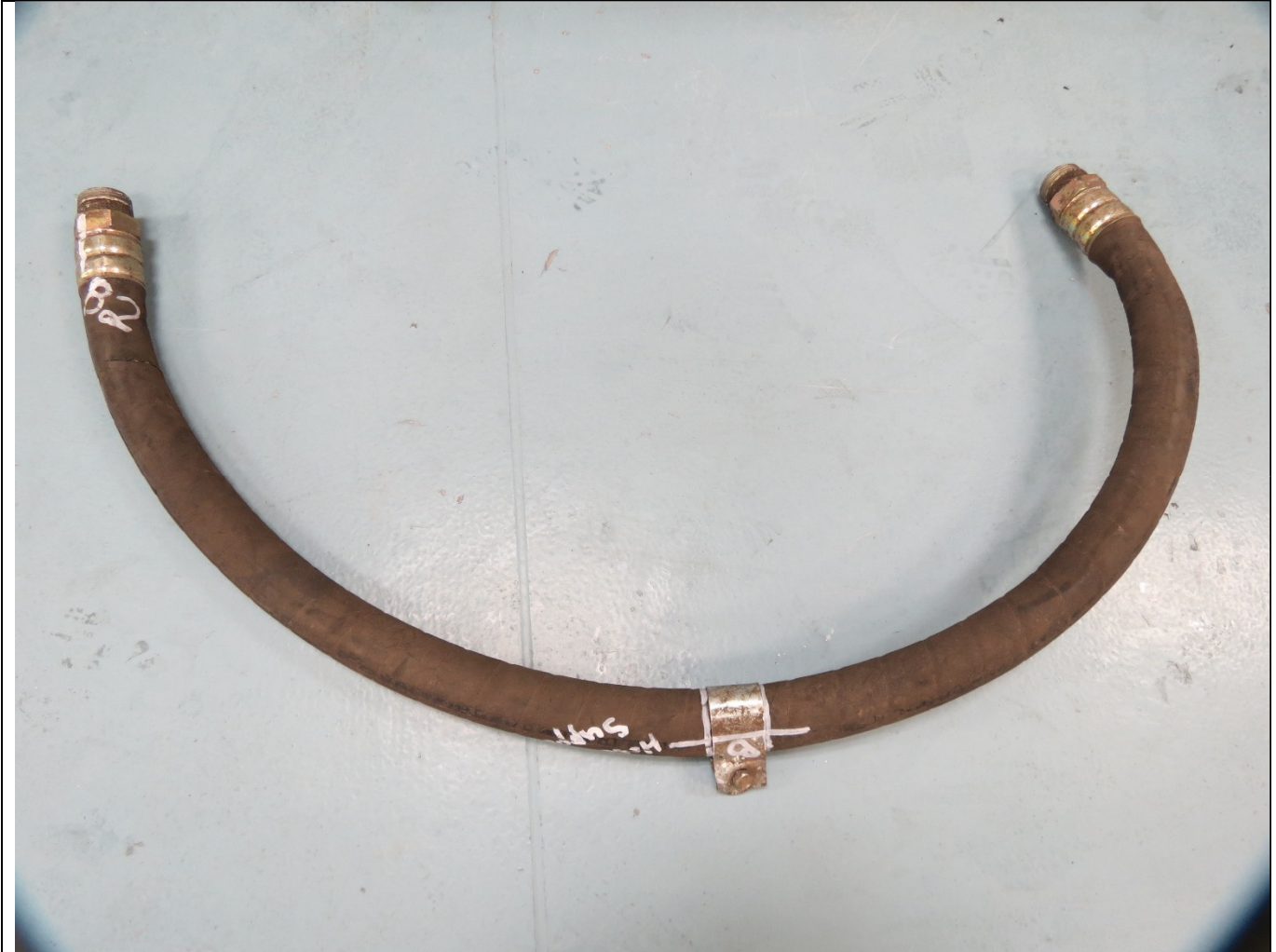
Figure 9: Assembly B2-B3. Severe damage at end mark B3. Also, some flattening at the support clamp.
