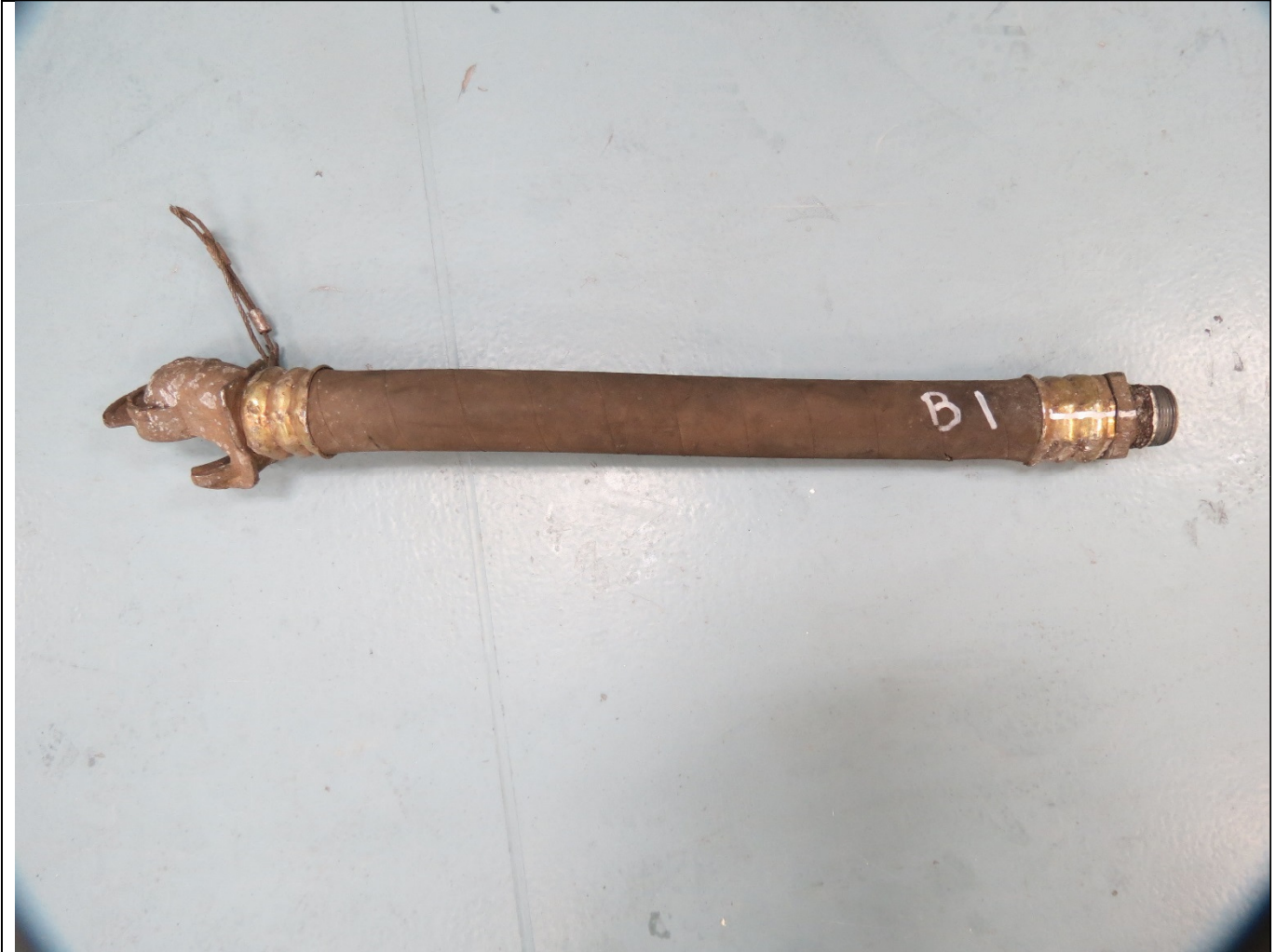
Figure 5: Assembly B1. Some cover damage at the end marked B1. No damage to the ID
