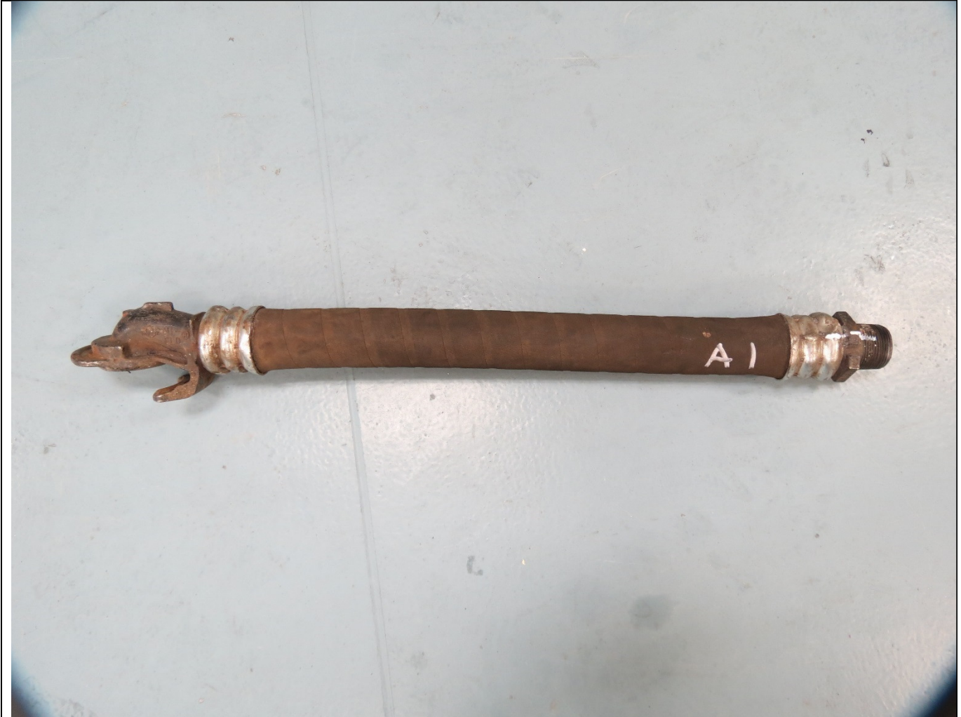
Figure 4: Assembly A1. No external damage. No issues with the ID of the assembly.
