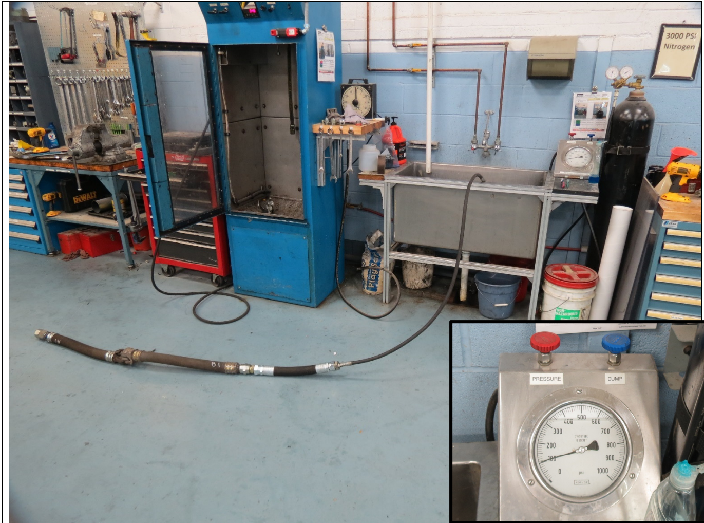
Figure 3: Pressure testing assemblies A1 and B1 with nitrogen at 100 psi. This set up was used to test all the assemblies.
