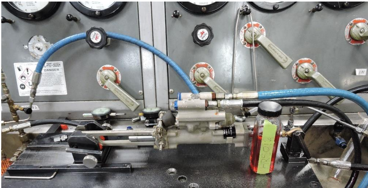
Figure 3. Servo HR5016 installed on the test bench with hydraulic fluid sample next to the servo body.
