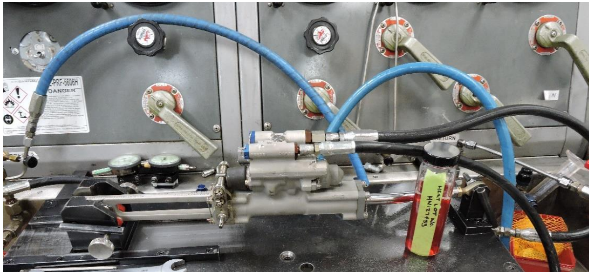
Figure 1. Servo HN127453 installed on the test bench with fluid sample positioned next to the servo body.
