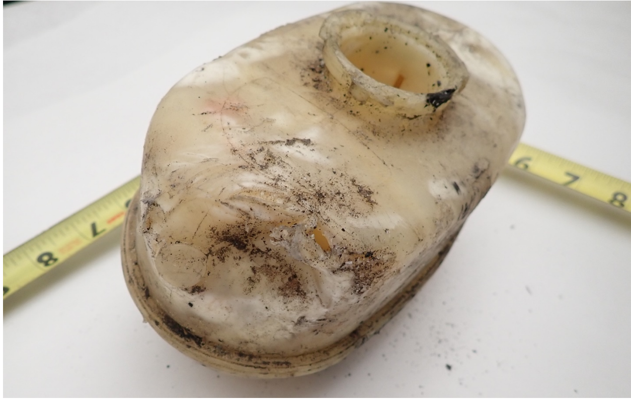
Vehicle Photograph: 25 - 2001 Ford Excursion Limousine – Damaged brake fluid reservoir.
