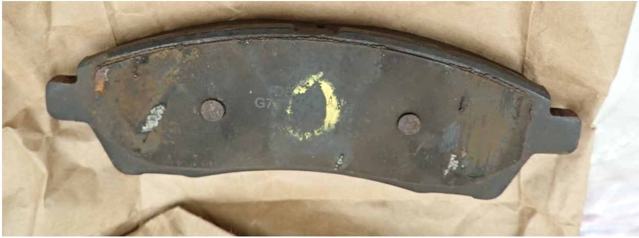
Vehicle Photograph: 14 - 2001 Ford Excursion Limousine: - Image shows the worn condition of the right rear brake pad backing plate.
