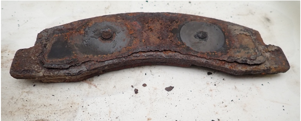
Vehicle Photograph: 18 - 2001 Ford Excursion Limousine – Image shows the severely deteriorated metal backing plate of the left front brake pad.
