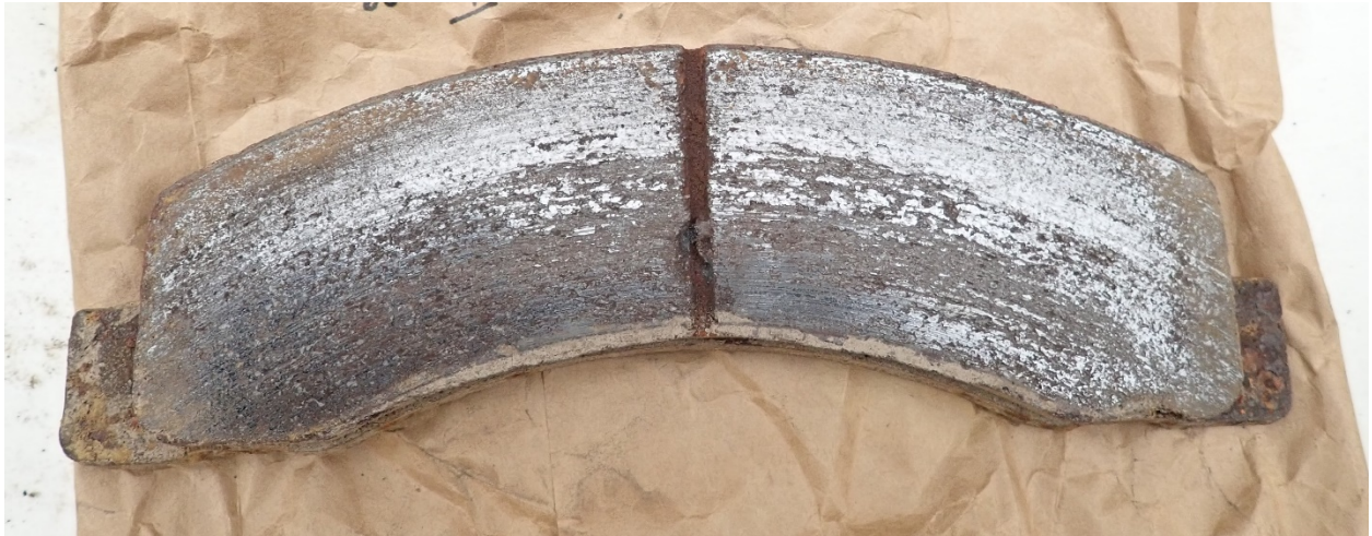
Vehicle Photograph: 22 - 2001 Ford Excursion Limousine - Friction surface of the right front brake pad.
