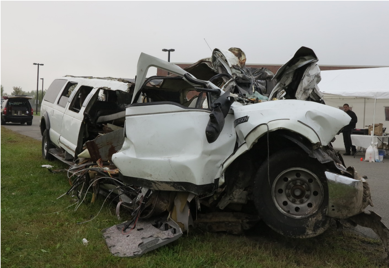
Vehicle Photograph: 2 - 2001 Ford Excursion Limousine – Overall damage view facing right front corner.
