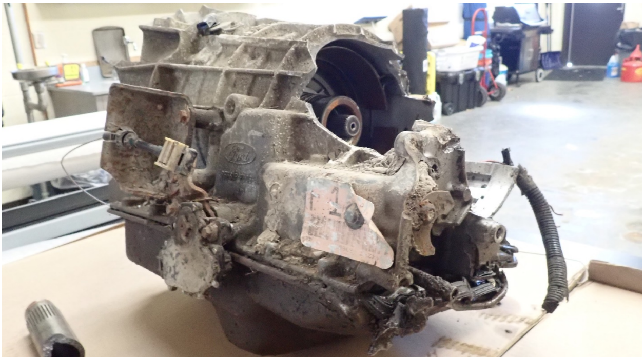
Vehicle Photograph: 29 - 2001 Ford Excursion Limousine - Fractured transmission main case.
