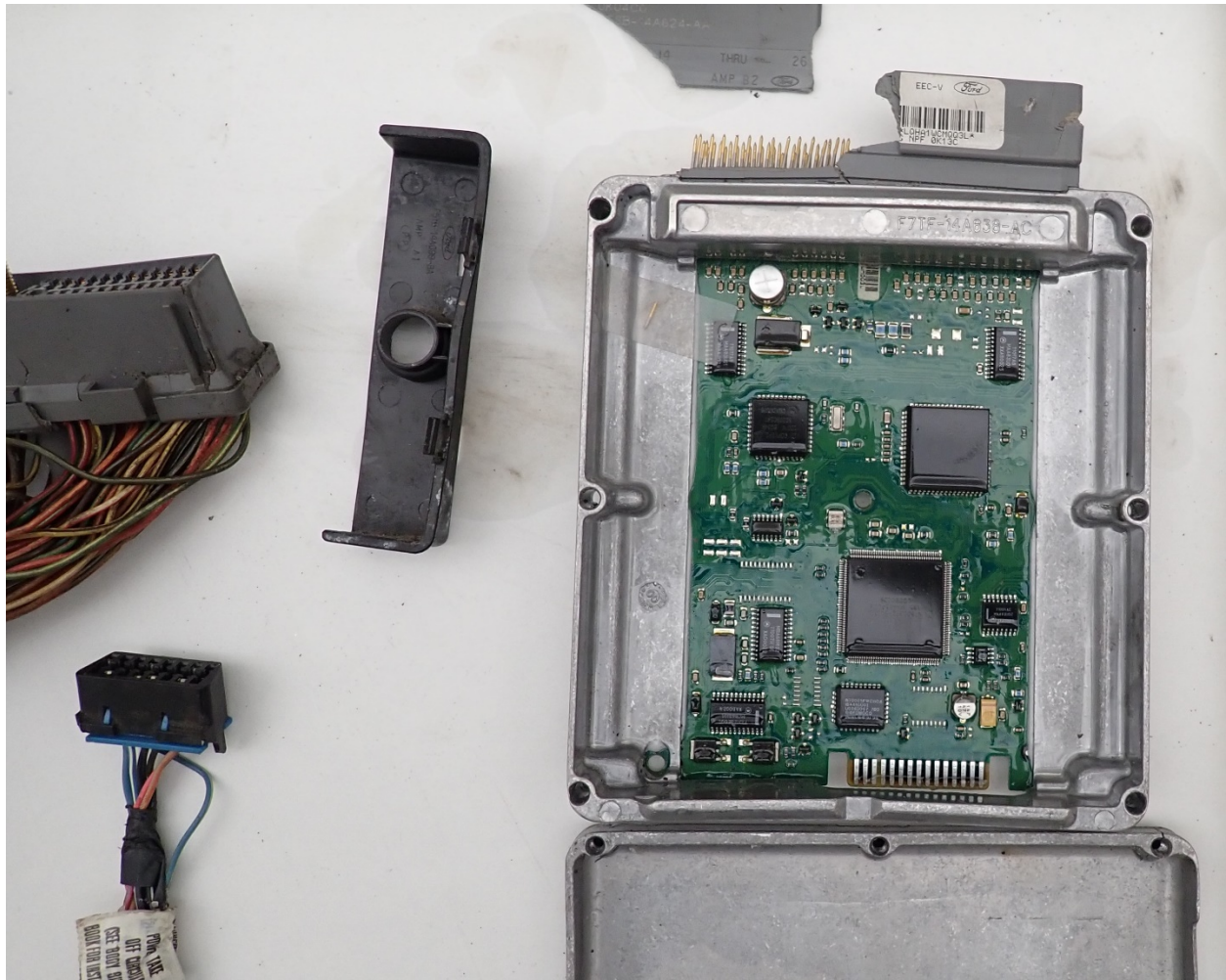
Vehicle Photograph: 32 - 2001 Ford Excursion Limousine – Damaged Ford powertrain control module.
