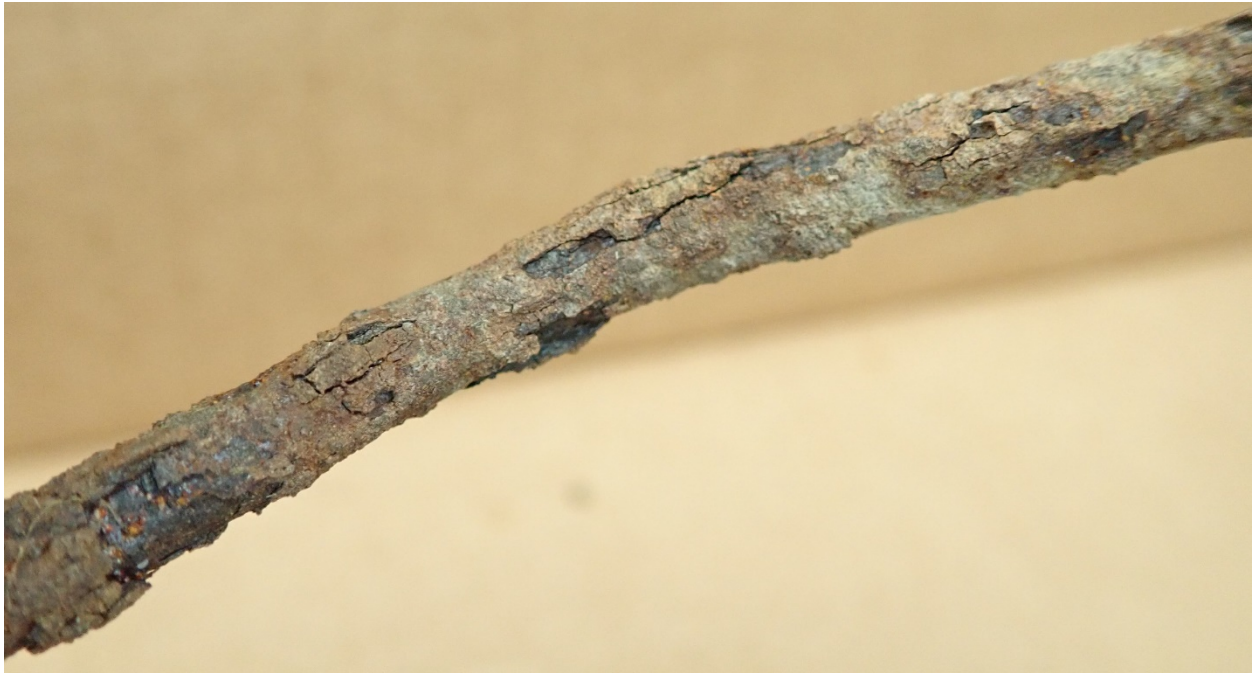
Vehicle Photograph: 26 - 2001 Ford Excursion Limousine – Close-up image of the corroded steel tubing removed from the rear brake system.
