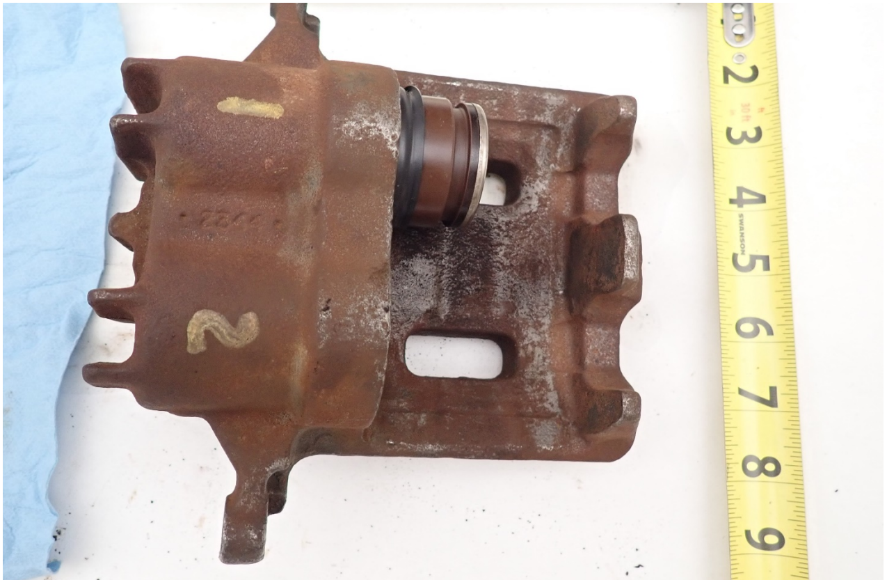
Vehicle Photograph: 7 - 2001 Ford Excursion Limousine – Left rear brake caliper showing one piston partially extruding from the piston bore.
