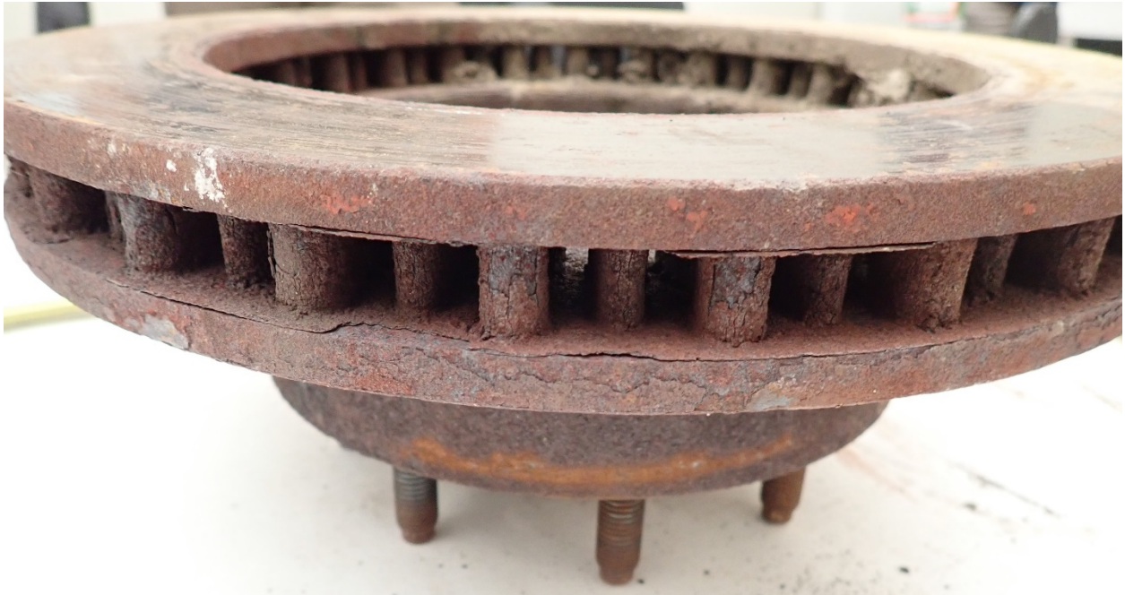
Vehicle Photograph: 16 - 2001 Ford Excursion Limousine – Image shows the corrosion present on the left front brake rotor vent vanes.
