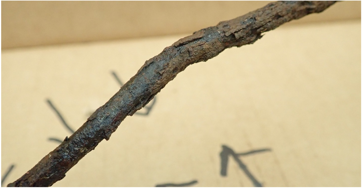
Vehicle Photograph: 28 - 2001 Ford Excursion Limousine – Image shows a portion of the corroded steel brake tubing with a coating of brake fluid.
