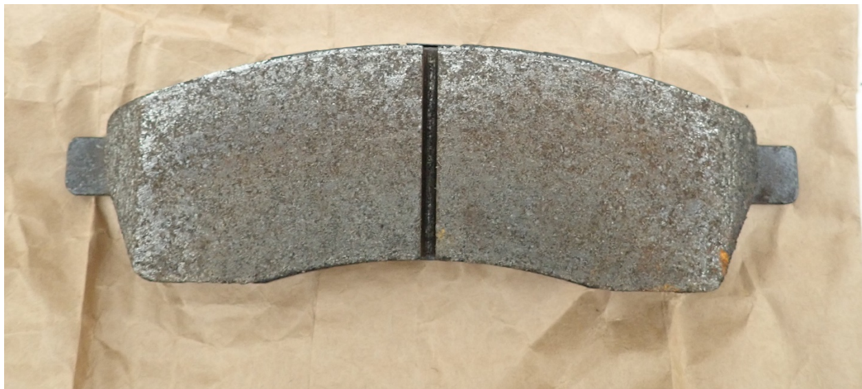
Vehicle Photograph: 9 - 2001 Ford Excursion Limousine - Friction surface of the left rear brake pad.
