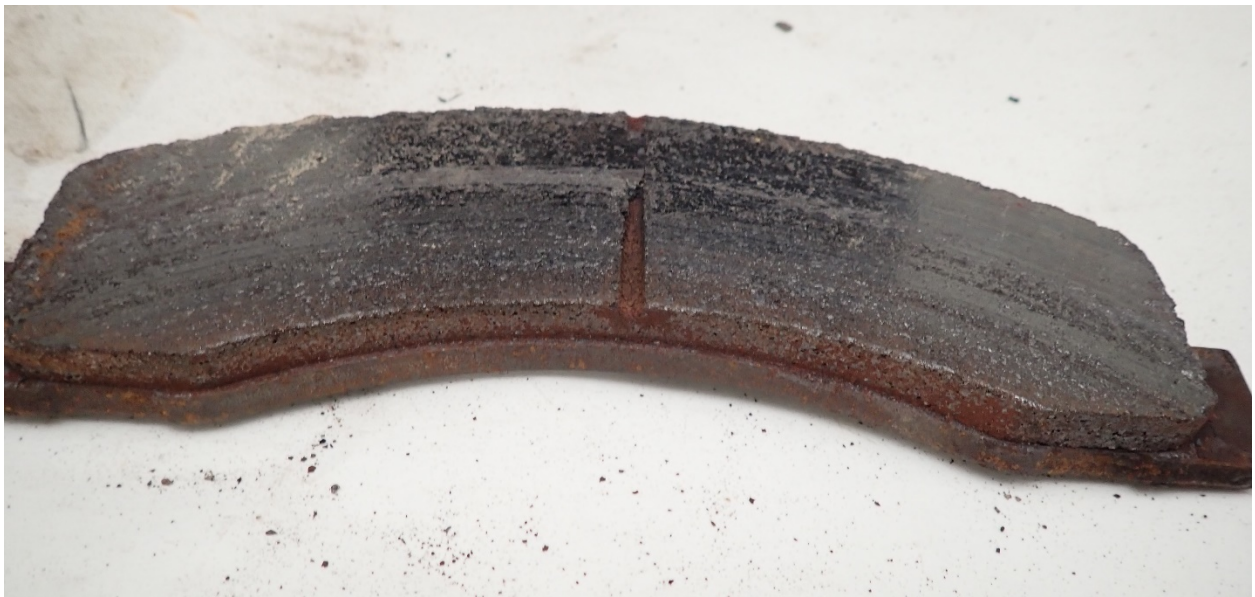
Vehicle Photograph: 17 - 2001 Ford Excursion Limousine - Friction surface of the left front brake pad.
