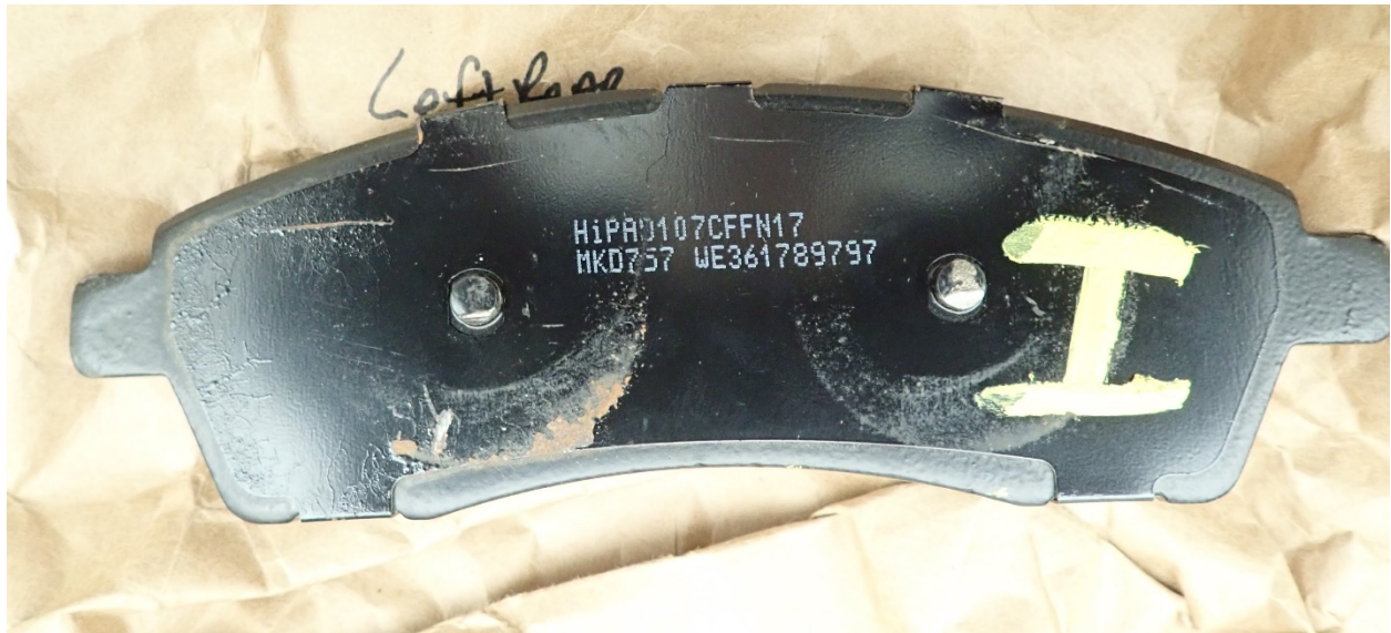
Vehicle Photograph: 10 - 2001 Ford Excursion Limousine – Image shows the backing plate of the left rear brake pad. It is in good condition and identifying markings are present.
