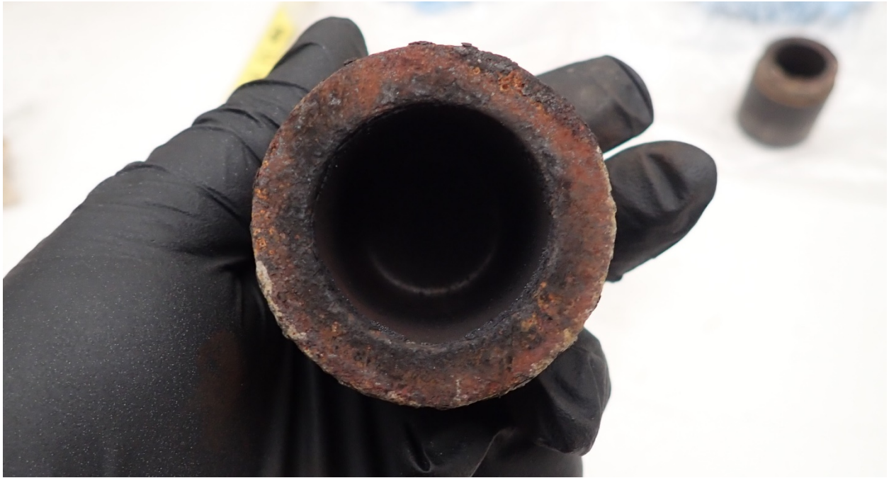
Vehicle Photograph: 20 - 2001 Ford Excursion Limousine – Image shows the severely corroded right front caliper piston shield.
