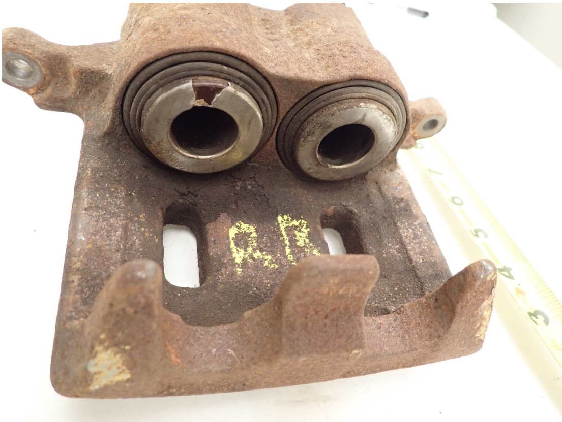
Vehicle Photograph: 11- 2001 Ford Excursion Limousine – Image shows the right rear disc brake caliper and damage to one of the pistons.
