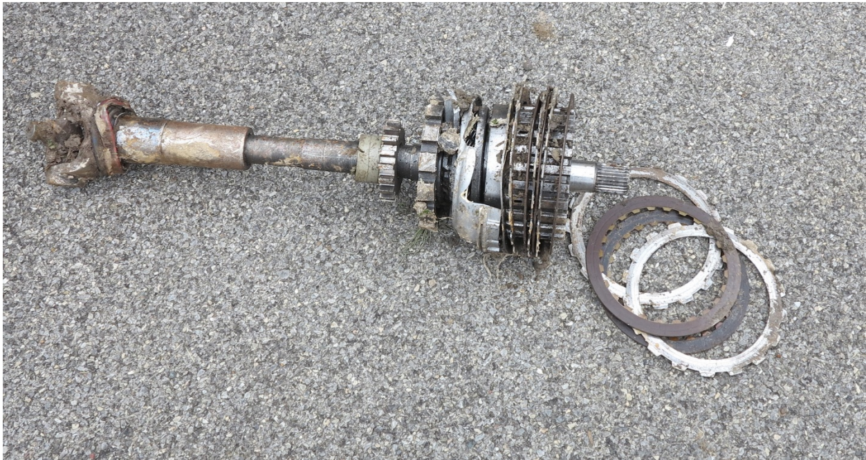
Vehicle Photograph: 30 - 2001 Ford Excursion Limousine – Image shows the damaged transmission output shaft which was displaced from the vehicle during the crash.
