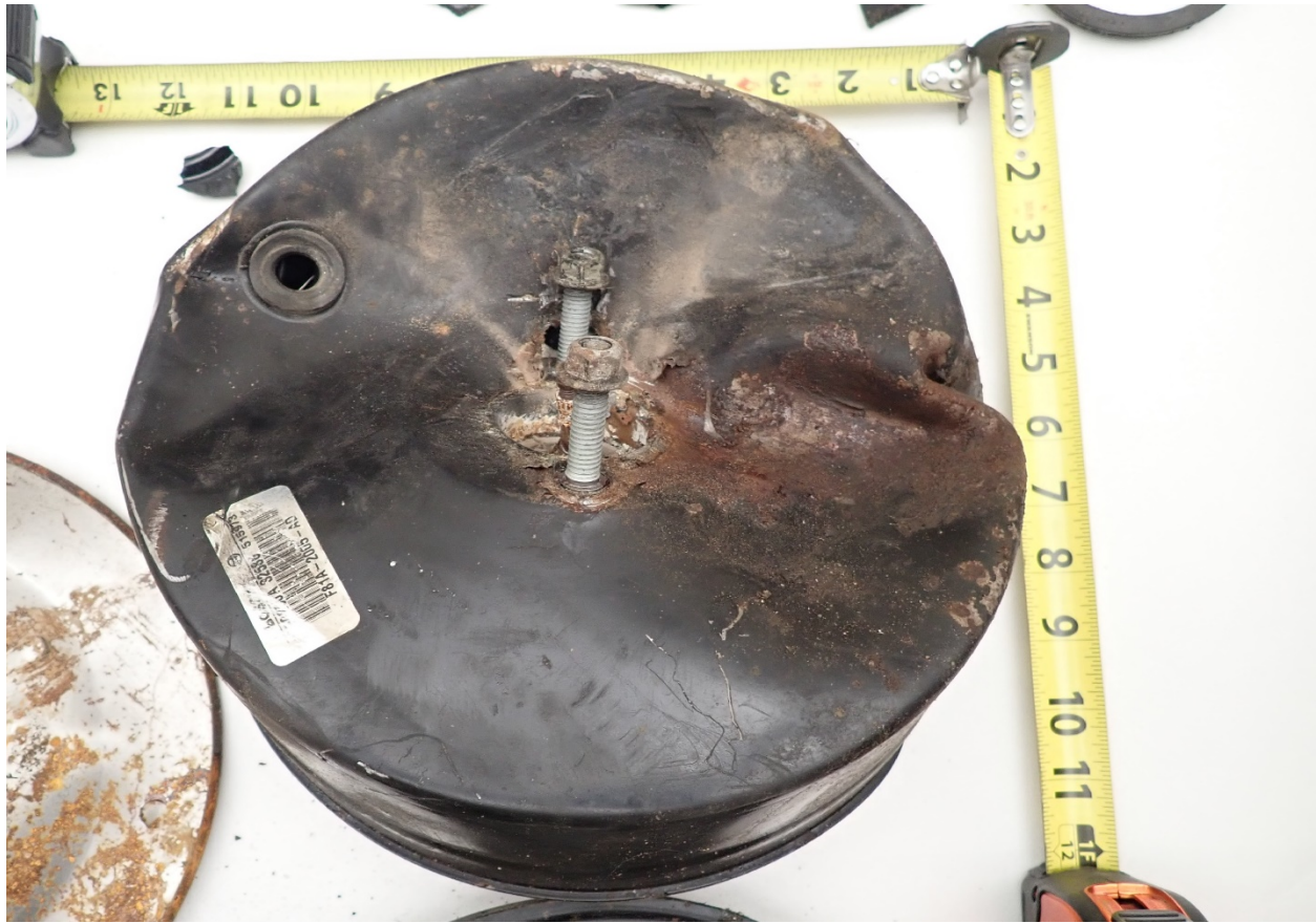
Vehicle Photograph: 24 - 2001 Ford Excursion Limousine - Damaged brake vacuum booster.
