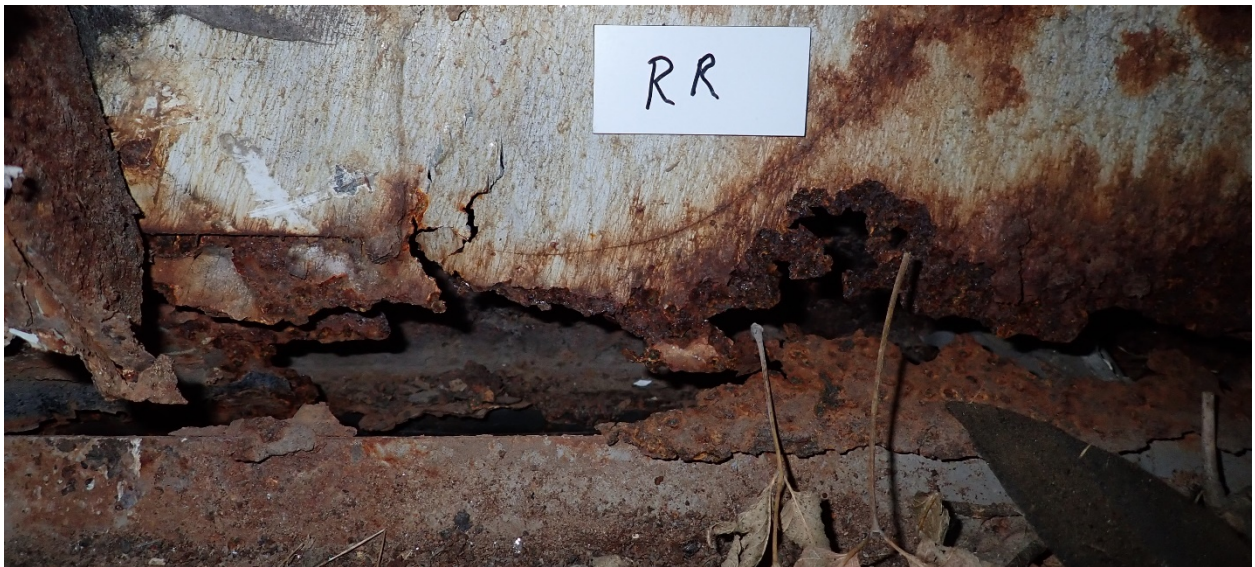
Vehicle Photograph: 4 - 2001 Ford Excursion Limousine – Image documents the severe corrosion present on the right rear of the vehicle chassis.
