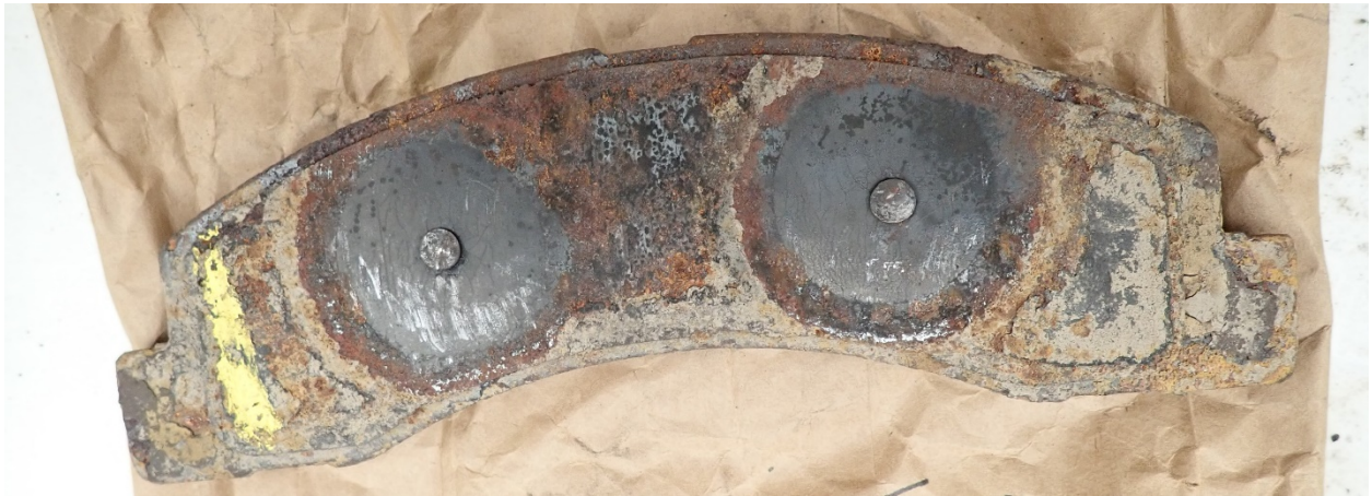
Vehicle Photograph: 23- 2001 Ford Excursion Limousine - Image shows the severely deteriorated metal backing plate of the right front brake pad.
