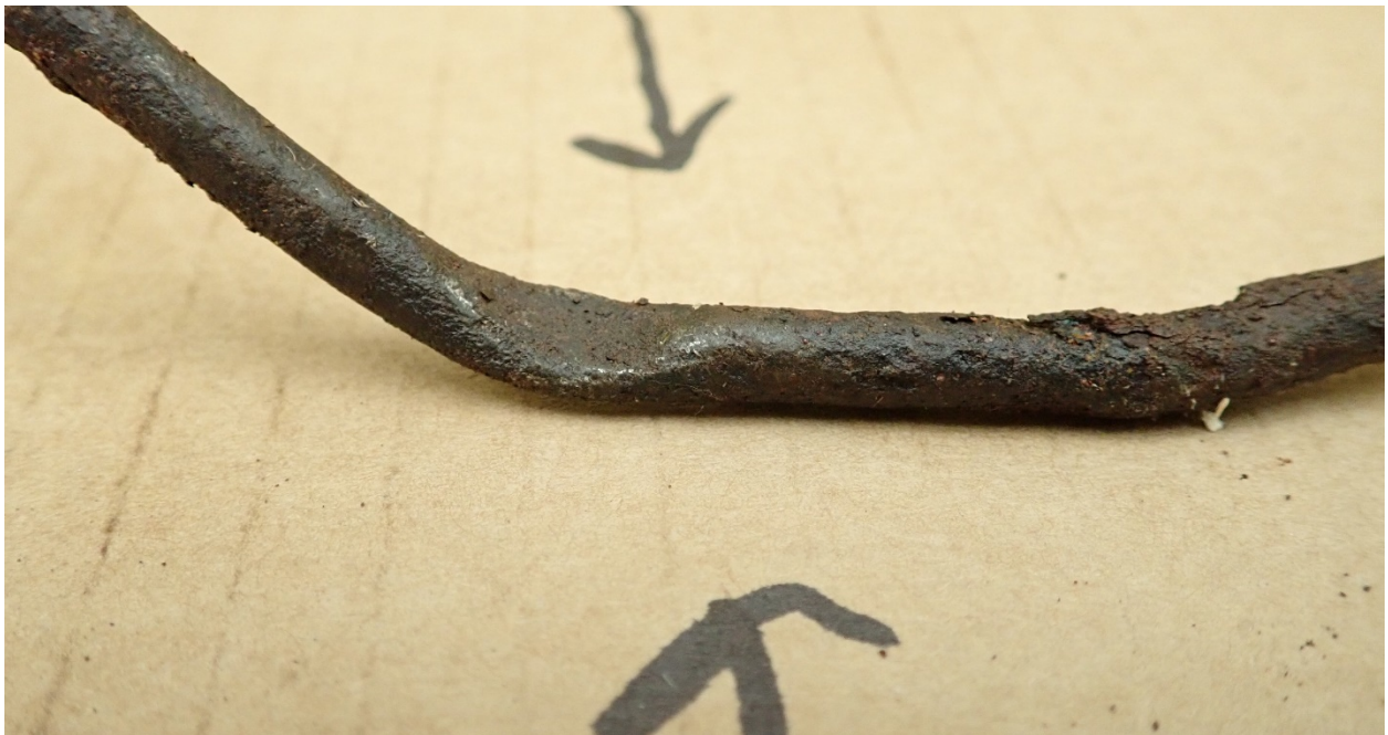
Vehicle Photograph: 27 - 2001 Ford Excursion Limousine – Image shows a crimp in the rear hydraulic brake tubing with corrosion present.
