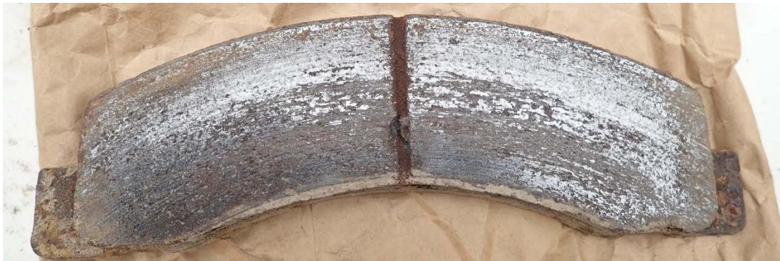
Figure 23: Inner Pad Friction Surface from Right Front Brake
