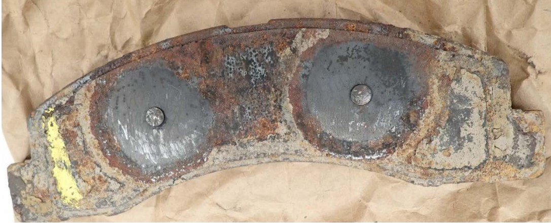
Figure 24: Metal Pad Backing Plate from Right Front Brake
