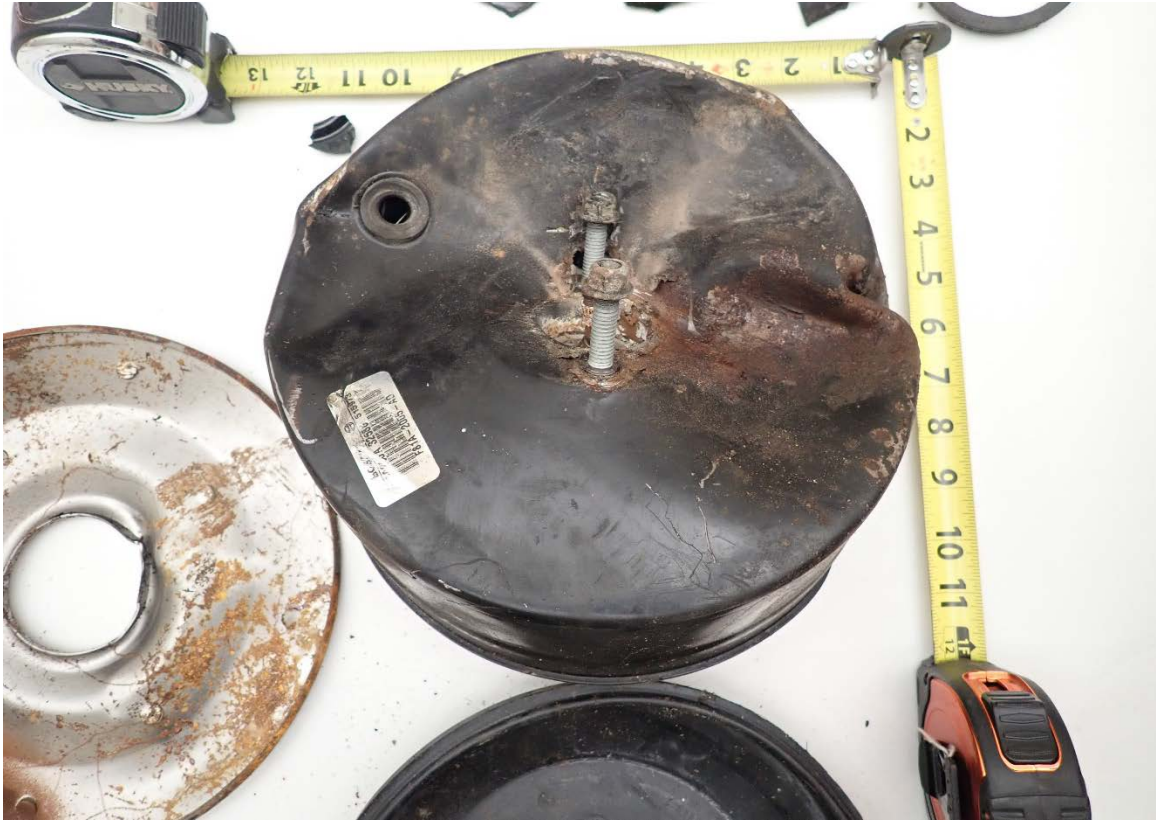
Figure 25: Damaged Brake Vacuum Booster
