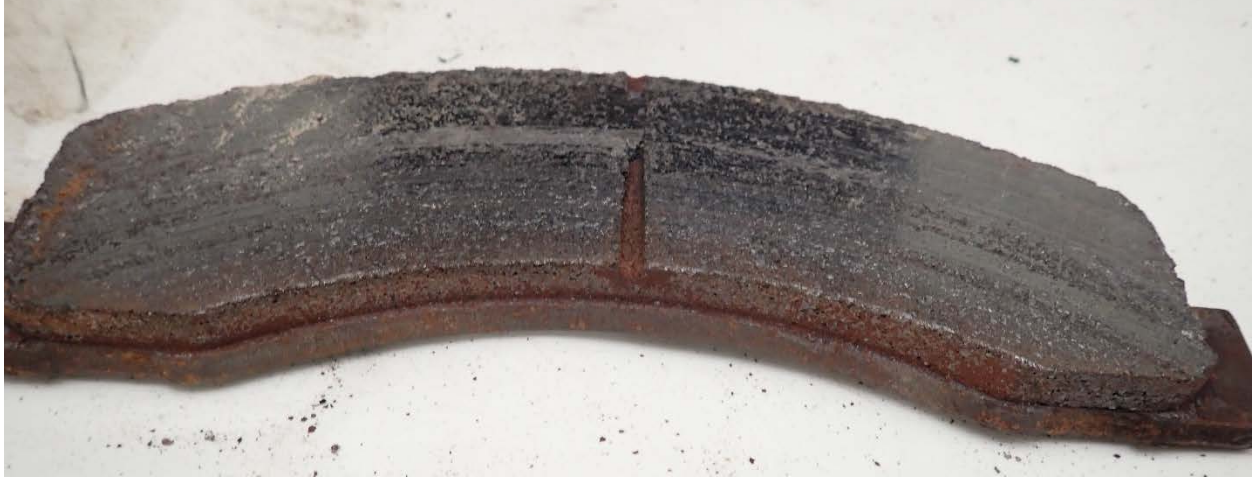
Figure 18: Friction Surface of Left Front Brake Pad
