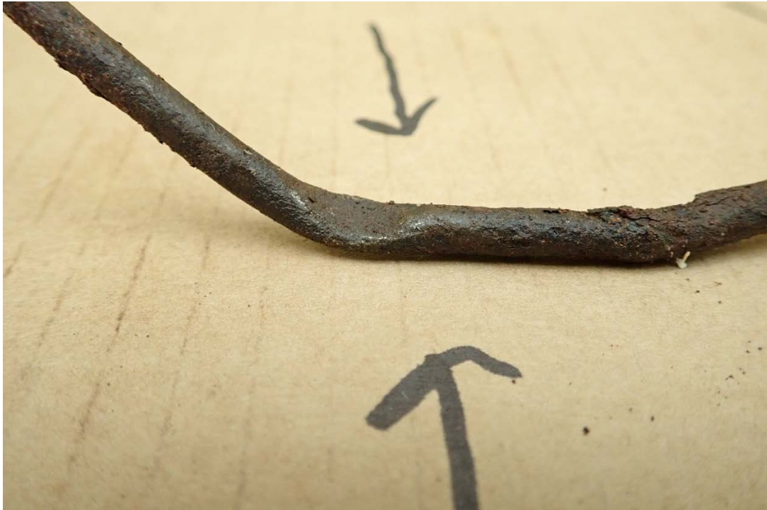
Figure 28: Crimped and Corroded Steel Tubing from Limousine Brake System
