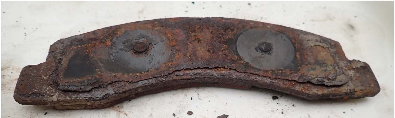
Figure 19: Metal Backing Plate of Left Front Brake Pad
