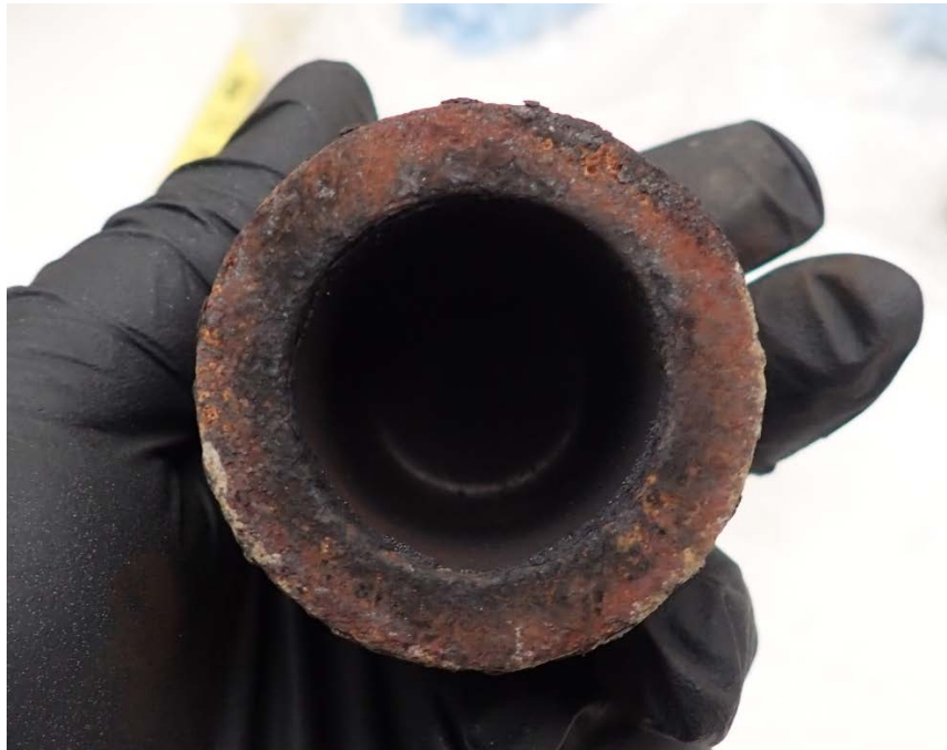
Figure 21: Corroded Right Front Caliper Piston
