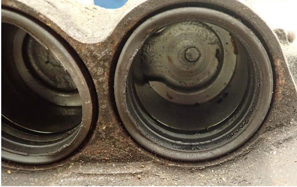
Figure 16: Interior of the Left Front Caliper Piston Bores
