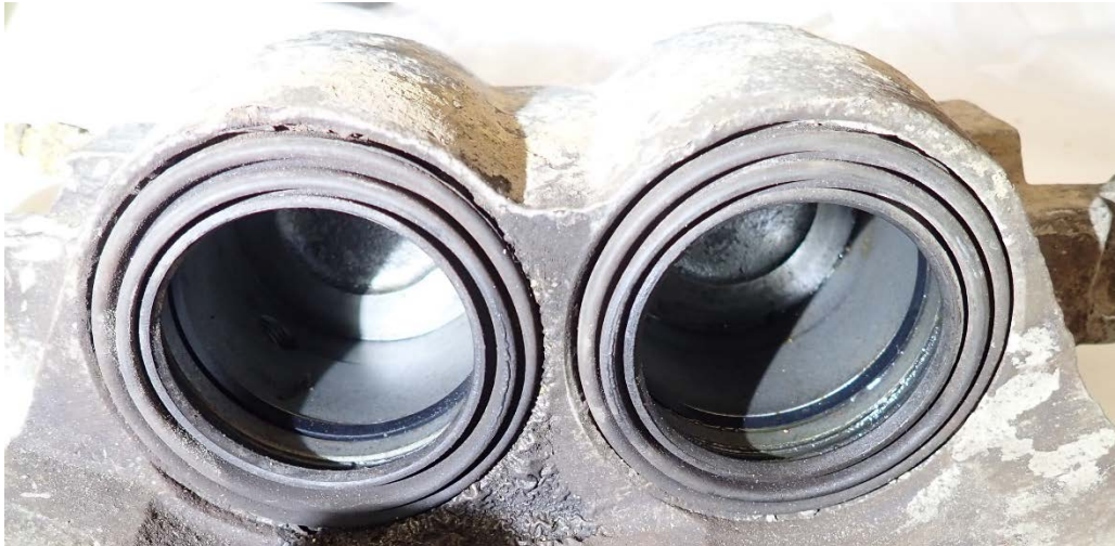
Figure 20: Interior of Right Front Caliper Piston Bore
