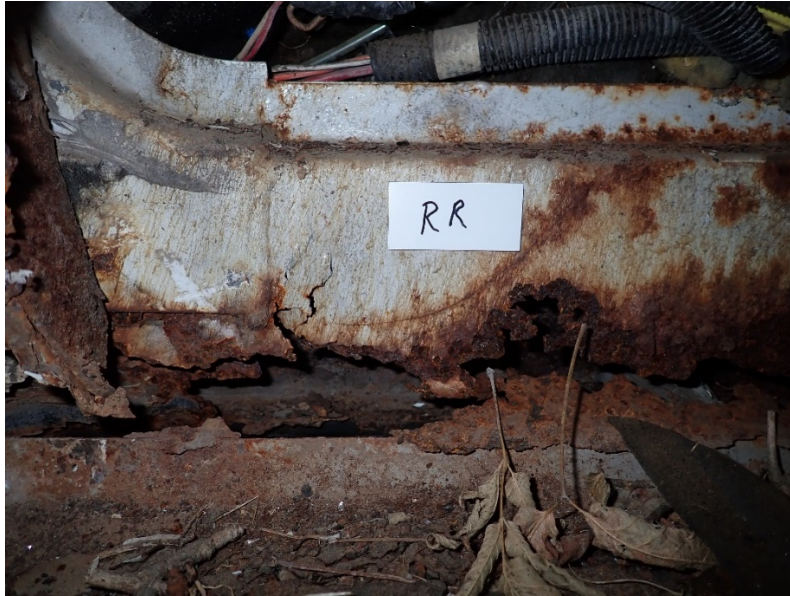
Figure 5: Corrosion to Right Rear Chassis
