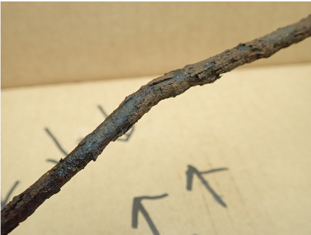
Figure 29: Corroded Steel Tubing with Brake Fluid Coating
