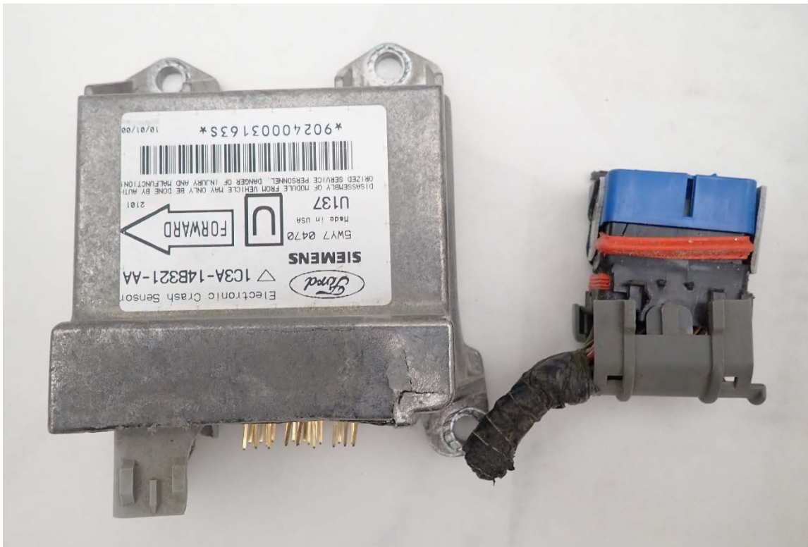
Figure 32: Damaged ACM from Ford Limousine
