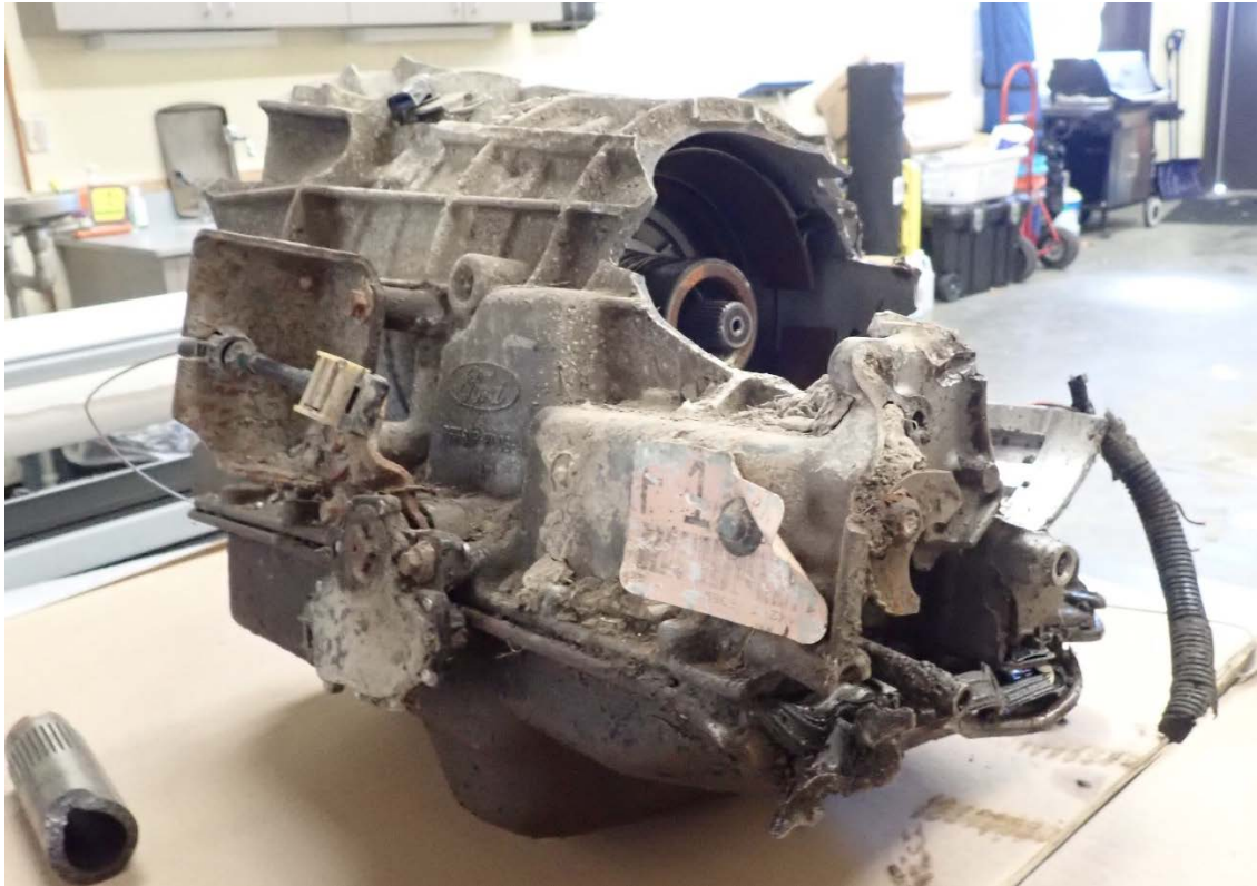
Figure 30: Fractured Transmission Main Case of Limousine
