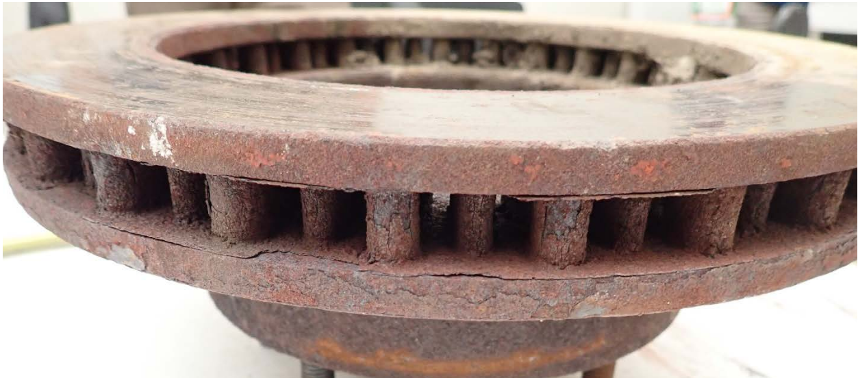
Figure 17: Left Front Brake Rotor Vent Vanes
