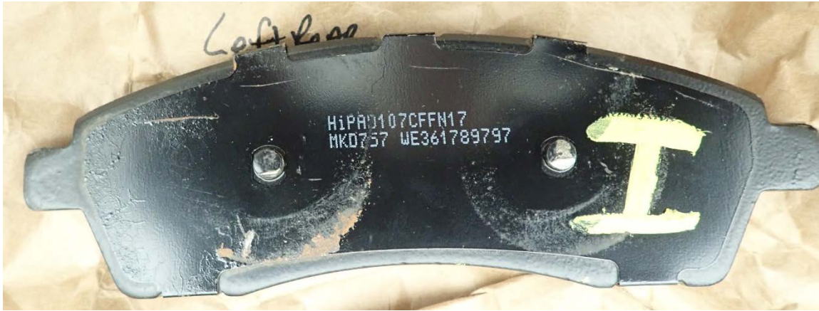
Figure 11: Backing Plate of Left Rear Brake Pad
