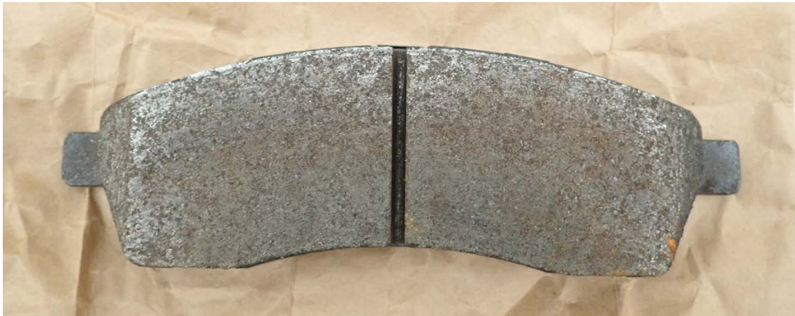
Figure 10: Friction Surface of Left Rear Brake Pad
