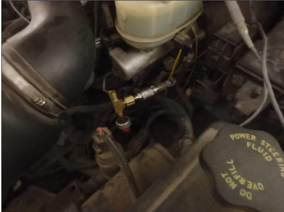
NATC Photograph Number 22330-0029 Instrumentation – Master Cylinder Rear Brake Pressure
