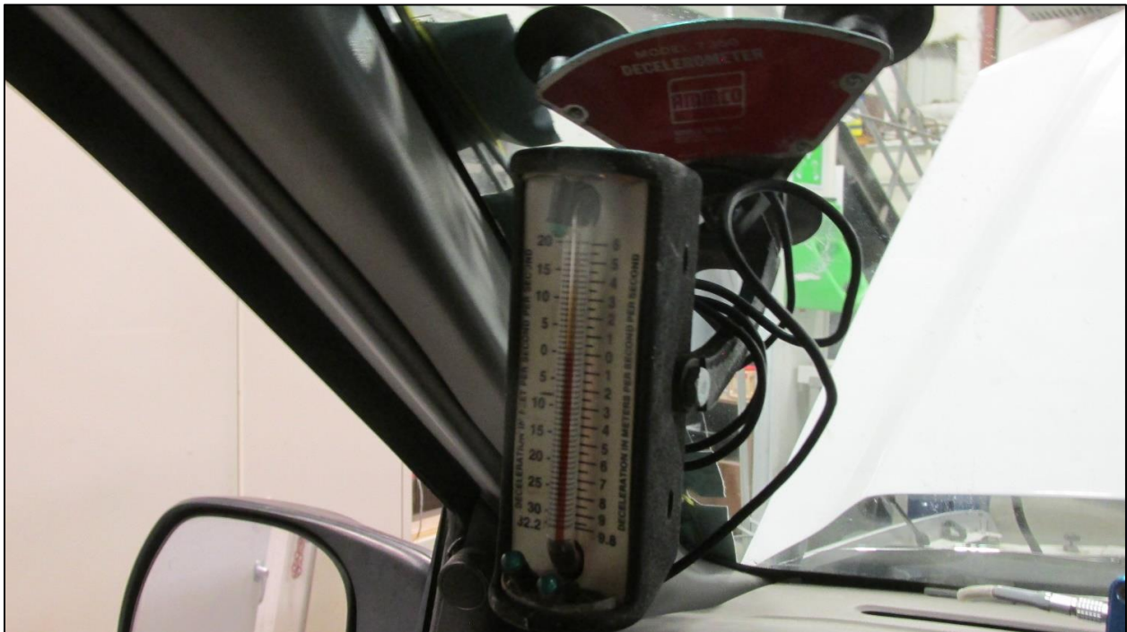
NATC Photograph Number 22330-0012 Instrumentation – Decelerometer
