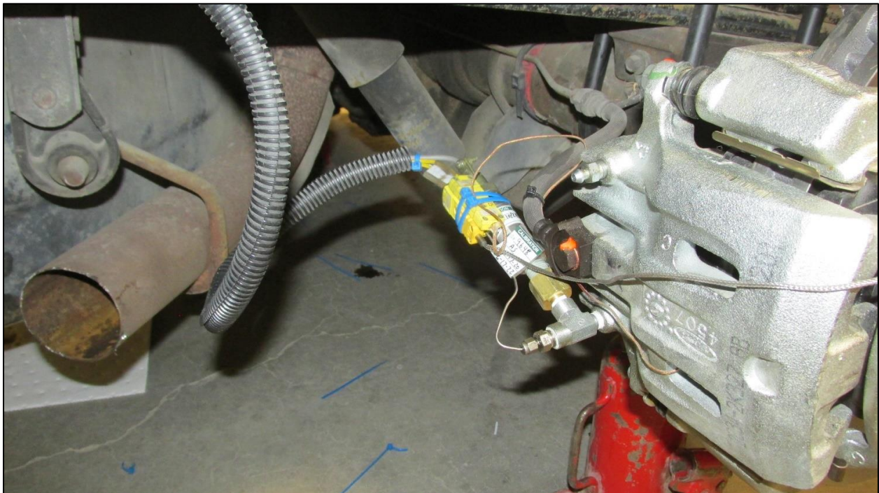
NATC Photograph Number 22330-0020 Instrumentation – Curbside Rear Brake Pressure Transducer
