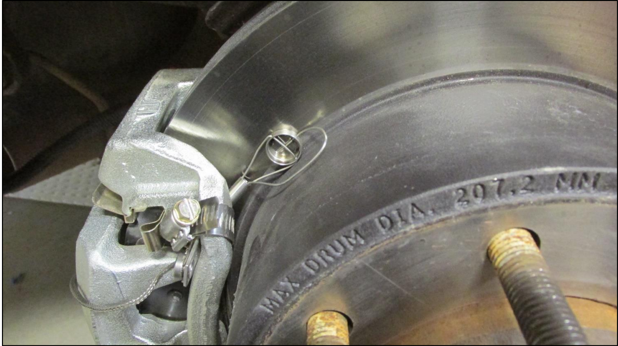
NATC Photograph Number 22330-0021 Instrumentation – Curbside Rear Rotor Thermocouple
