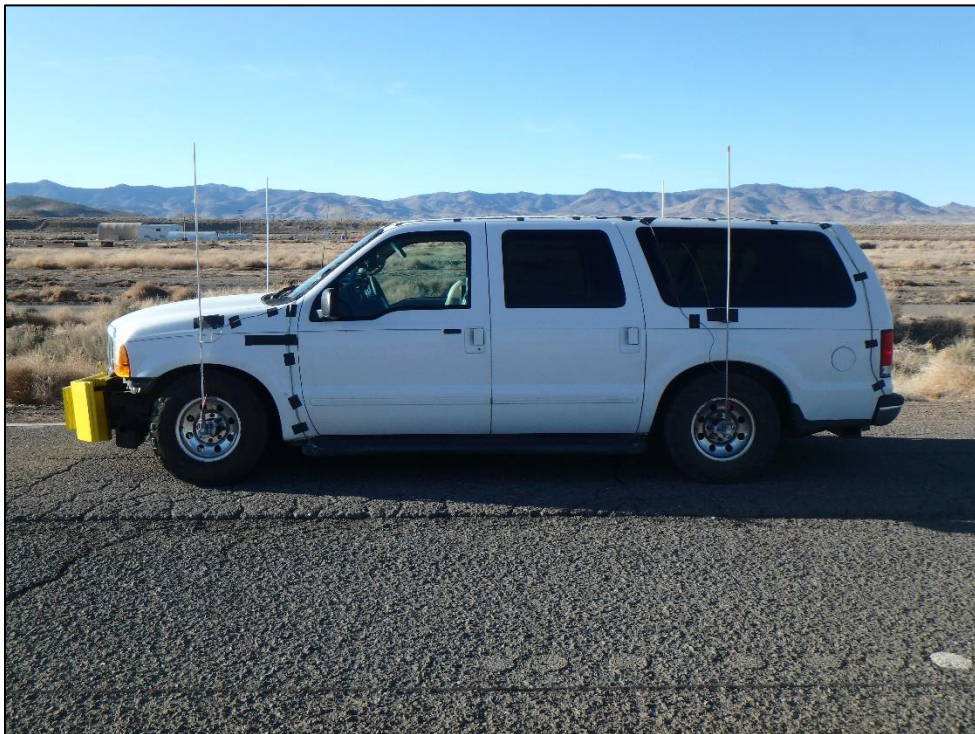
NATC Photograph Number 22330-0008 Instrumentation – Roadside Wheel Encoders
