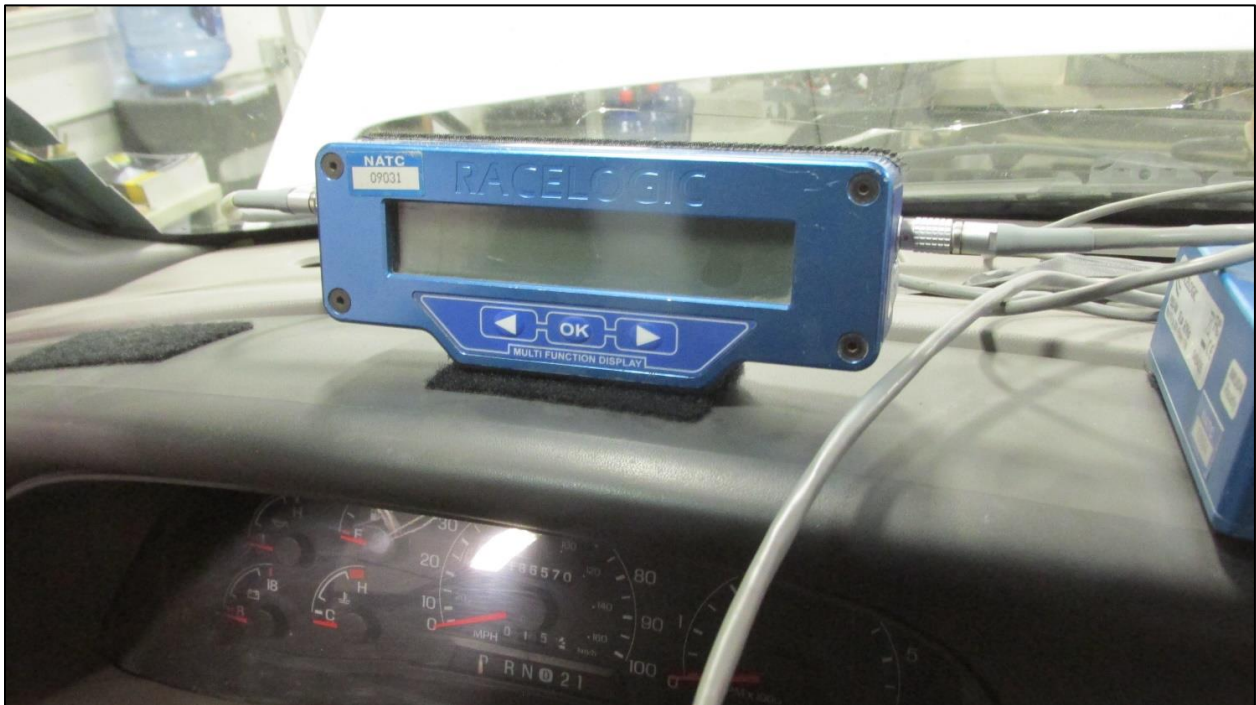
NATC Photograph Number 22330-0014 Instrumentation – VBOX Display
