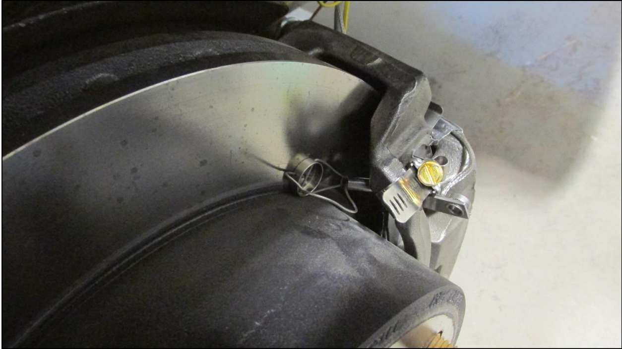
NATC Photograph Number 22330-0023 Instrumentation – Roadside Rear Rotor Thermocouple
