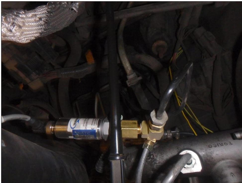
NATC Photograph Number 22330-0028 Instrumentation – Master Cylinder Front Brake Pressure
