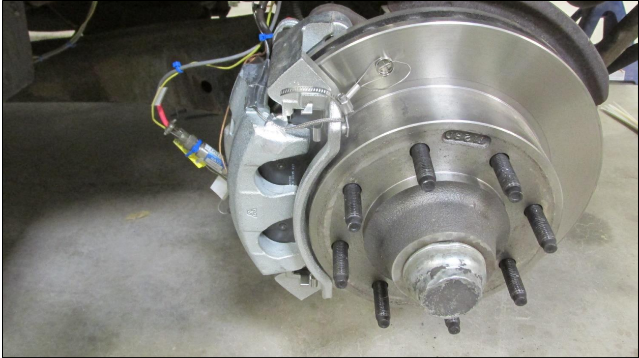
NATC Photograph Number 22330-0025 Instrumentation – Curbside Front Rotor Thermocouple
