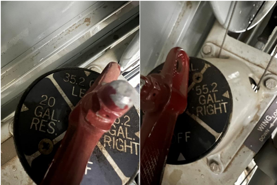
Detail view of the front seat fuel selector handle and placard
