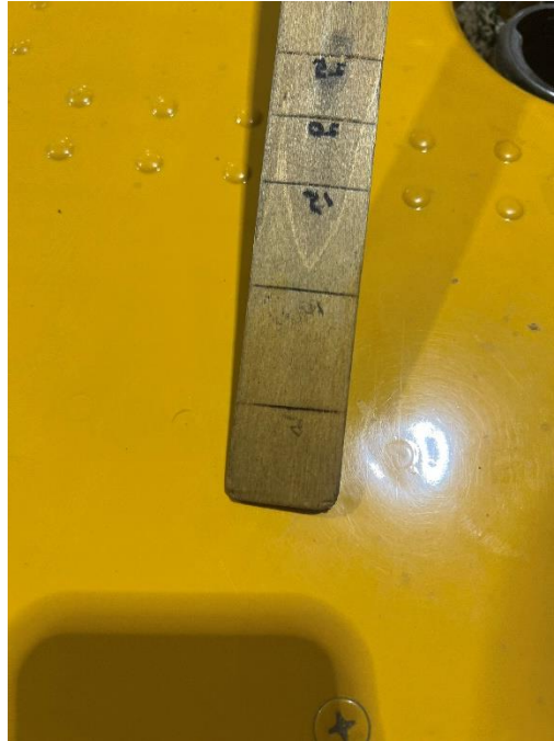
Detail view of the calibrated dip stick reading of the left tank upon arrival in lone
