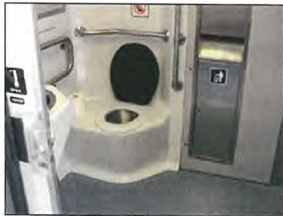
Figure 13 Toilet inside a Caltrain gallery car, Caltrain photo
