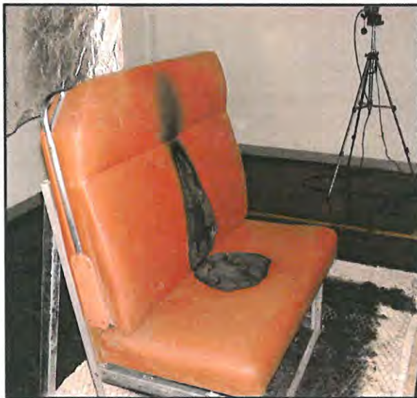
Figure 21: VRE seat after fire test. WH photo
