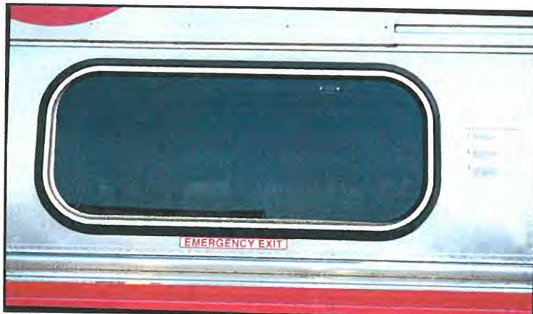
Figure 10: Gallery car emergency window, FCA photo
