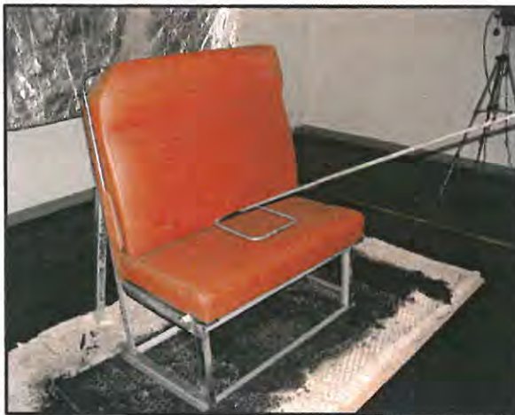
Figure 20: VRE seat before fire test, WH photo
