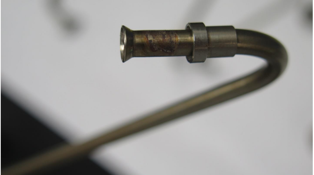
Example of corrosion found on engine equipment (start injector pipe)
