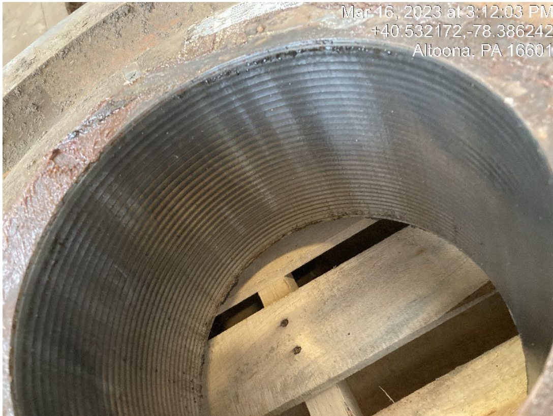
Figure 2. Wheel bore of wheel 05508 from car NS 162581 after being pressed from its axle.
