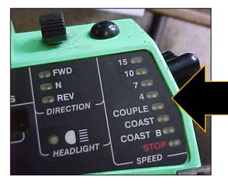
Movement will be initiated by selecting Couple Remember to keep the RCL moving at a slow speed (2 mph or less) until the entire cut is moving. The 4 mph setting should not be selected until slack has adjusted and entire train is moving
