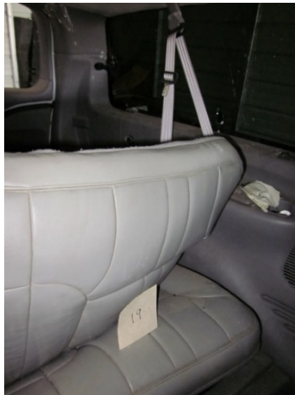
Figure 28: Limousine OEM seat position 19 D-ring location between G and H pillar.
