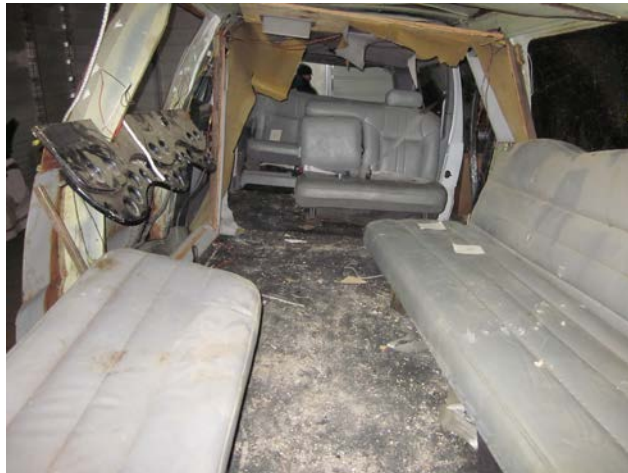
Figure 24: View of limousine interior looking aft, with lateral seat cushions put back in approximate position during post crash inspection
