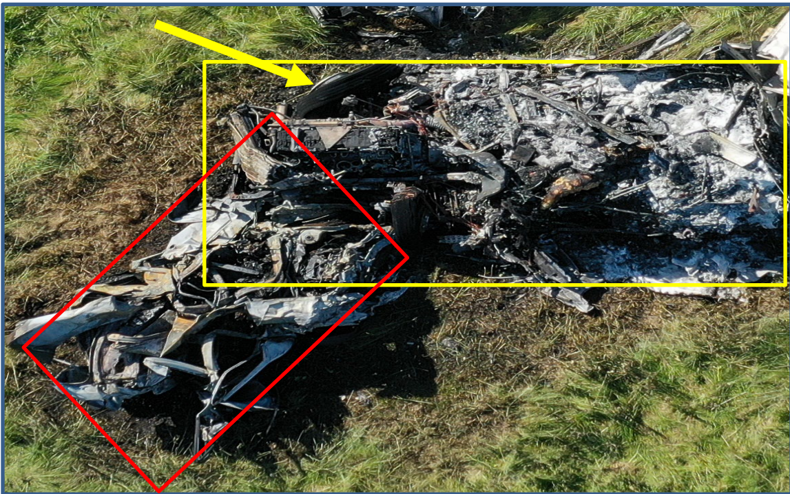
Figure 1. Overhead view of the Freightliner truck tractor, outlined in the yellow box, with the left-front portion in contact with the Chevrolet Malibu, outlined in red box. [source: WSP]
