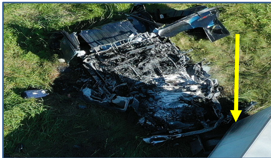
Figure 5. Overhead view of the Ford pickup at its final rest position, with the left-front corner in contact with the left-rear drive axle of the Freightliner. [source: WSP]
