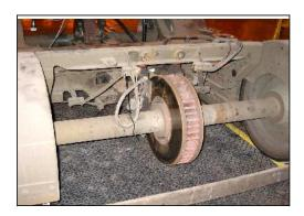
C. <u>Track</u> – An electro magnetic brake located between the wheels of each truck that operates through direct contact with the running rail. Applied as the second step in an emergency braking process.
