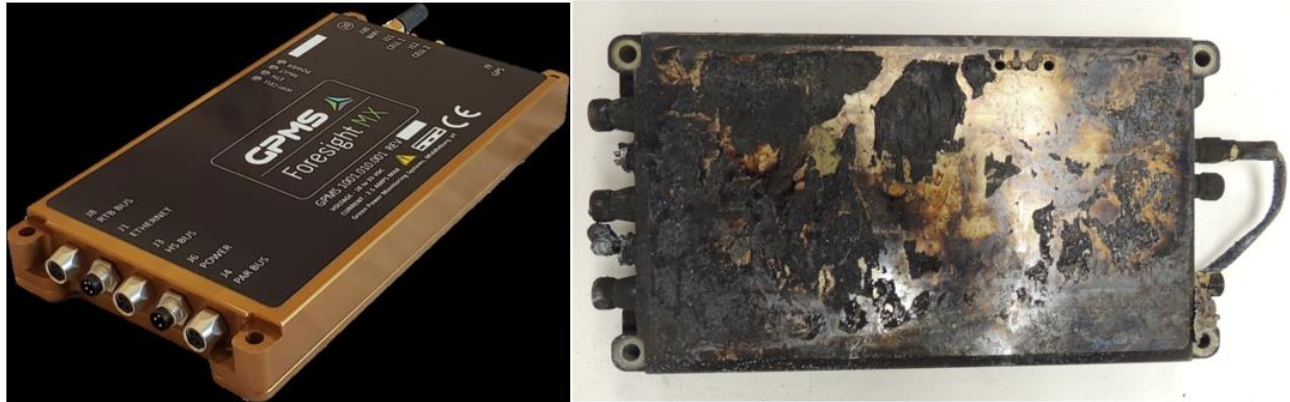
Figure 1: Undamaged OBCU vs. OBCU as received.
