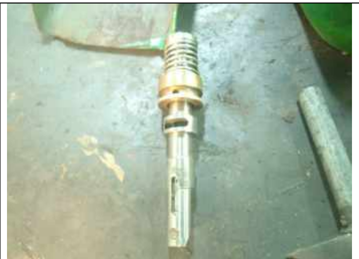
Dismantled No.:1 piston valve condition (cleaned and normal)
