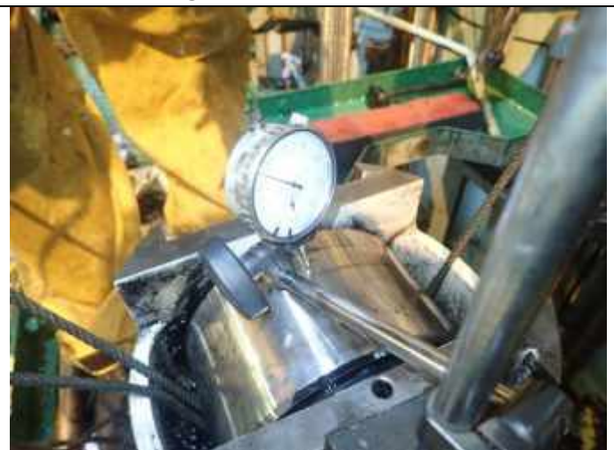
Measured clearance of roller guide
