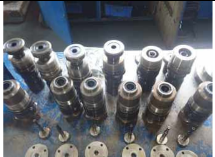
Maintained suction and puncture valves
