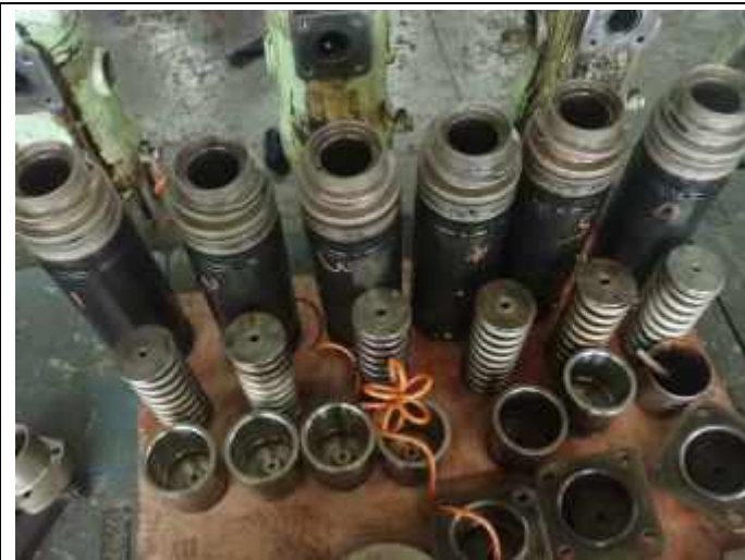
Dismantled plunger and barrels
