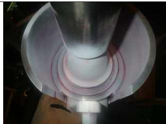
Penetration test of roller guide
