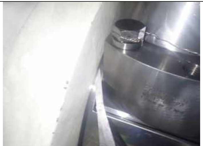
Crosshead bearing clearance measured
