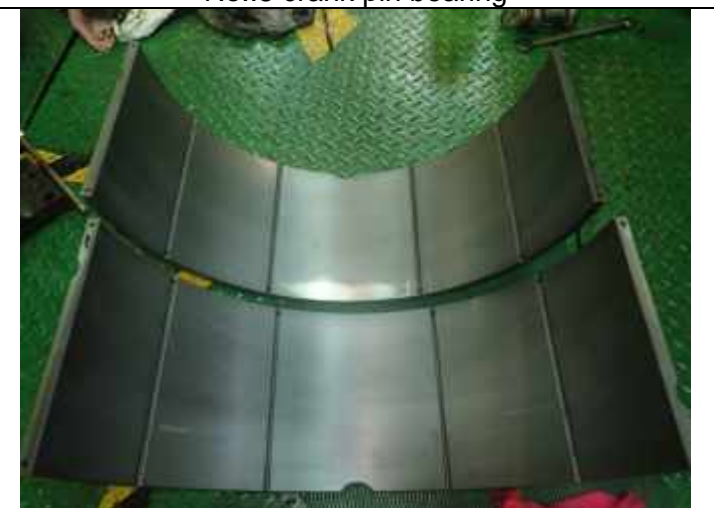
No.:2 crosshead bearing
