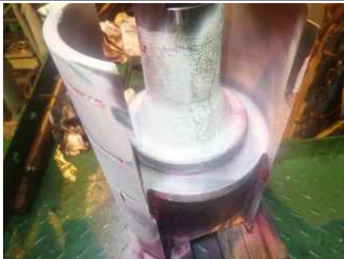
Penetration test of roller guide
