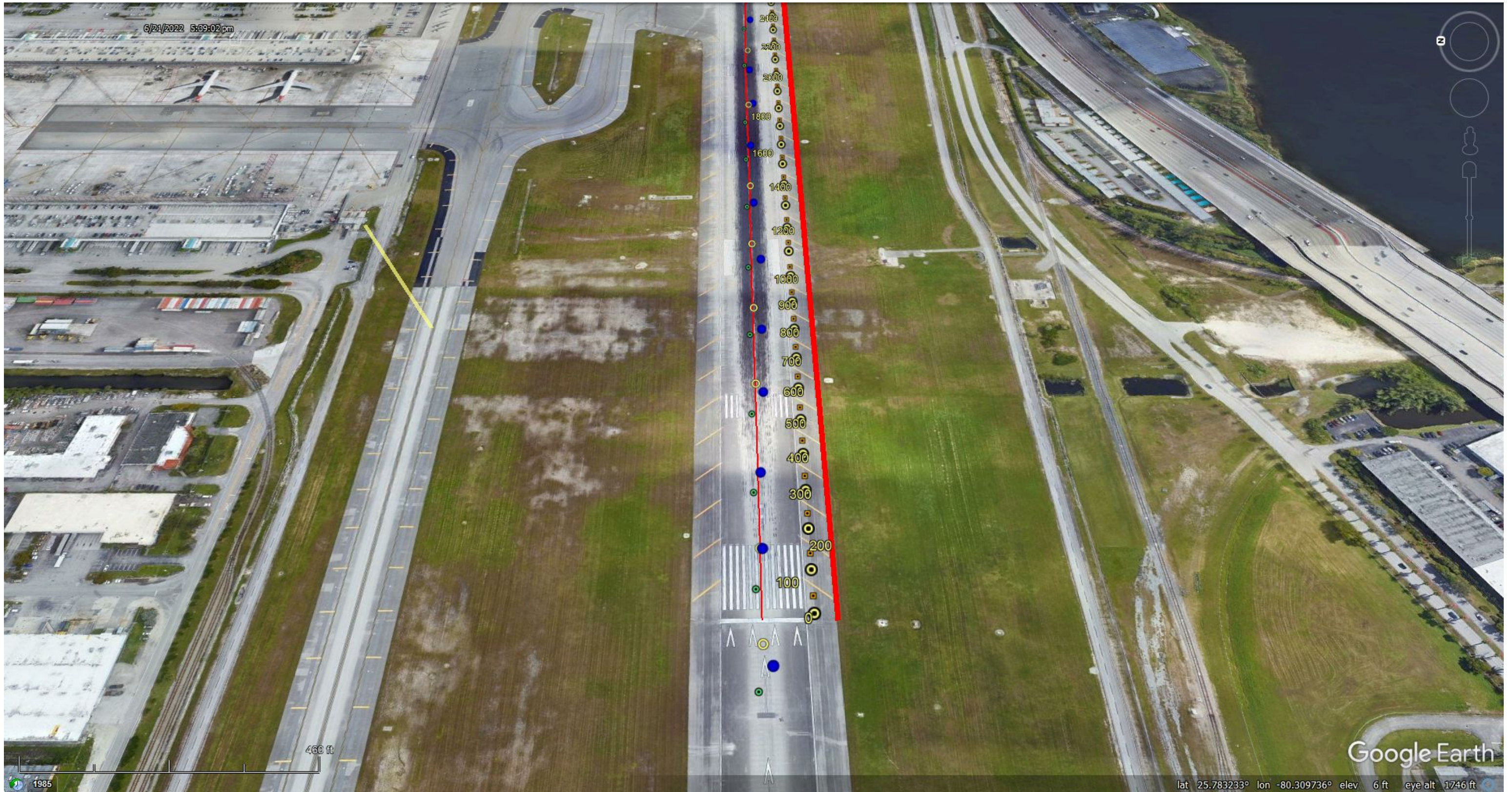
Figure 10: Example of HI1064 accident flight path reconstruction looking toward the runway 9 displaced threshold, showing 0 to 2,400 feet along the runway. Ground track reconstruction is based on ADS-B, FDR, paraphrased CVR, video, and runway witness mark evidence. Aircraft direction of travel is toward the top of the page. FAA ADS-B data recorded for HI1064 are identified by blue symbols. Green symbols depict NTSB flightpath calculated by integrating FDR accelerometer data. Distance beyond the runway 9 displaced threshold is annotated in feet. This image is a duplicate of Attachment 14, Figure A14.3.
