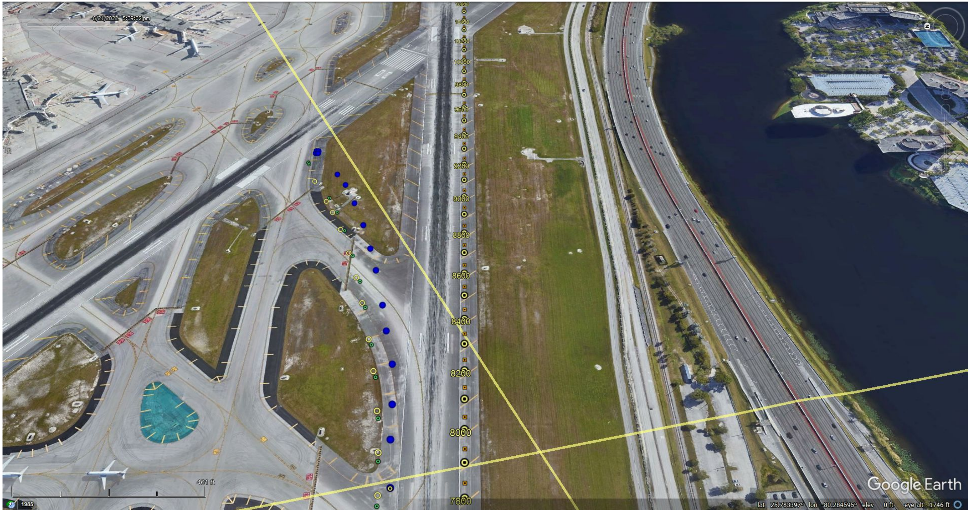
Figure A14.11: HI1064 accident flight reconstruction 8,000 to 9,000 feet beyond the runway 9 displaced threshold. Ground track reconstruction is based on FAA ADS-B, paraphrased CVR, FDR, video, and runway witness mark evidence. Aircraft direction of travel is toward the top of the page. FAA ADS-B data recorded for HI1064 are identified by blue symbols. Green symbols depict NTSB flightpath calculated by integrating FDR accelerometer data. Distance beyond the runway 9 displaced threshold is annotated in feet.
