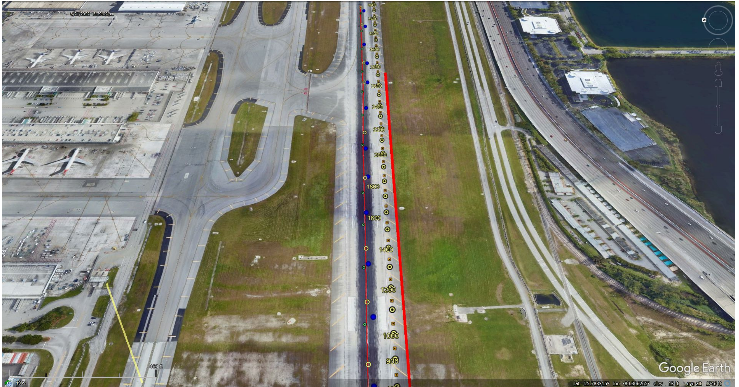
Figure A14.4: HI1064 accident flight reconstruction 1,000 to 2,000 feet beyond the runway 9 displaced threshold. Ground track reconstruction is based on FAA ADS-B, paraphrased CVR, FDR, video, and runway witness mark evidence. Aircraft direction of travel is toward the top of the page. FAA ADS-B data recorded for HI1064 are identified by blue symbols. Green symbols depict NTSB flightpath calculated by integrating FDR accelerometer data. Distance beyond the runway 9 displaced threshold is annotated in feet.
