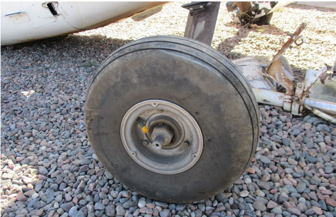
Figure 4: View of left main landing gear (photo courtesy of the FAA)
