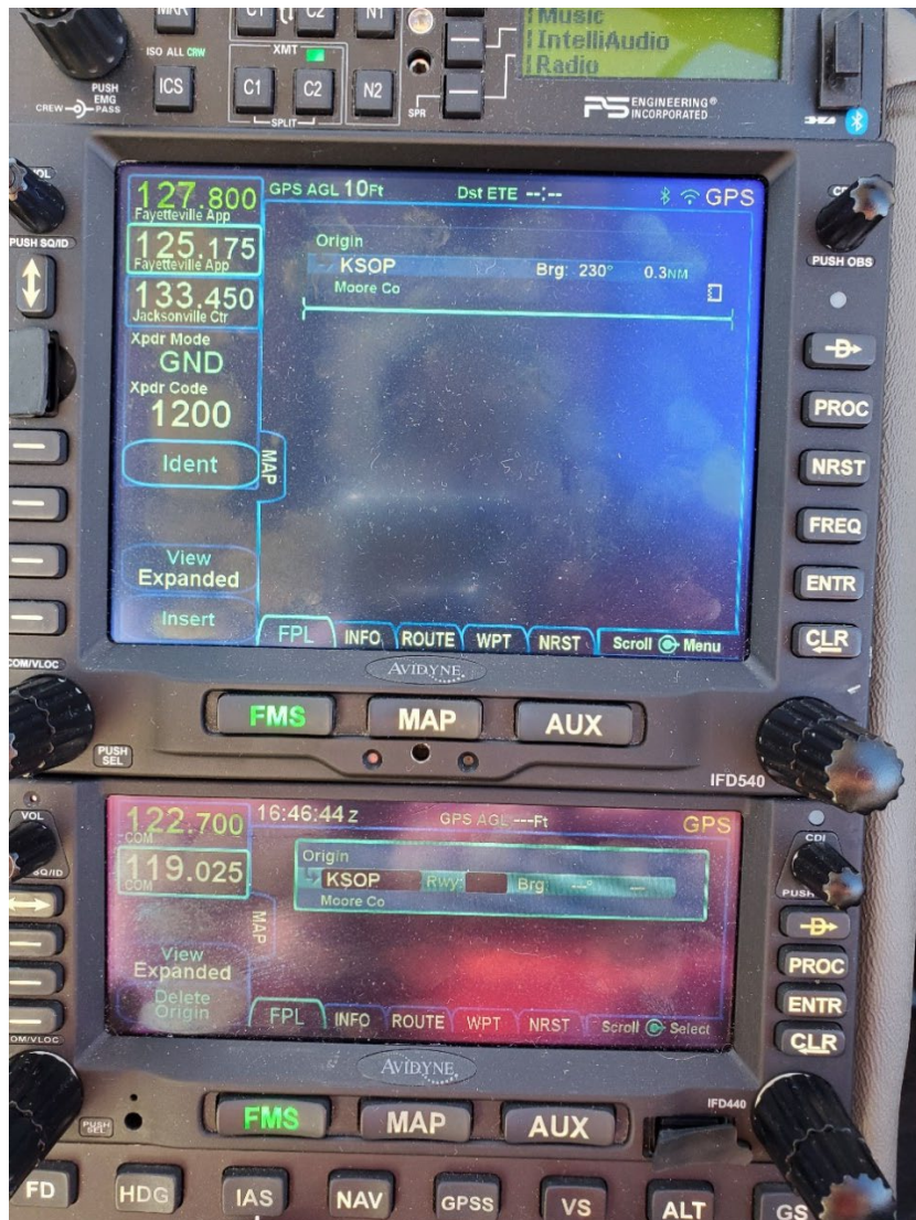
Figure 1: Photograph Taken by AMF Personnel 8 . View Depicting The Comm #2 Radio Active Frequency set to 122.700 MHz and the Transmitter Set to the #2 Comm Radio. The photograph was taken 2/10/2022 at 1146 local.
