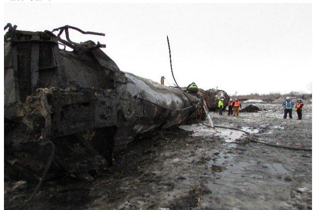
1(d) A-end head looking toward B-end along bottom. Impact damage on right side.
