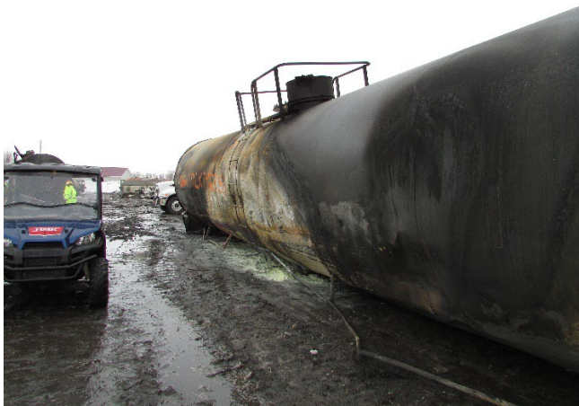
4 (c) left side from A-end showing thermal damage.
