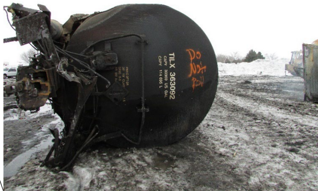
1(a) B-end head, damage to head at 7 to 8 o'clock position.
