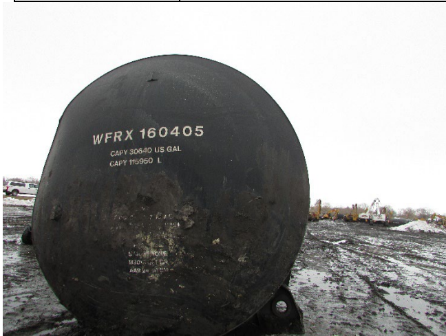
5(a) A-end showing damage to head at 9 to 10 o'clock.
