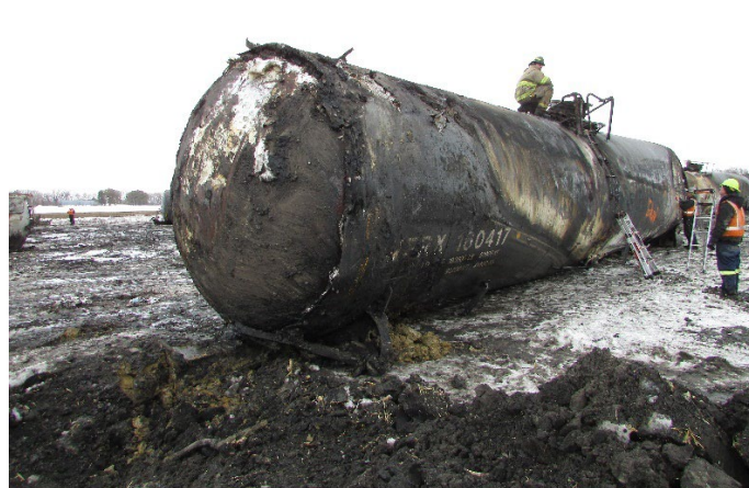
3(c) A-end looking along right side. A-end head shield missing
