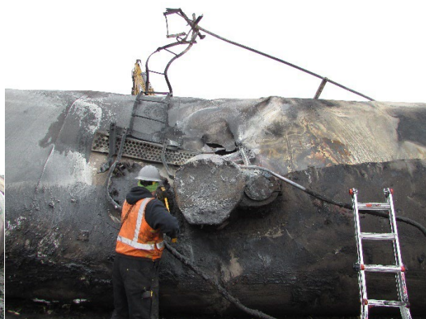
2(b) Shell puncture damage near protective housing
