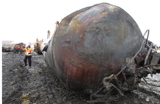
2(c) B-end showing missing head shield and damage at 1 o'clock position
