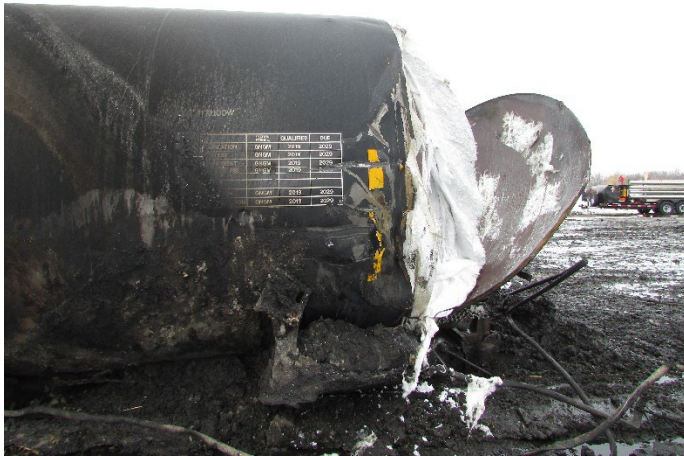
5(c) B-end, showing certification dates and damage to head shield.
