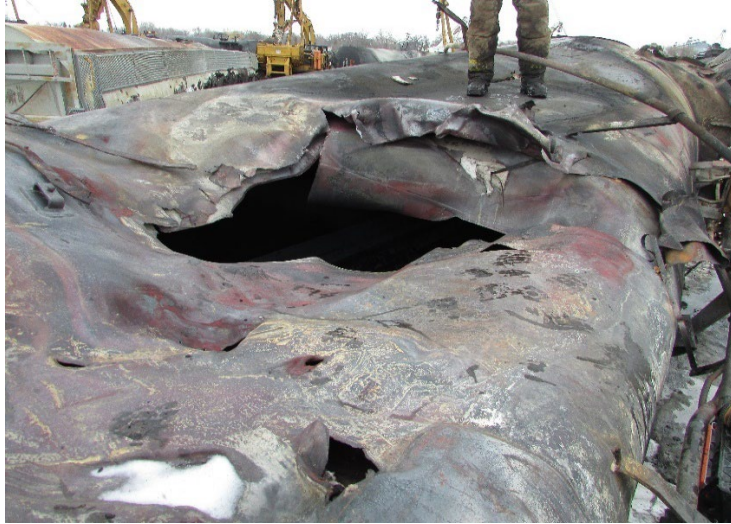
1(e) Right side of car. Triangle shaped puncture.
