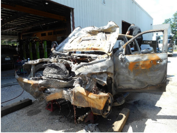
Figure 1. Frontal view of deformation to Ram 2500. Figure 2. Right side view of deformation to Ram 2500.
