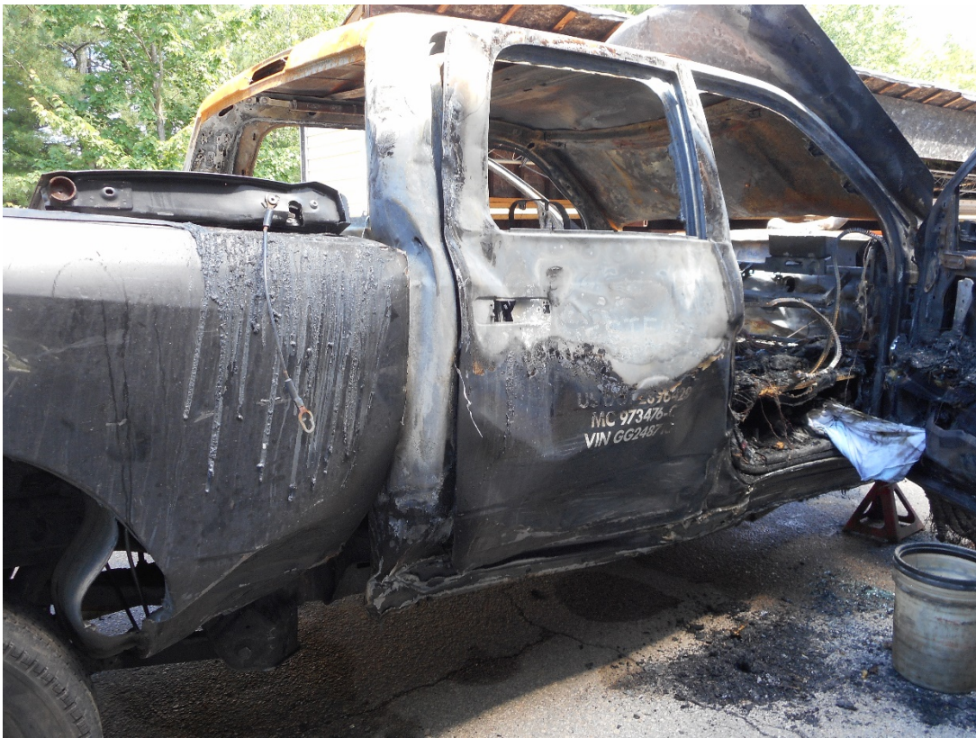
Photo 3 – Right side view of damage and deformation to 2016 Ram 2500.
