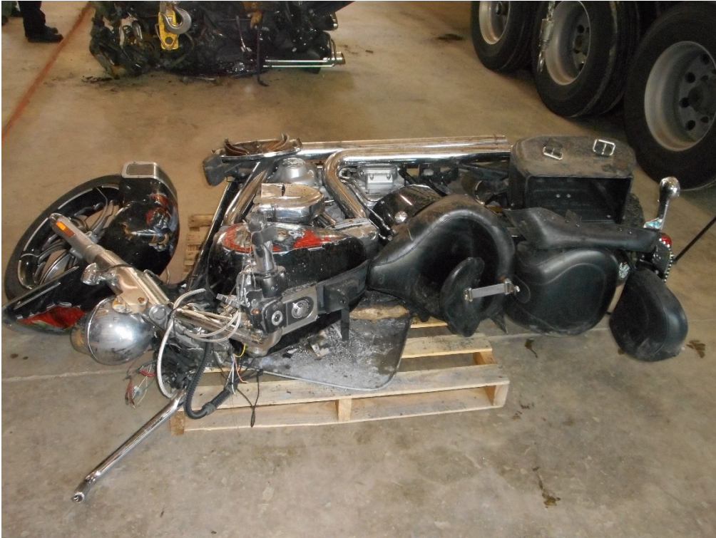
Photo 7 – View of deformation to 2006 Harley Davidson Heritage Softail FLSTI.
