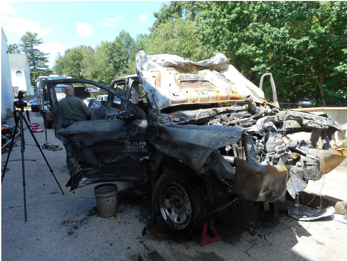
Photo 2 – Front left angle view of deformation and fire damage to front and right side of 2016 Ram 2500.
