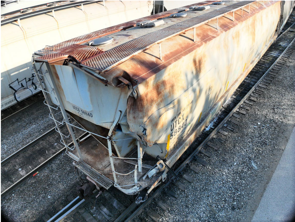
Figure 4 - The west railcar UTCX 58840 that struck locomotive NS 1648
