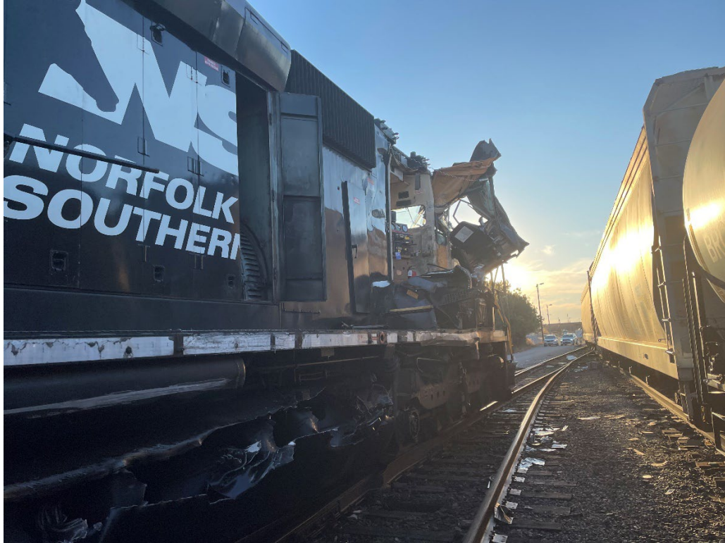
Figure 3 - Locomotive NS 1648 that was struck by the rail cars that rolled from the east end of track CT7.
