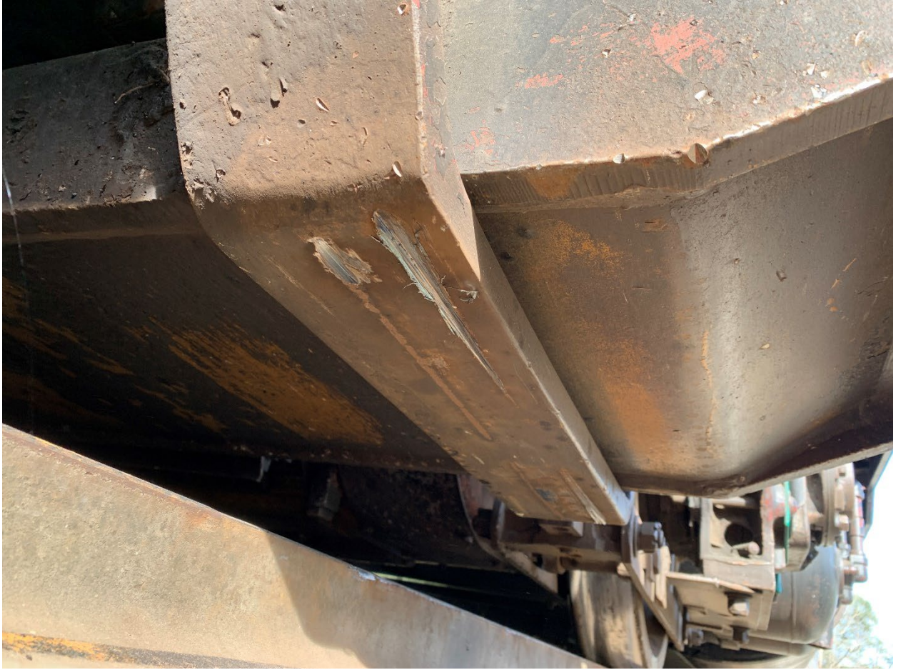
Figure 12. REX 06 rear right hanger with rail burn witness marks.
