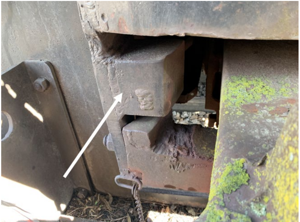
Figure 18. RMEX 08 non-alignment control coupler alignment block
