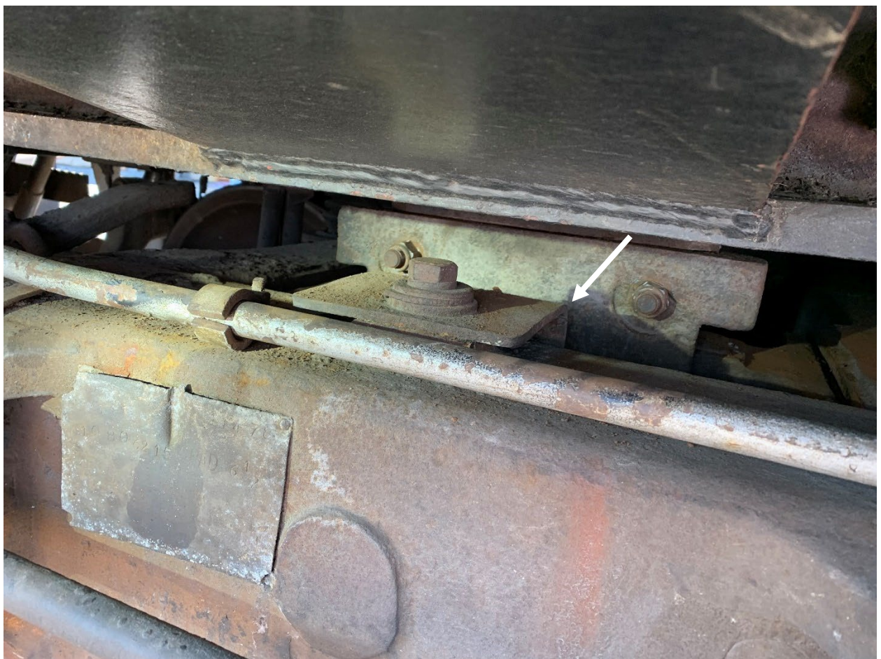
Figure 40. RMEX 08 Bolster stop block in the normal configuration.
