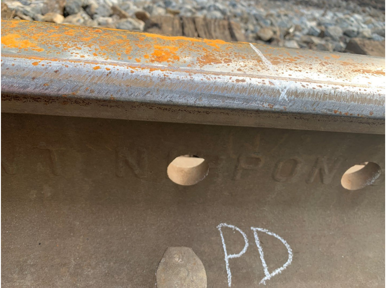
Figure 10. Wheel and wheel tread departure mark near MP 721.05.
