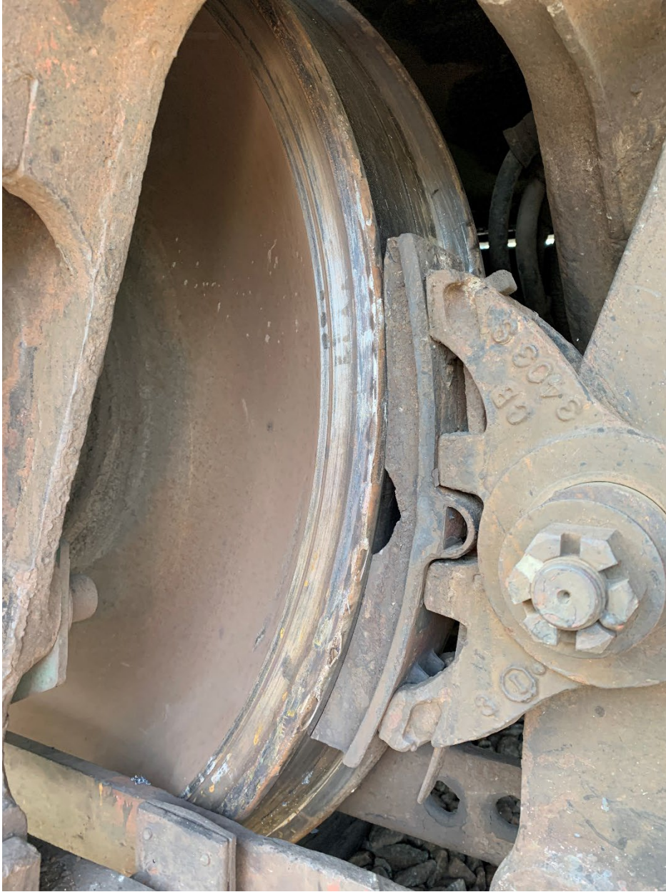
Figure 11. RMEX 06 R3 Wheel with rail burn witness marks.
