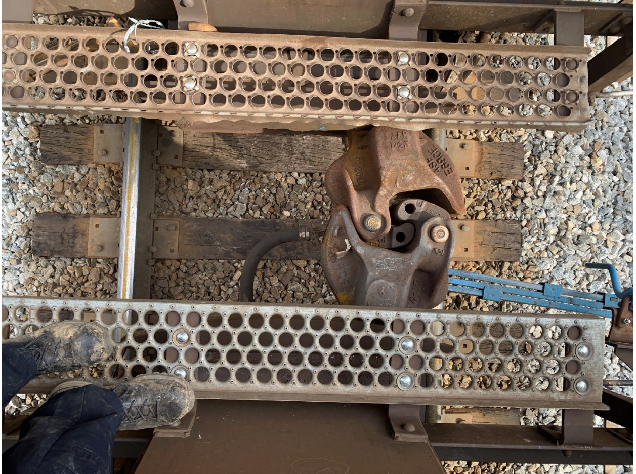
Figure 13. Cars at rest (post-derailment) near MP 721.05 with jackknifed couplers
