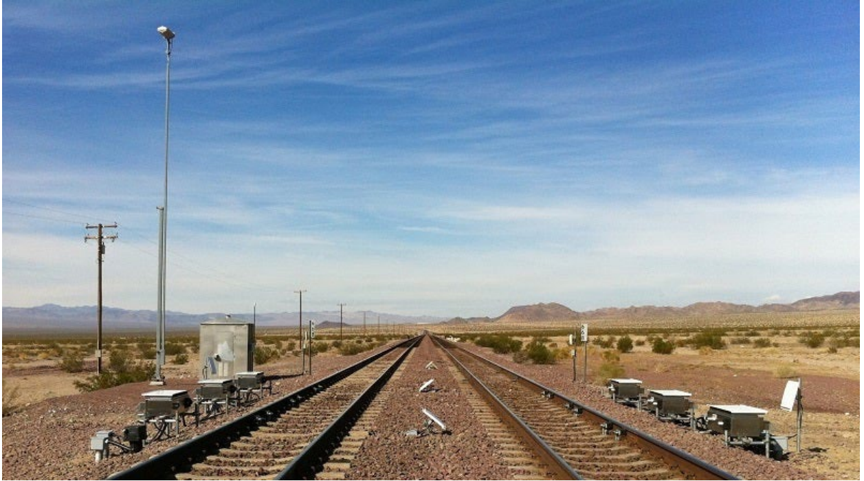
Figure 36. A field installation of TBOGI (WDI stock image)
