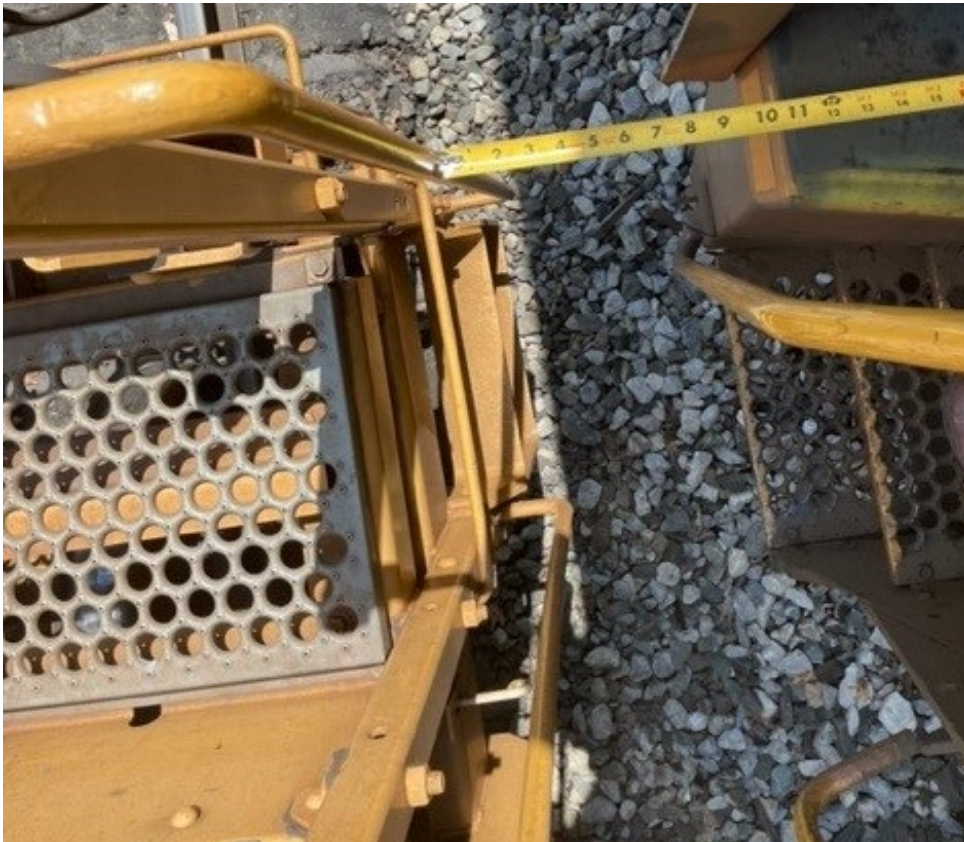
Figure 3: Clearance between the intermodal car and standing locomotives. (Photo: CSX.)
