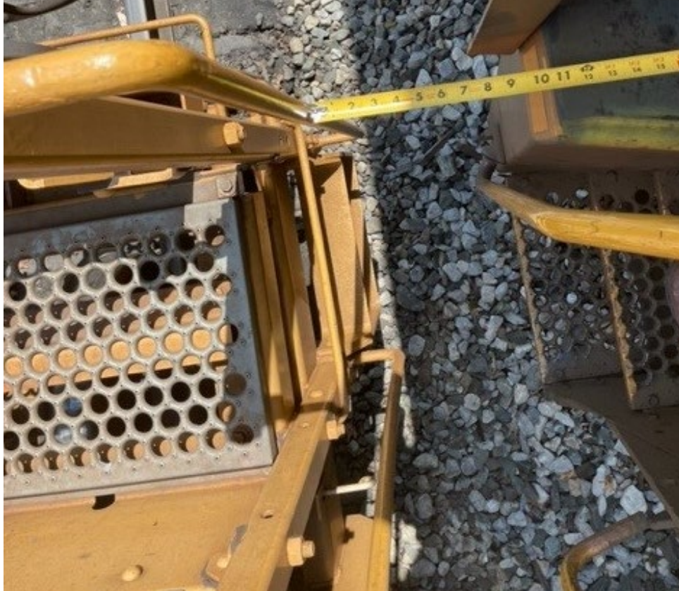
Figure 2. Clearance between the intermodal car and standing locomotives. (Photo: CSX.)
