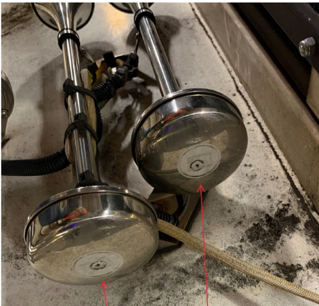
Figure 4 Spiker GS 15022 Rear facing trumpets with screws accessible (FRA Photograph and annotations)
