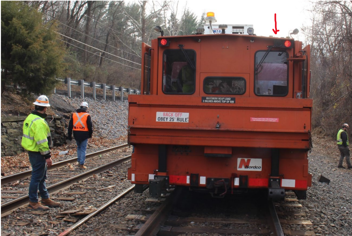
Figure 8. Spiker GS 16043 with an arrow pointing to the rear facing change-of-direction alarm speaker. The disconnected speaker plug can be seen below the speaker. (NTSB Photograph and annotations)
