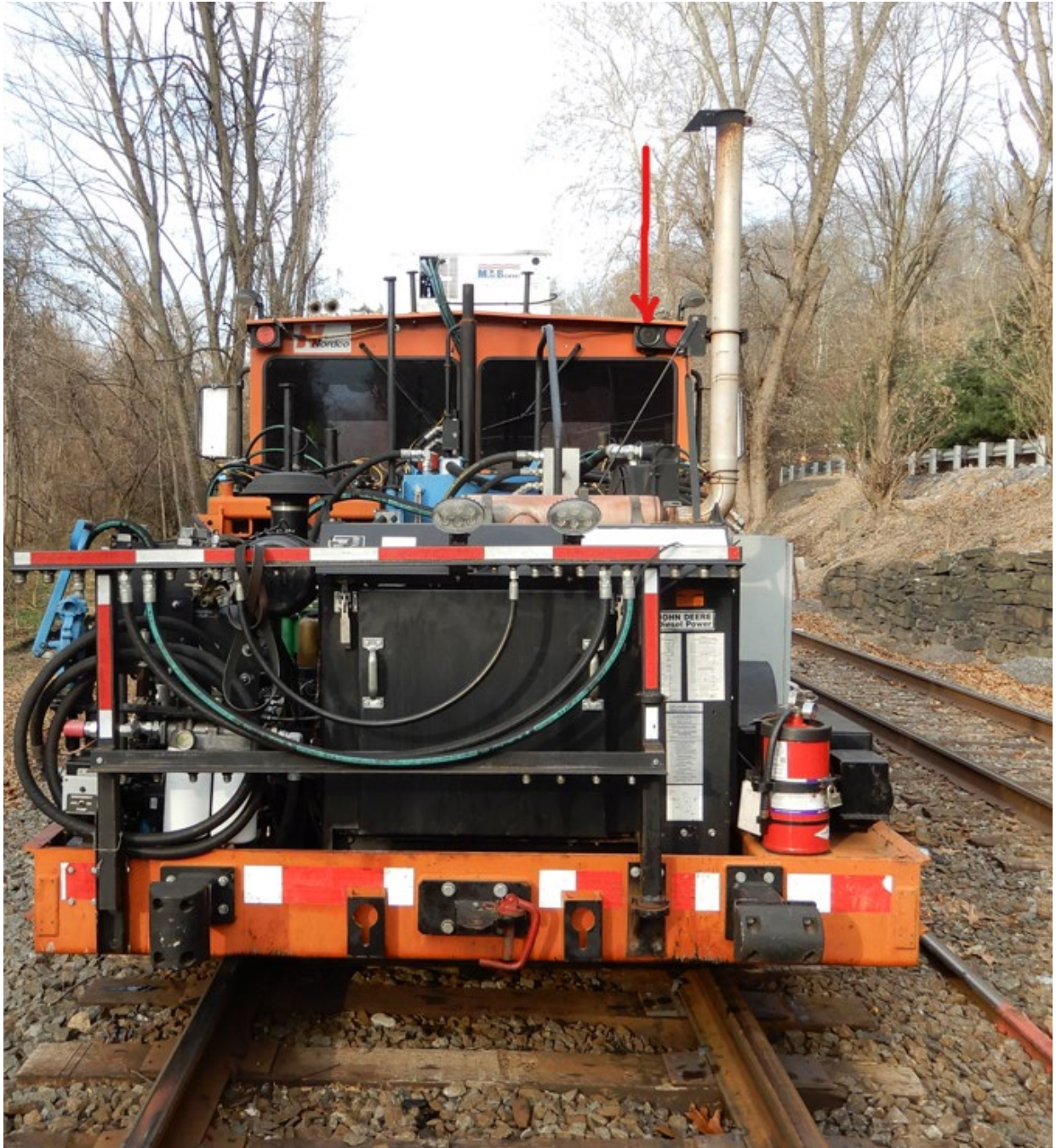
Figure 7. Spiker with arrow pointing to front facing change-of-direction alarm speaker (NTSB Photograph and annotations)
