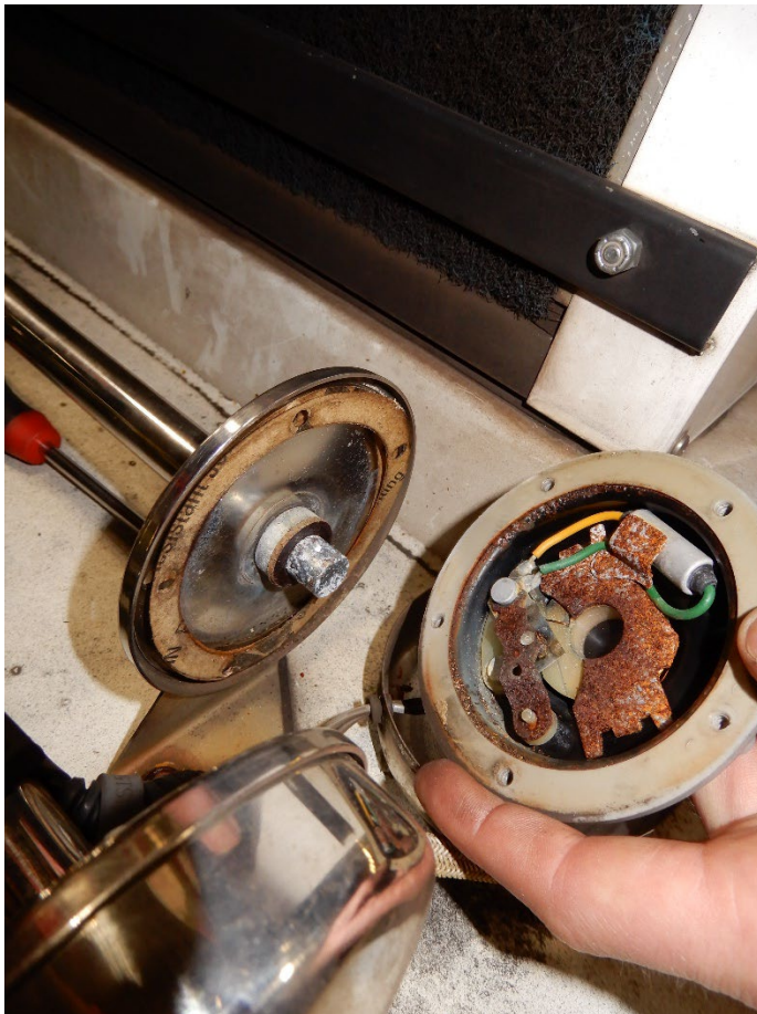
Figure 5. The interior condition of a horn trumpet.
