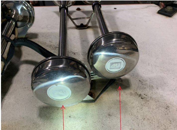
Figure 3 Spiker GS 15022 Front facing trumpets with screw covered (FRA Photograph and annotations)
