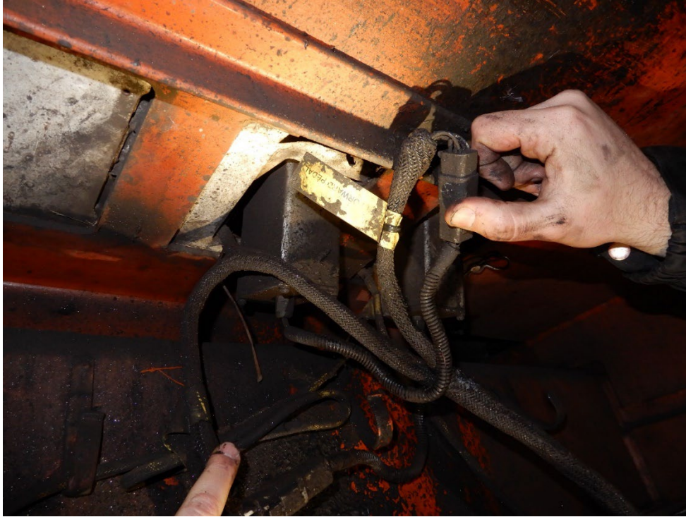
Figure 9. Under the cab, looking at the plugs for the left side pedals. They are reversed (as found) in this photo.
