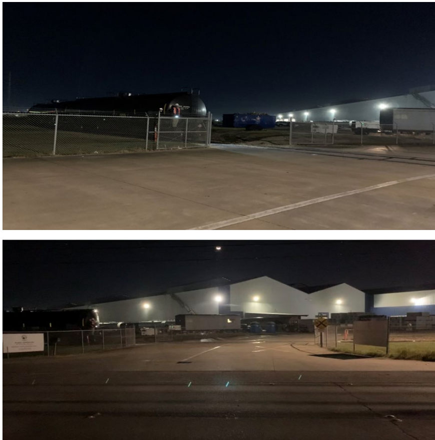
Figure 3: Photos taken during the site distance test conducted at 4:00 a.m. local time. Note: The approach photographs and video do not represent a complete view from the perspective of the driver since the tank cars remains still.
