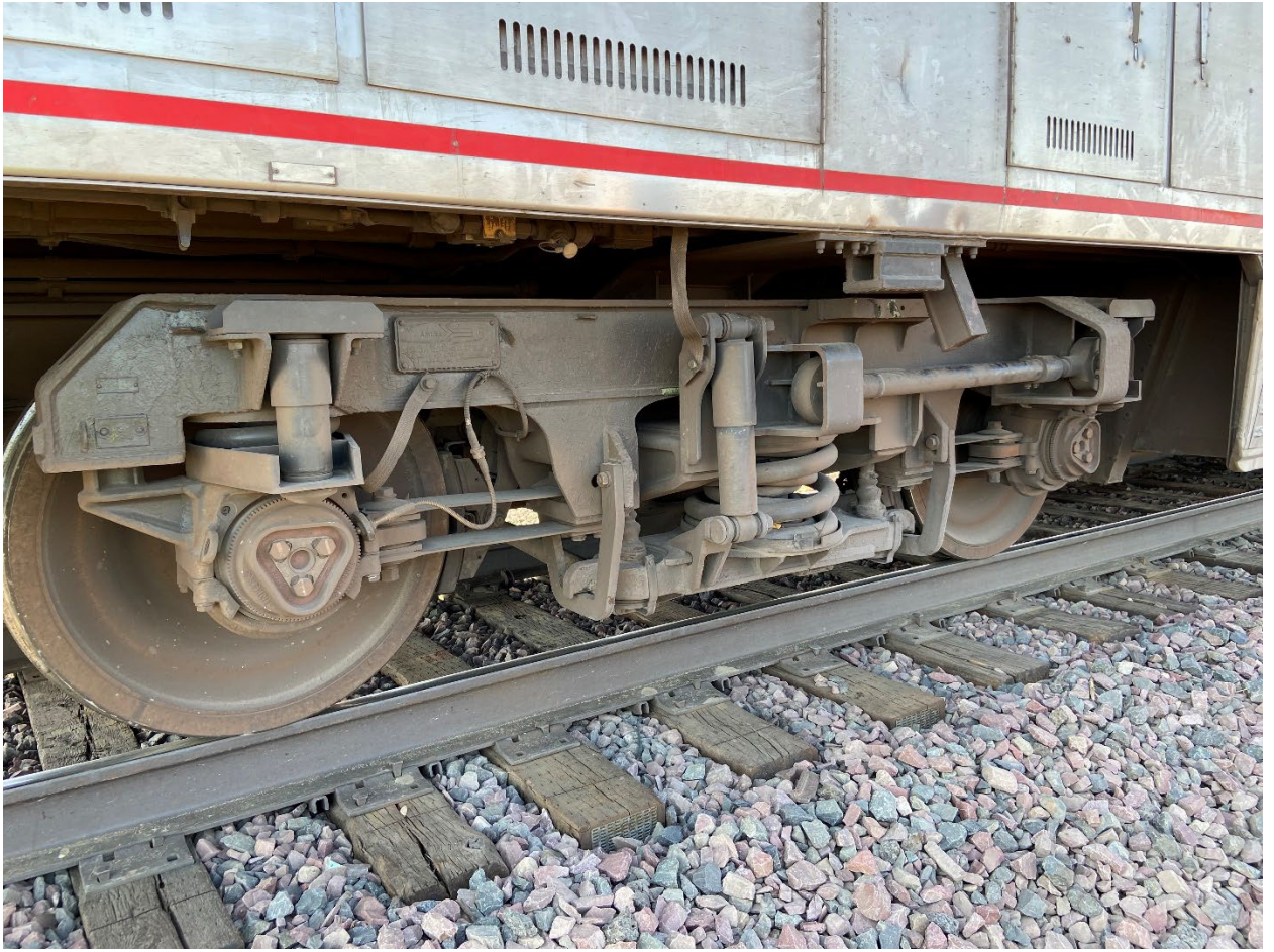
Figure 2. Post-accident image of a Superliner I truck assembly.
