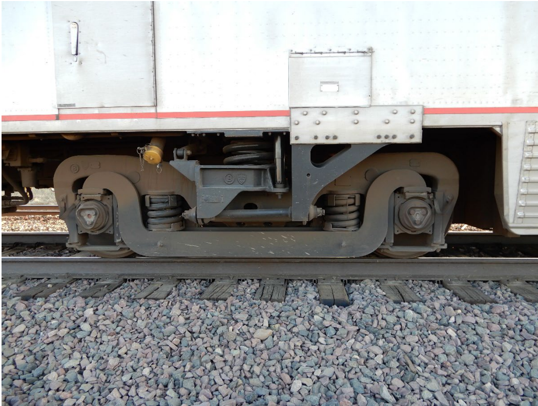
Figure 3. Post-accident image of a Superliner II truck assembly.
