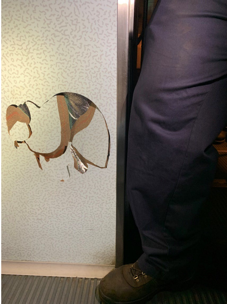
Figure 3. Trolley 3862 inside facia with hole.
