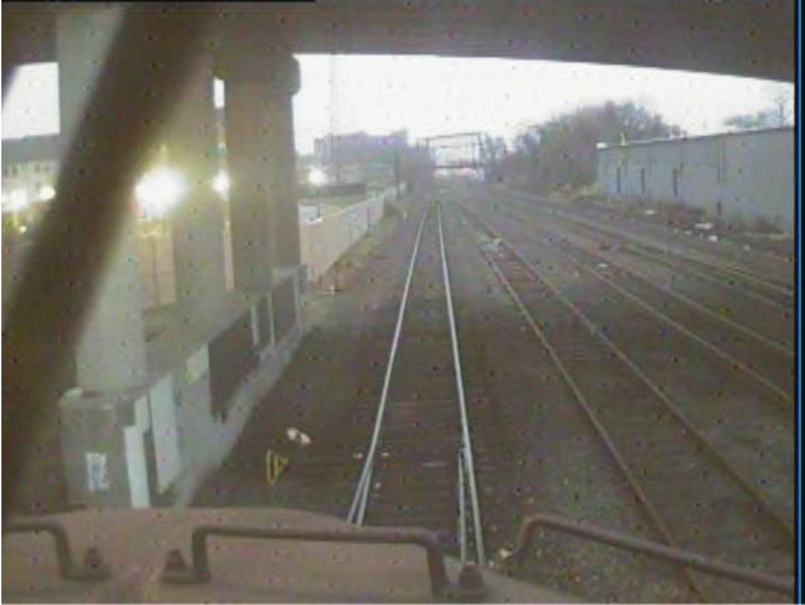
Figure 2. The locomotive reversing past a switch in the vicinity of the President's Street Bridge. The switch is lined for the Bank track, the Perryville track is seen to the right of the locomotive.
