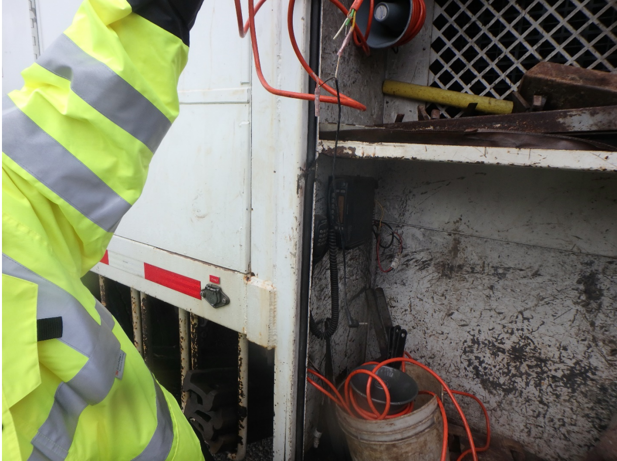
Figure 6. Photo showing two speakers that were located inside the truck cabinet that contained the external radio.
