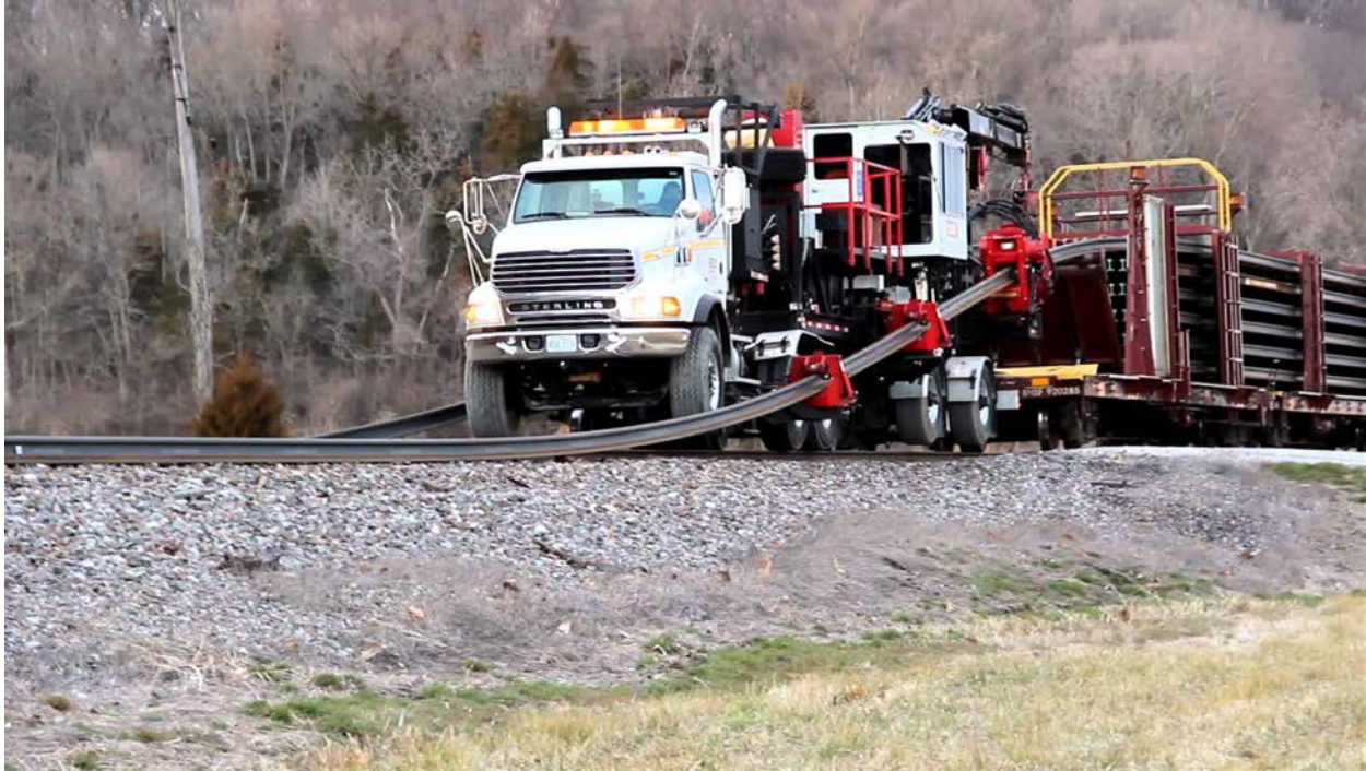
Figure 5 Photo courtesy of BNSF, this is a photo of the work train a day prior to the accident. The Rail Unloading Machine (RUM) truck is attached to the rear of the work train.
