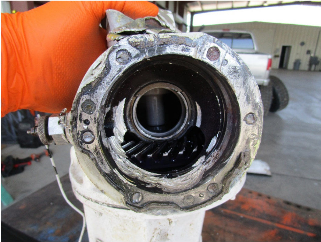
Figure 6: Attachment Bolt Fragments
