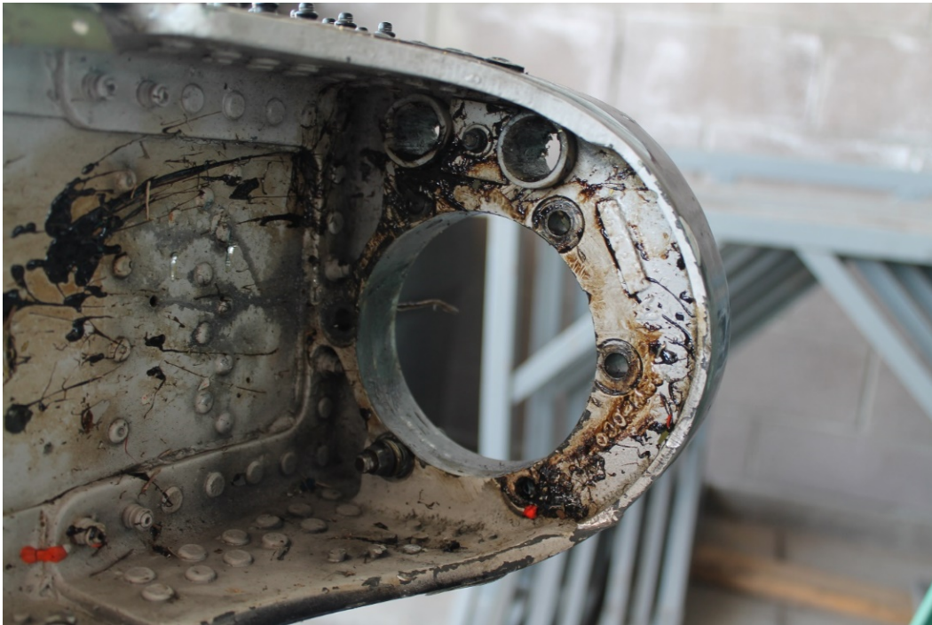
Figure 1: Underside of the top of the Vertical Stabilizer
